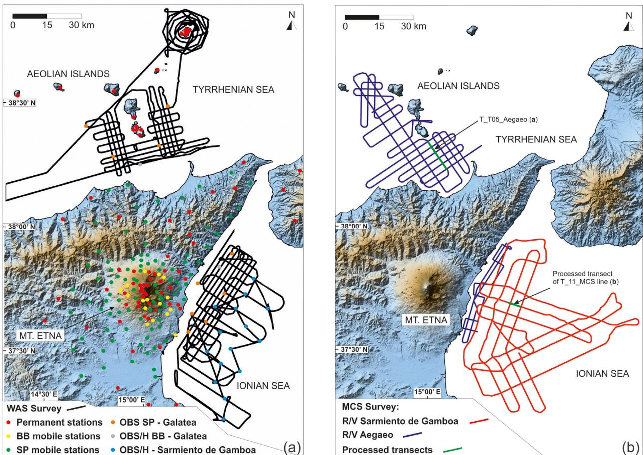
**Figure 2.** Lines of shots: (a) wide angle seismic (WAS) for the "Sarmiento de Gamboa" campaign. Colored dots indicate the position of the seismic stations (see legend in the figure for details); (b) multi-channel seismic (MCS) lines for the "Sarmiento de Gamboa" and "Aegaeo" campaign. (Figure 2 continues on next page.)
