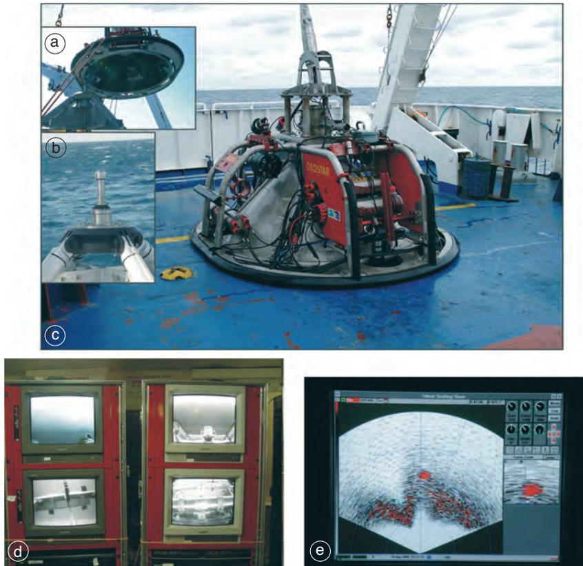
**Fig. 3a-e.** MODUS, the GEOSTAR deployment/recovery vehicle: a) docking cone and b) pin; c) MODUS on the deck of R/V Urania; d) MODUS on-board console; e) Bottom Station signature displayed on the sonar monitor.
