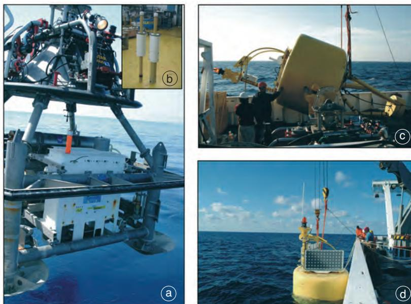
**Fig. 5a-d.** a) MESSAGERS installed on the Bottom Station (height 1.3 m); b) MESSAGERS Storage and Expendable-type in Brest IFREMER Laboratory; c) surface buoy (weight: 35 kN; volume: 5 m<sup>3</sup>) GEOSTAR-2 version on board R/V Urania; d) surface buoy ORION-GEOSTAR-3 version just deployed.
