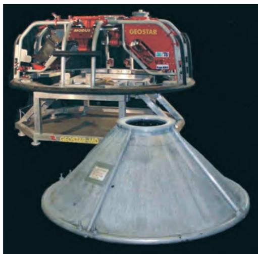
**Fig. 2.** MODUS with SCISKID (background) and docking cone (foreground).
