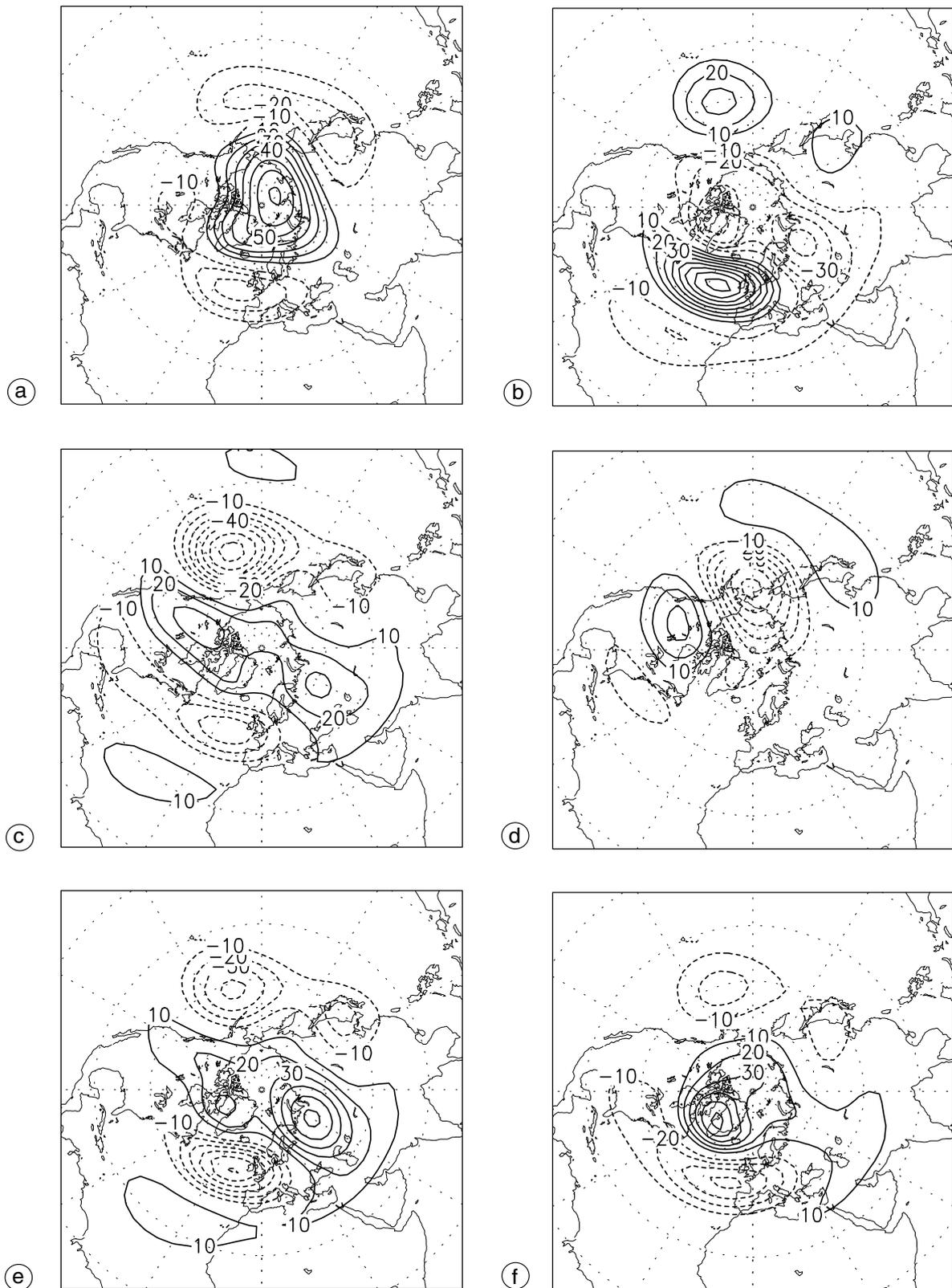
**Fig. 6a-f.** Common spatial structures obtained through the super-ensemble rotated EOF analysis for DJF-mean 500-hPa geopotential height in the Northern Hemisphere. The explained variance is respectively 16.2% (a); 13.4% (b); 12.3% (c); 10.7% (d); 9.5% (e), and 7.5% (f). Total variance is  $302 \text{ m}^2 \text{ s}^{-2}$ . Units are in meters.
