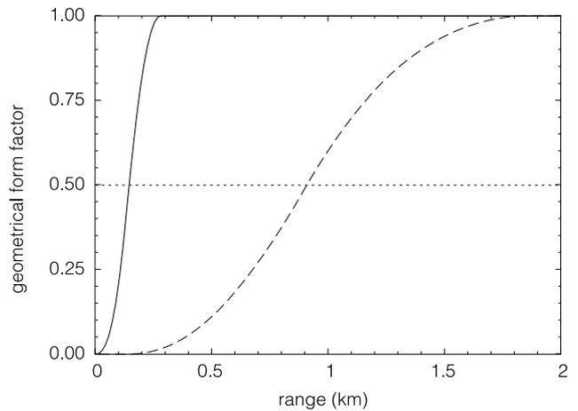
**Fig. 1.** Geometrical form factors for the two receivers: small telescope (solid line); large telescope (dashed line).
