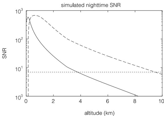
**Fig. 4.** Simulated SNR in nighttime (no background) for 2 min integration time with the small telescope (solid line), and for 30 min integration time with the large telescope (dashed line). The thin dotted line denotes the SNR = 7 level.
