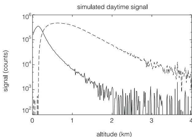
**Fig. 2.** Simulated water vapour Raman lidar signal for 2 min integration time with the small telescope (solid line), and for 30 min integration time with the large telescope (dashed line). A random statistical error with Poisson distribution was added to simulate photon count statistics.
