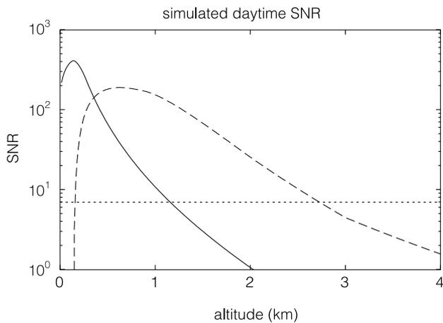
**Fig. 3.** Simulated SNR in daytime for 2 min integration time with the small telescope (solid line), and for 30 min integration time with the large telescope (dashed line). The thin dotted line denotes the SNR = 7 level.
