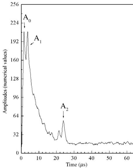
**Fig. 2.** Example of the radar traces acquired during 1999 at Talos Dome.  $X$  axis represents the full time range of  $64 \mu\text{s}$  while  $Y$  axis indicates the 8-bit A/D dynamics.  $A_0$  is the amplitude of the transmitted peak,  $A_1$  is the reflection from the ice surface and  $A_2$  is the bedrock echo.
