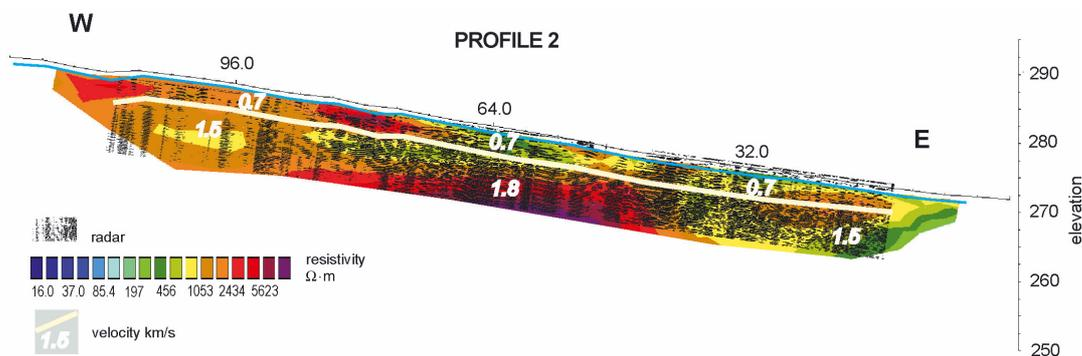
Fig. 9. Overlapping of three seismic, electric and radar methods.
