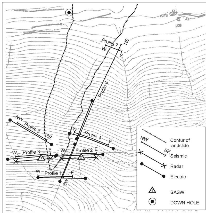
Fig. 3. Planimetry showing the positions of different indirect surveys.
