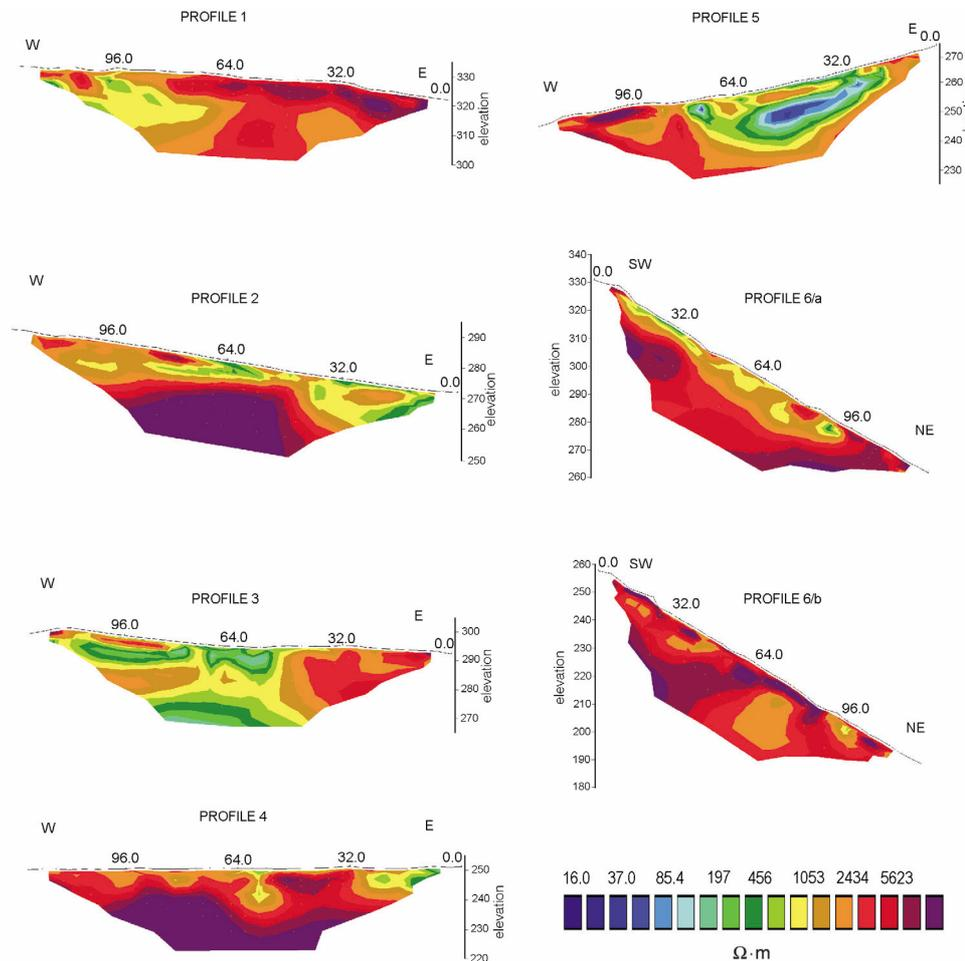
Fig. 5. Electric imaging profile.
