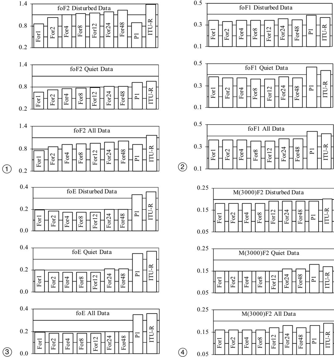
**Fig. 1.** Bar chart created for RMS errors for  $f_oF_2$  characteristic, for disturbed data (upper panel), quiet data (middle panel), and for all data together (lower panel). Autocovariance forecasting method: For1, 1 h ahead For2, 2 h ahead, etc. Persistence: P1.
