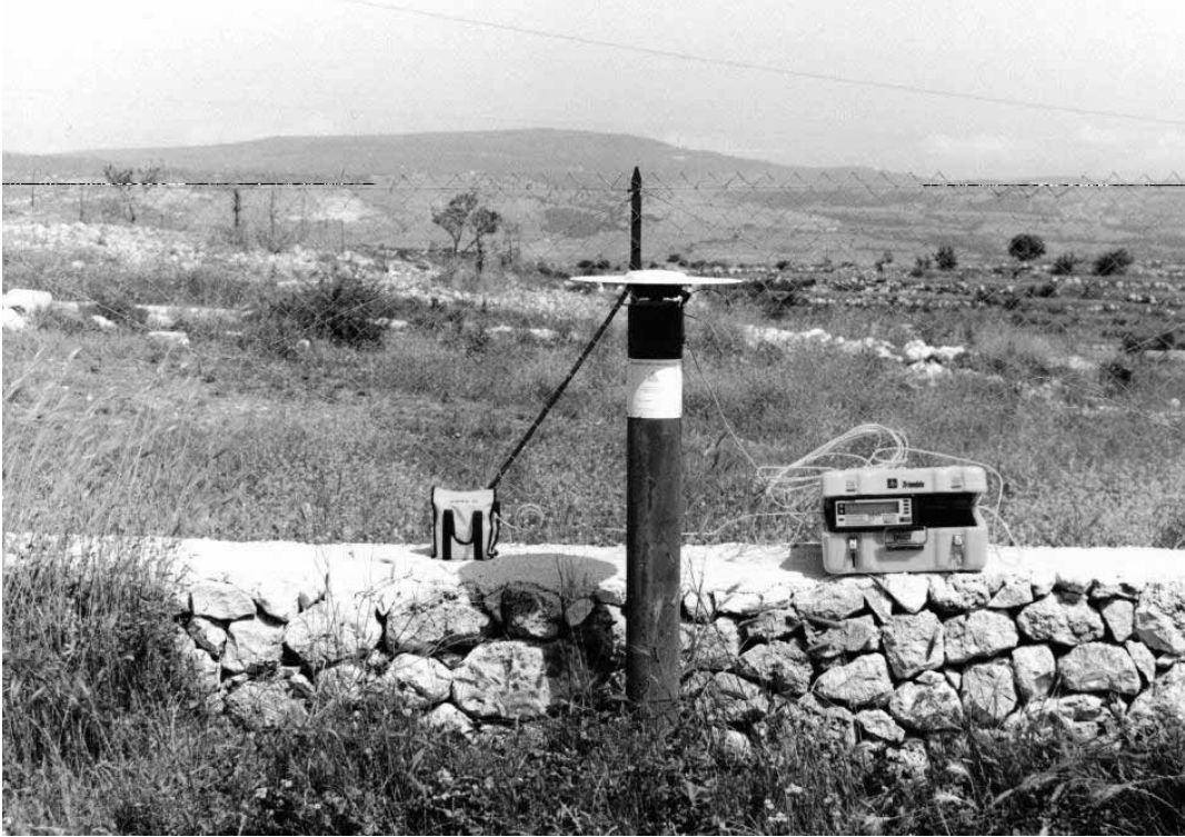
Fig. 3. Typical station of the Hyblean GPS network (IP21 pillar).
