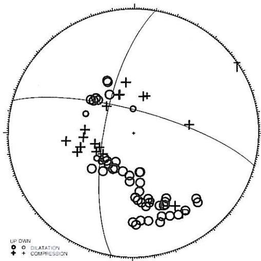
**Fig. 2.** Example of polarity distribution on a lower hemisphere projection for a small magnitude deep event of the Tyrrhenian zone.
