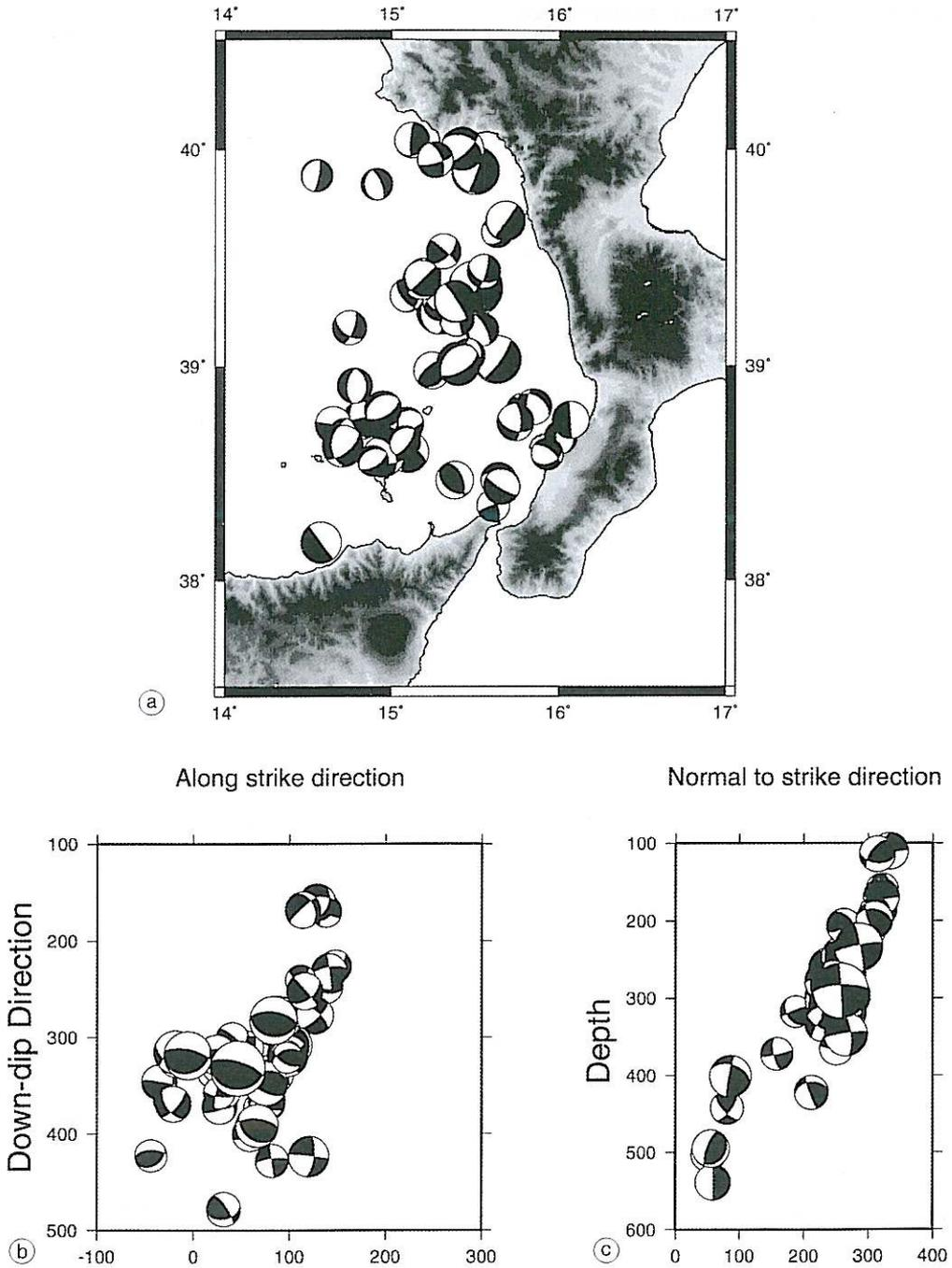
Fig. 3a-c. Available fault plane solutions for the Tyrrhenian deep earthquakes. a) Map view; b) projected on a 70° dipping plane in the along strike direction of the slab; c) perpendicular to the slab direction.
