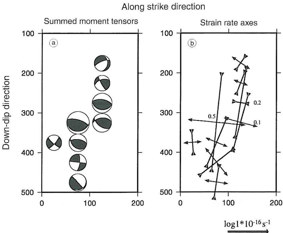
**Fig. 4a,b.** a) Summed moment tensor in each zone in which the slab has been divided. Fault plane solutions are scaled with magnitude; b) average seismic strain rate principal axes, inward arrows are compressional strain and outward arrows are extensional strain. Length is on log scale. Down-dip shortening (mm/yr) is shown in cubic regions when larger than 0.1 mm/yr.
