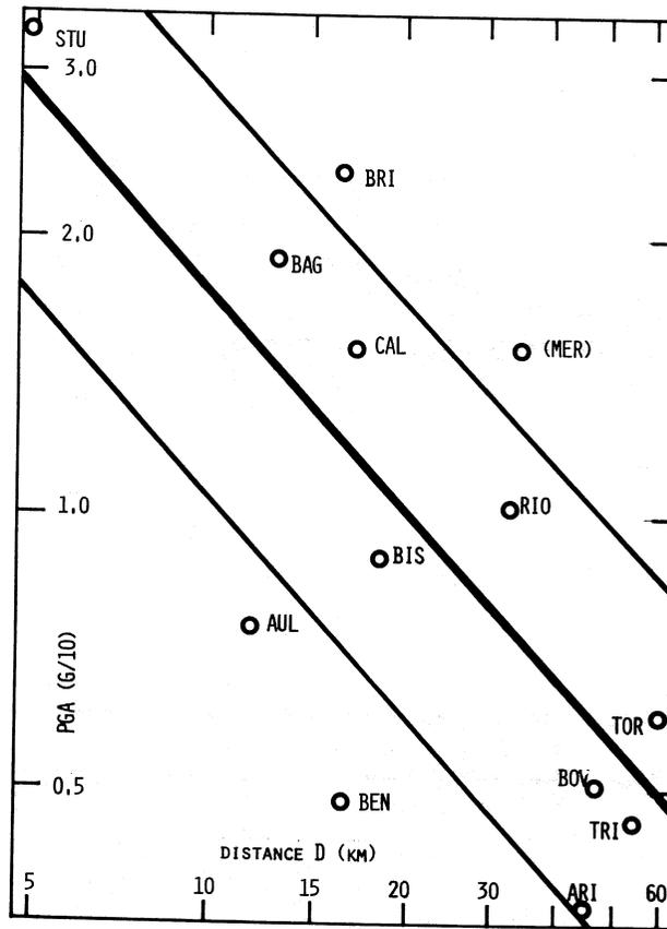
Fig. 4. Attenuation of PGA with distance from the horizontal projection of the assumed line source. Thin lines indicate the standard error of the estimate.
