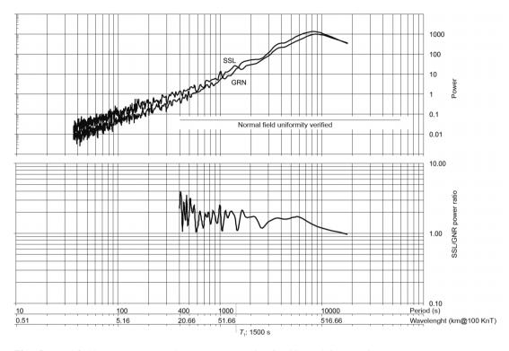
Fig. 5. Total field power spectra and power spectra ration for SSL and GRN stations.
