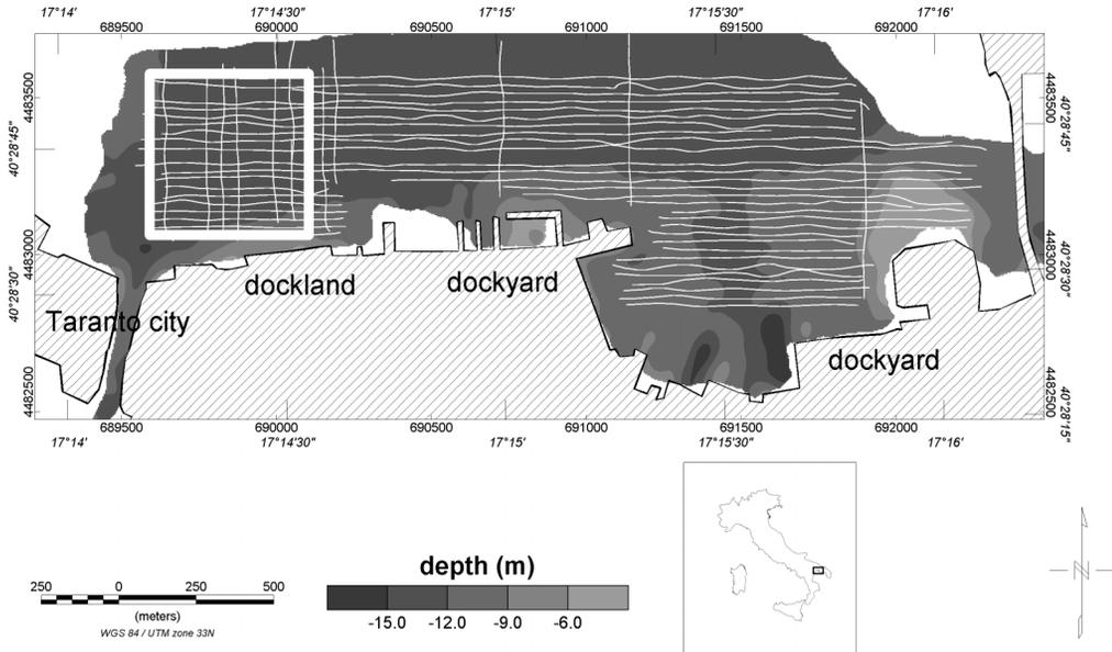
**Fig. 1.** Bathymetry of the survey area, main harbour infrastructure. The Taranto harbour is located on the south-eastern coast of Italy, approximately in the middle of the box on the bottom right map. The survey extent lines and ties path are indicated in white; in the boxed region on the left, all the horizontal components of the magnetic gradient are measured and the AS is evaluated.
