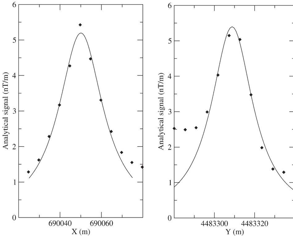
**Fig. 7.** Analytical signal least squares fit with a bell shaped function in order to estimate the depth of the source of anomaly n. 3.
