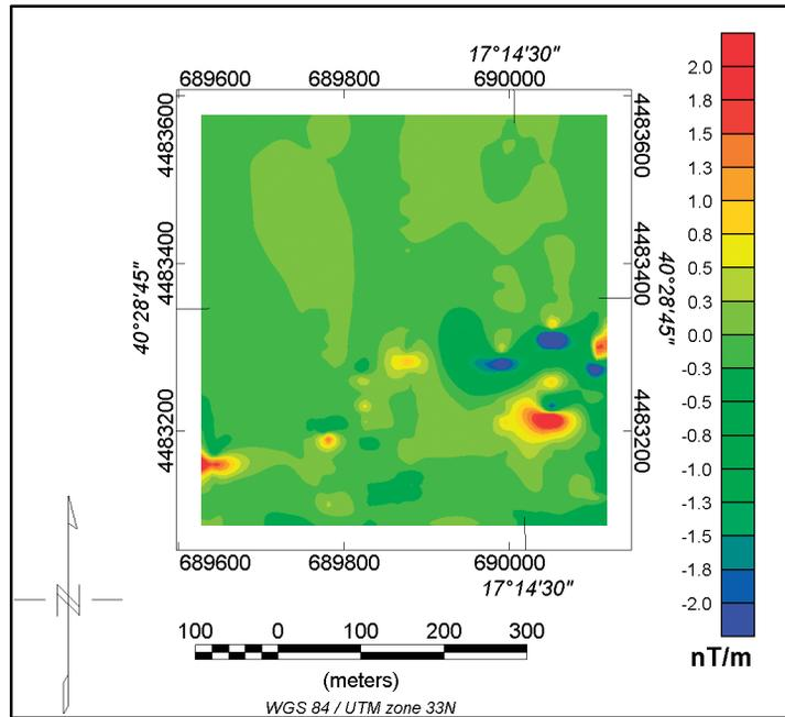
Fig. 3. Magnetic gradient: the east-west component.
