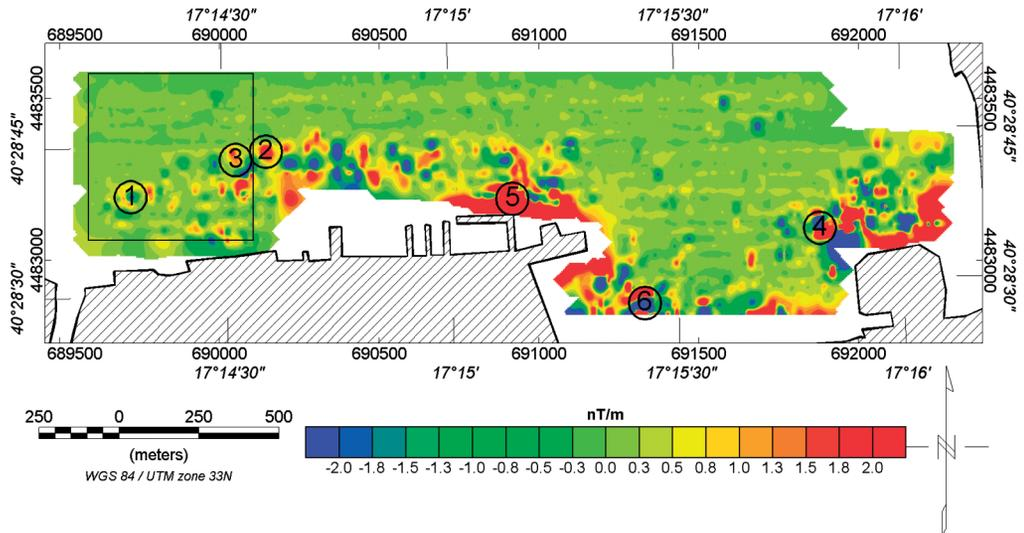
**Fig. 2.** Magnetic gradient: measured component in the north-south direction; the circles identify the actual object found on the seabed and listed in table I. The whole analytical magnetic signal was computed inside the box on the left. This is plotted in fig. 4.
