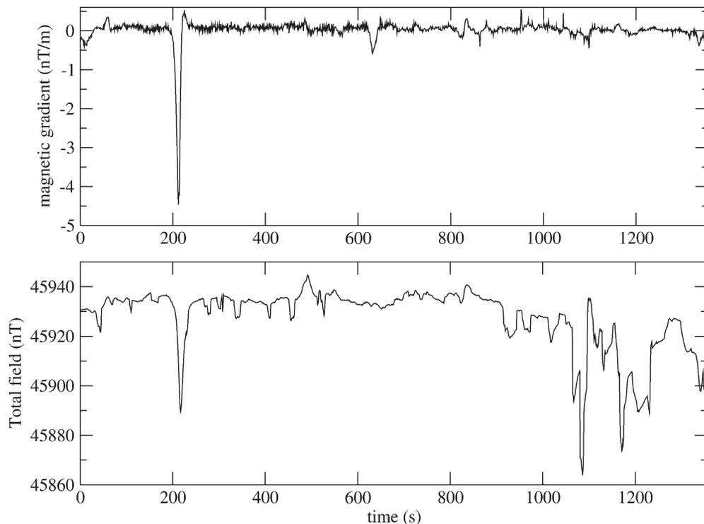
**Fig. 5.** Example of the magnetic signal (bottom panel) and gradient signal (upper panel) along a survey line. The large anomaly on the left is due to some magnetic sources, while the anomalies on the right, which are present only on the magnetic signal and not in the gradient, are probably due to anthropic noise.
