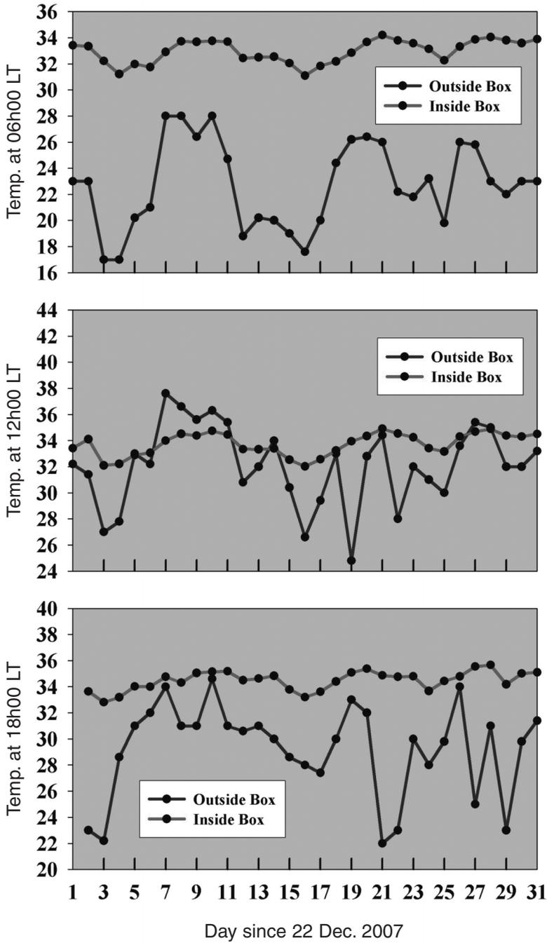
**Fig. 6.** The temperature variation at KMH Observatory as recorded inside the instrumentation box (grey curves) as well as measured outside by the Meteorological Office at the Keetmanshoop Airport at different times of the day (06h00,12h00, and18h00LT). Data shown are from 23 December 2007 till 22 January 2008.
