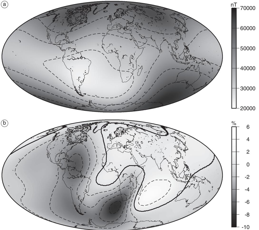
**Fig. 1a,b.** a) Global map of magnetic field intensity. The region of weakest intensity is known as South Atlantic Anomaly. (GRIMM Model, (Lesur *et al.*, 2008) b) Change of field intensity between 1979.85 and 2003.5 in percent (Difference between GRIMM and a model from MAGSAT data (Langel *et al.*, 1980).
