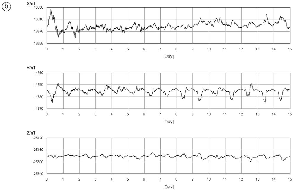
**Fig. 10a,b.** Examples for data from STH observatory. a) Measured (black dots) baselines for November 2007 to January 2008. The scatter of the first measurements will be reduced as the observer gains experience. b) One minute values of the north (X), east (Y) and vertical (Z) component for the time interval December 17 to 31, 2007.
