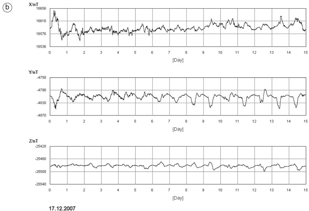
**Fig. 10a,b.** Examples for data from STH observatory. a) Measured (black dots) baselines for November 2007 to January 2008. The scatter of the first measurements will be reduced as the observer gains experience. b) One minute values of the north (X), east (Y) and vertical (Z) component for the time interval December 17 to 31, 2007.
