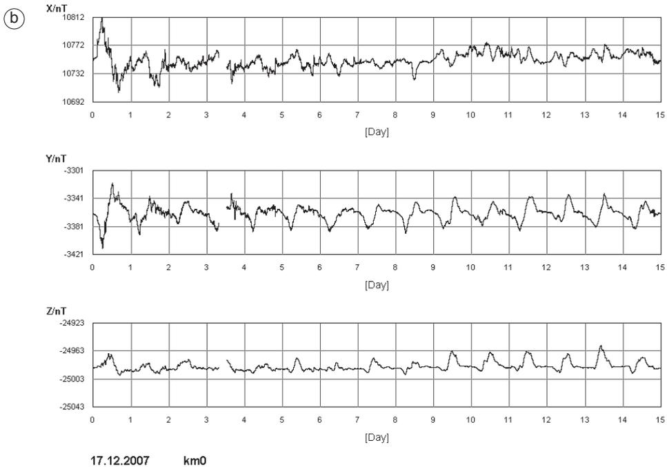
**Fig. 7a,b.** Examples for data from KMH observatory. a) Measured (black dots) and adopted (grey line) base lines for 2007. b) One minute values of the north (X), east (Y) and vertical (Z) component for the time interval December 17 to 31, 2007.
