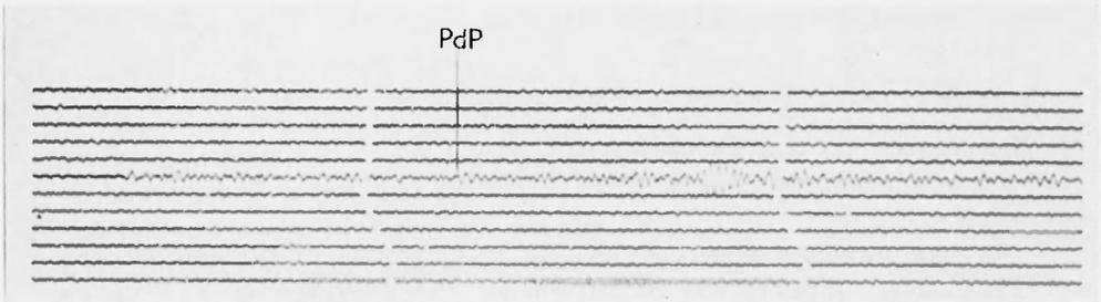
Fig. 3 - Earthquake of 1965 March 22, originating in Aegean basin, recorded at Messina station by a Sprengnether seismograph (vertical component, short period). *PdP* arrival indicated.
