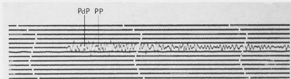
Fig. 6 - Earthquake of 1967 July 26, originating in Turkey, recorded at Messina station by a Sprengnether seismograph (vertical component, short period). *PdP* arrival indicated.
