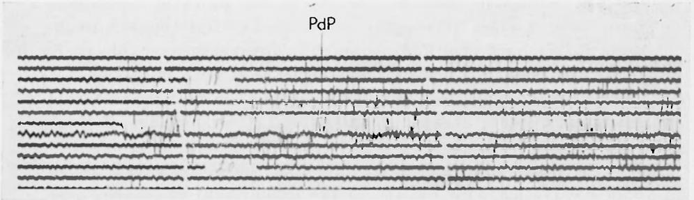
Fig. 2 - Earthquake of 1965 March 9, originating in Aegean basin, recorded at Messina station by a Sprengnether seismograph (vertical component, short period). *PdP* arrival indicated.
