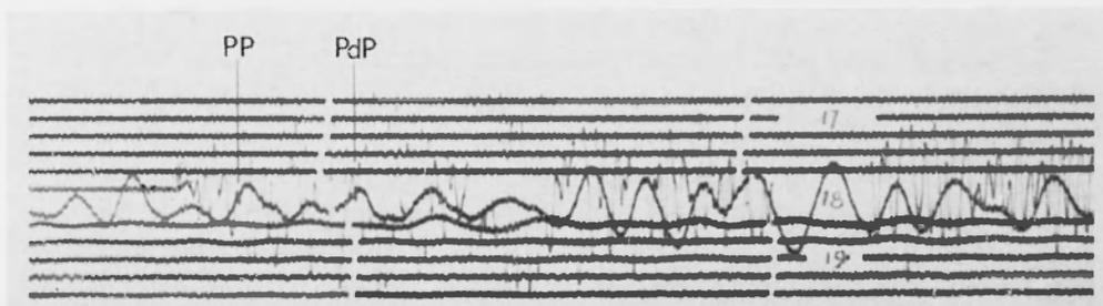
Fig. 5 - Earthquake of 1967 July 22, originating in Turkey, recorded at Messina station by a Sprengnether seismograph (vertical component, short period). *PdP* arrival indicated.
