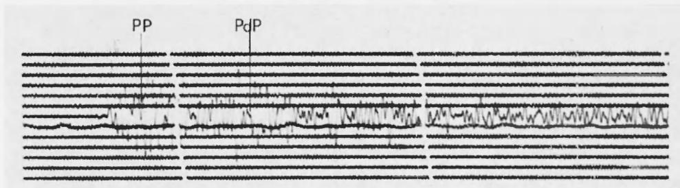
Fig. 7 - Earthquake of 1969 March 28, originating in Turkey, recorded at Messina station by a Sprengnether seismograph (vertical component, short period). *PdP* arrival indicated.
