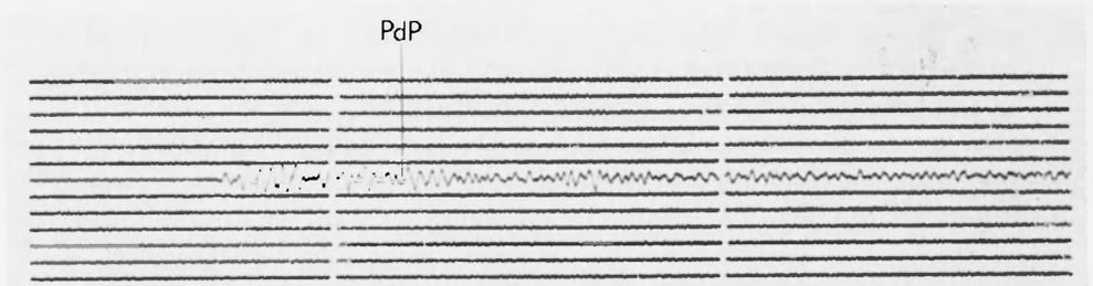
Fig. 4 - Earthquake of 1965 June 13, originating in Turkey, recorded at Messina station by a Sprengnether seismograph (vertical component, short period). *PdP* arrival indicated.
