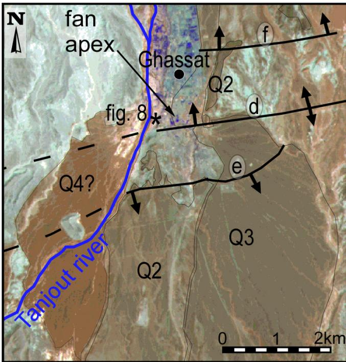
**Figure 9.** Map of the Quaternary deposits and surface flexures in the Tanjout area, on an ASTER image extract. South of Ghassat, an alluvial fan is sourced on the structure 'c'.
