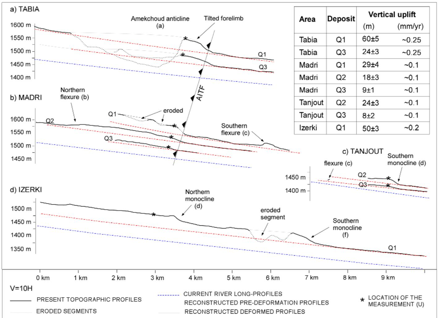
**Figure 6.** Topographic profiles projected onto lines perpendicular to the structures for the Tabia, Madri, Tanjout and Izerki areas. The profiles are vertically exaggerated 10-fold. Red dashed lines represent the reconstructed pre-deformation profile for each terrace. The table indicates the structural uplift measured (U) for each terrace. The sites where terrace heights were measured are indicated in the profiles.
