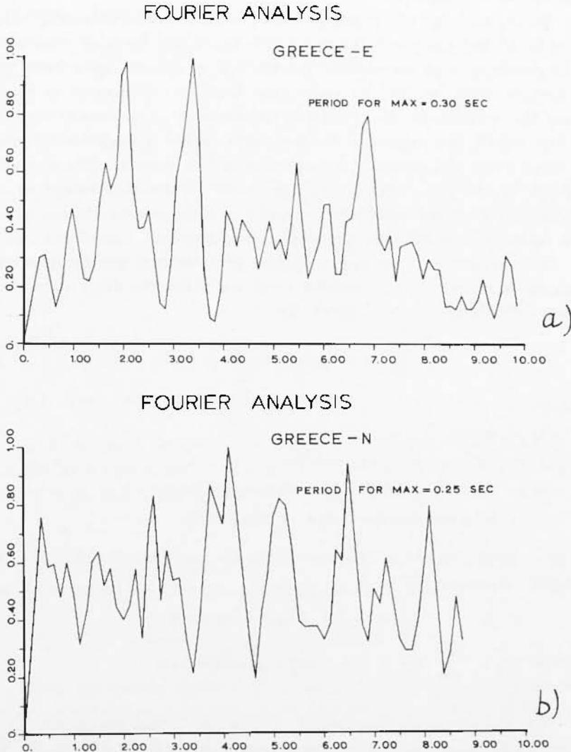
Fig. 9 - Fourier spectral density function of the main shock for the E-W (9a) and N-S (9b) accelerograms.
