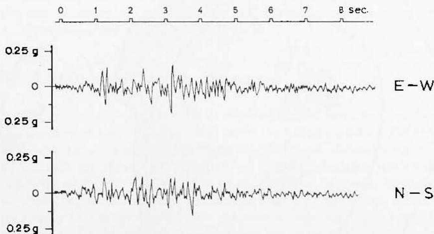
Fig. 2 - Records for the main shock of a SMAC-B type strong motion seismograph at Argostolion ( $38^{\circ}10'N$ ,  $20^{\circ}36'E$ ) on Cephallenia Island.
