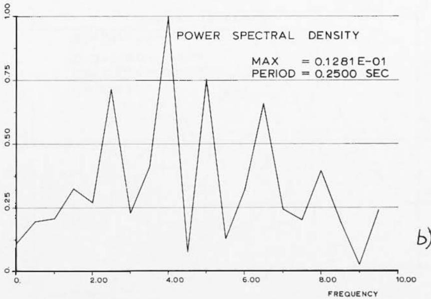
Fig. 7 - Power spectral density of the main shock for the E-W (7a) and N-S (7b) accelerograms.
