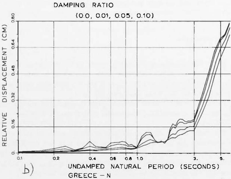
Fig. 11 - Relative displacements versus period and different damping ratios of the main shock for E-W (11a) and N-S (11b) components.
