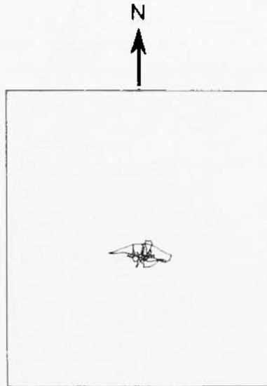
Fig. 3 - A 12 mm N100°E full-scale deflection of a SR-100 Wilmot seismoscope installed at the site of the strong motion seismograph.
