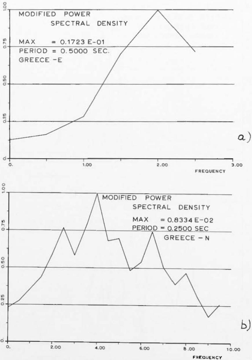
Fig. 8 - Modified power spectral density of the main shock for the E-W (8a) and N-S (8b) accelerograms.
