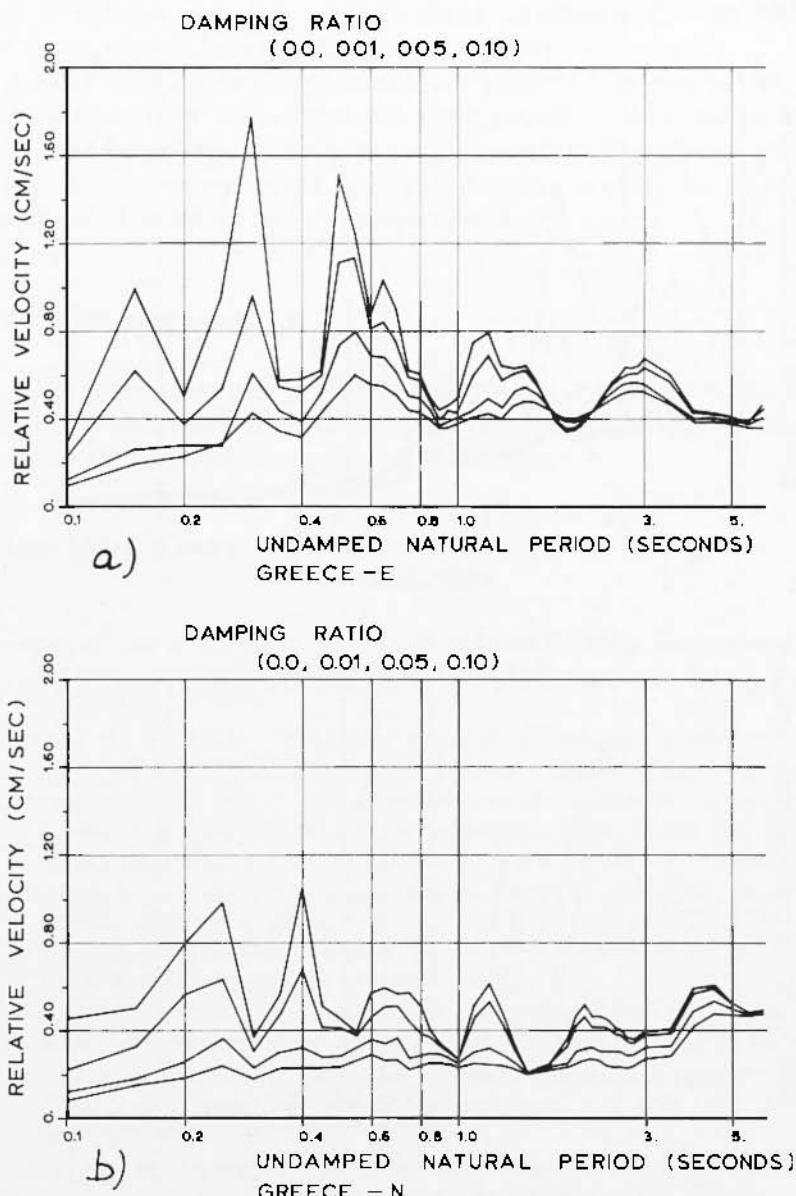
Fig. 12 - Relative velocities versus period and different damping ratios of the main shock for E-W (12a) and N-S (12b) components.
