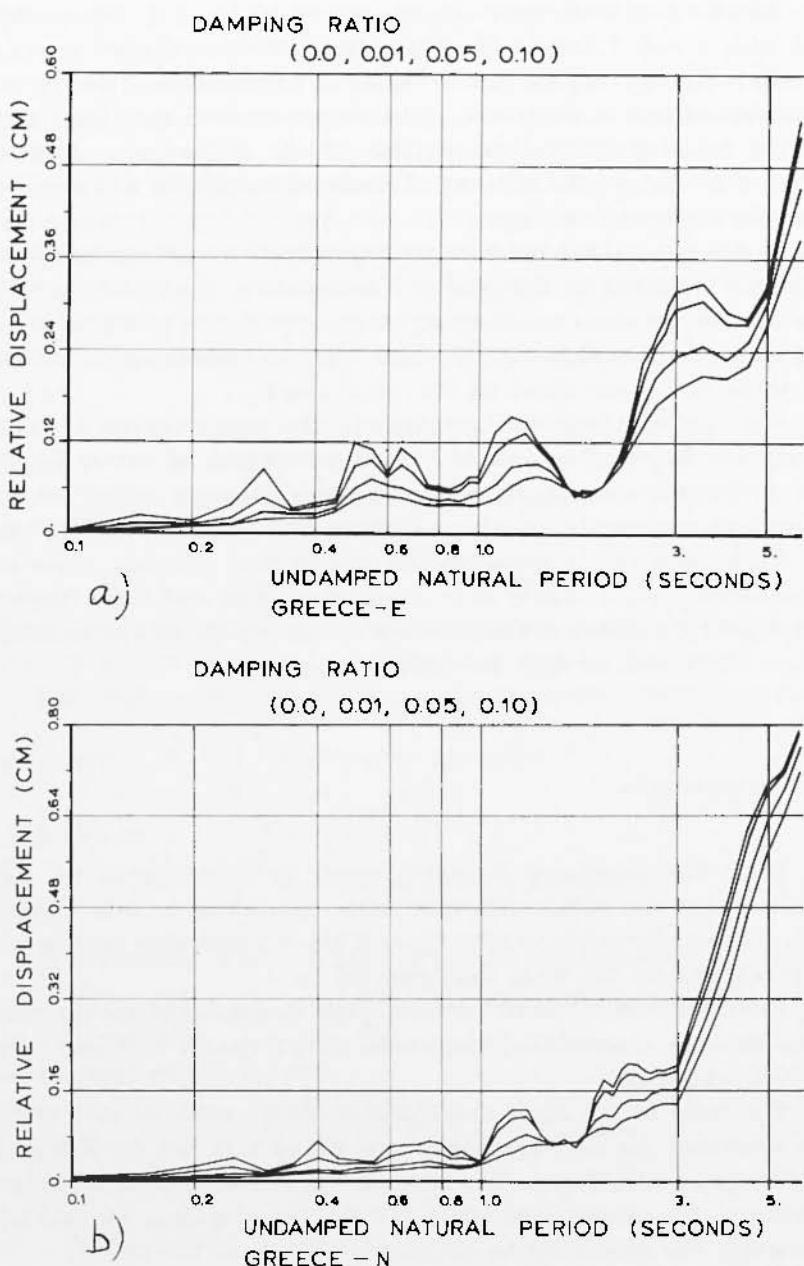
Fig. 11 - Relative displacements versus period and different damping ratios of the main shock for E-W (11a) and N-S (11b) components.
