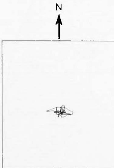
Fig. 3 - A 12 mm N100°E full-scale deflection of a SR-100 Wilmot seismoscope installed at the site of the strong motion seismograph.
