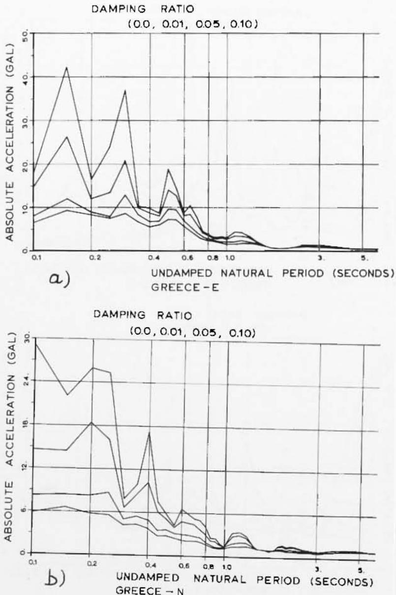
Fig. 13 — Absolute accelerations versus period and different damping ratios of the main shock for E-W (13a) and N-S (13b) components.
