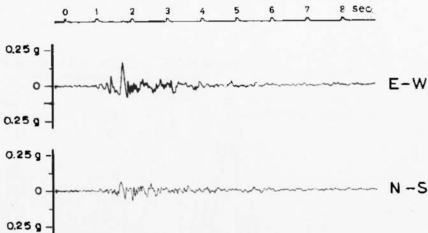
Fig. 5 - Records for the late aftershock of a SMAC-B strong motion seismograph at Argostolion ( $38^{\circ}10'N$ ,  $20^{\circ}36'E$ ) on Cephalenia Island.
