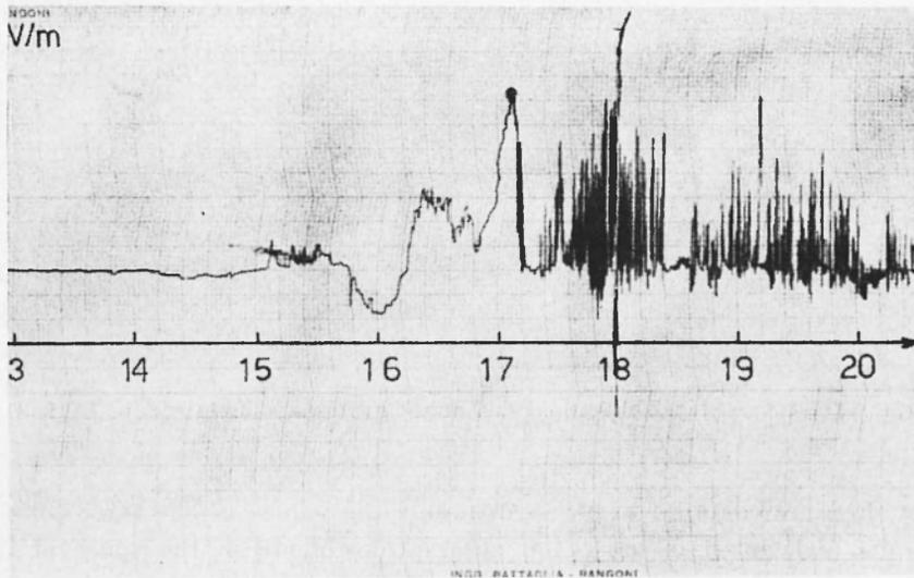
Fig. 10 - Polarity of the potential gradient during a snowfall at Macerata Observatory (Jan. 20, 1968).
