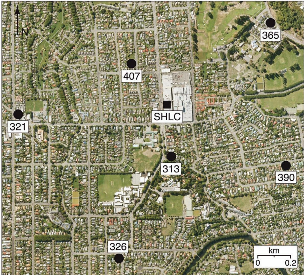
**Figure 4.** Map of the small-scale array of six QCN stations (circles) installed near the GeoNet station SHLC (square). The location of the map is shown in Figure 1. Additional information about each of the stations is given in Table 3.
