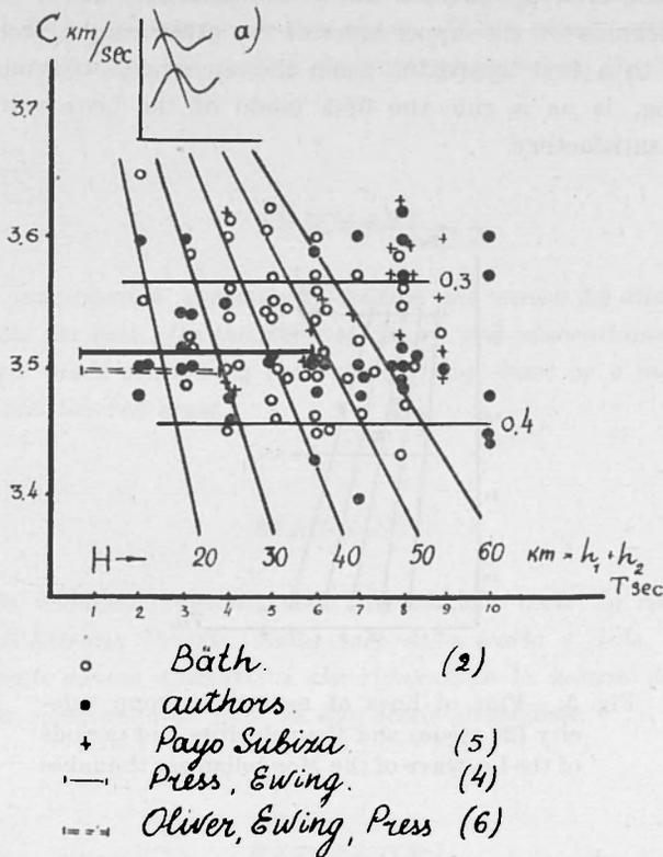
Fig. 4. — Plot of lines of maxima (group velocity 1st mode) and the velocity and period of the  $L_{g_1}$  wave by different authors.
