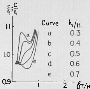
Fig. 3. — Plot of dispersion curves of Love waves in the two-layered crust.
