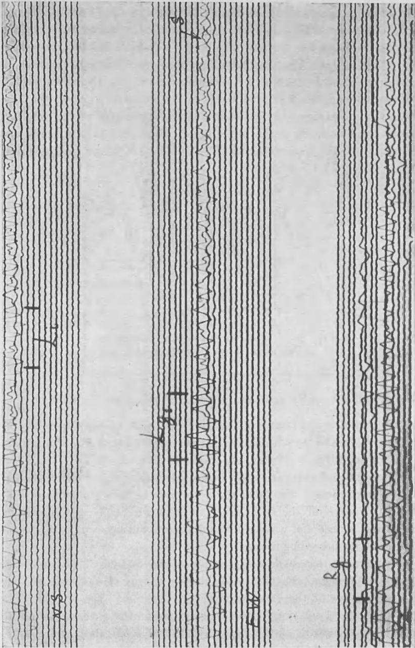
Fig. 2. - Copy of a seismogram of the seismic station Tiksi where Lg and Rg waves are absent.
