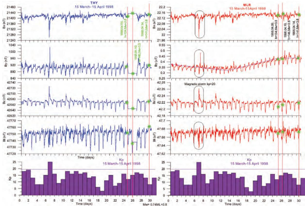
**Figure 5.** On March 21, 1998 (day 7) another magnetic storm ( $K_p = 25$ ) induced a variation in the geomagnetic flux density. It can be seen that the  $B_y$  component has a V-shaped anomaly, which ends on day 25 (April 9, 1998). Two earthquakes ( $M_w = 3.8$  h = 134 km, and  $M_w = 3.5$  h = 146 km, respectively) occurred on April 9, 10, 1998.
