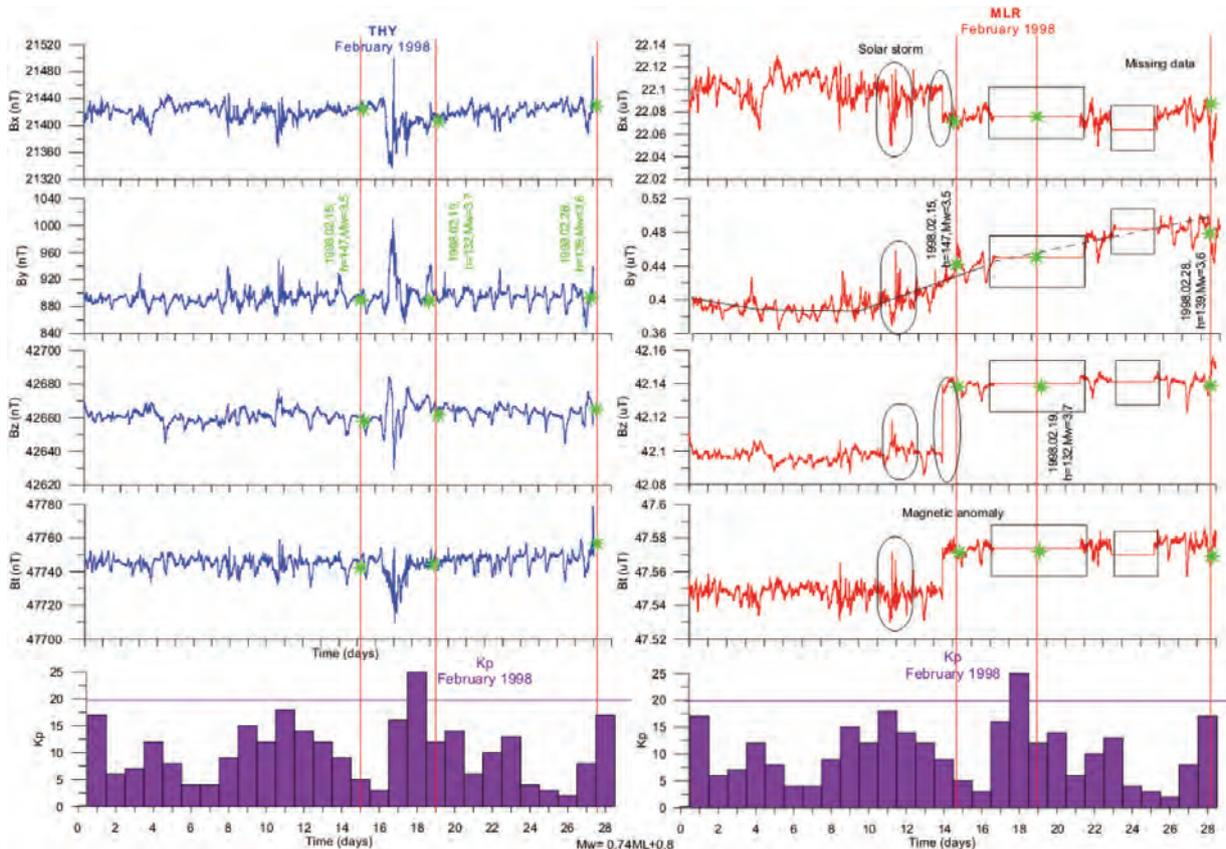
**Figure 4.** The V-shaped anomaly of *By* started on January 23, 1998 (see Figure 2), and continued until February 15, 1998, when the prior value of *By* was restored. One day before restoration, a step-change occurred on the *Bx* and *Bz* components. An earthquake with magnitude *Mw* = 3.5 (*h* = 147 km) occurred on February 15, 1998. Between February 17 to 21, 1998, there was a data gap. The same situation is seen for February 23 to 25, 1998.
