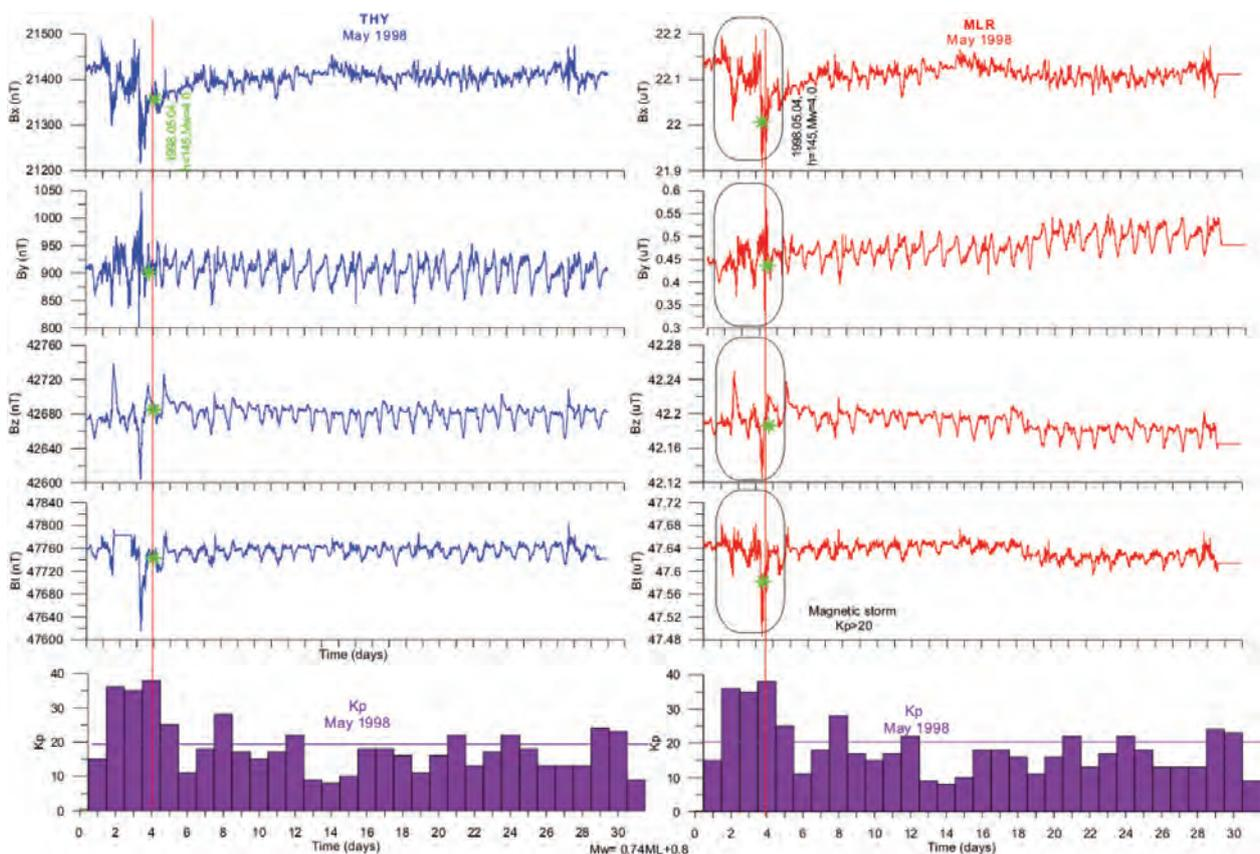
**Figure 2.** Solar storm that took place on May 2, 3, 4, 1998, had a triggering effect on the earthquake that occurred on May 4, 1998  $M_w 4.0$ ;  $h = 145$  km). In this case, the geomagnetic anomaly was induced by the solar storm (as the  $Kp$  index reveals) and it is not a seismo-magnetic precursor.
