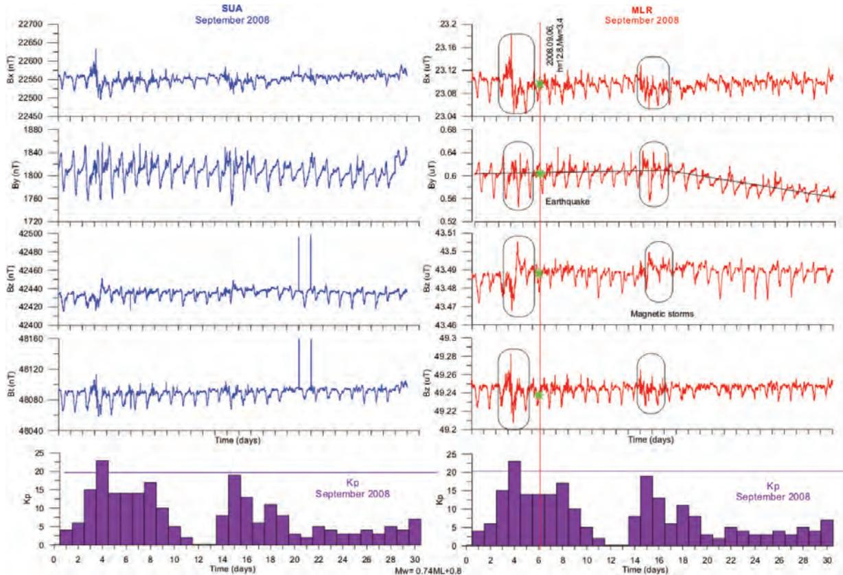
Figure 6. The V-shaped anomaly recorded on the horizontal component  $B_y$  of the MLR Observatory data prior to the  $M_w = 4.4$  (October 2, 2008) crustal Vrancea earthquake.
