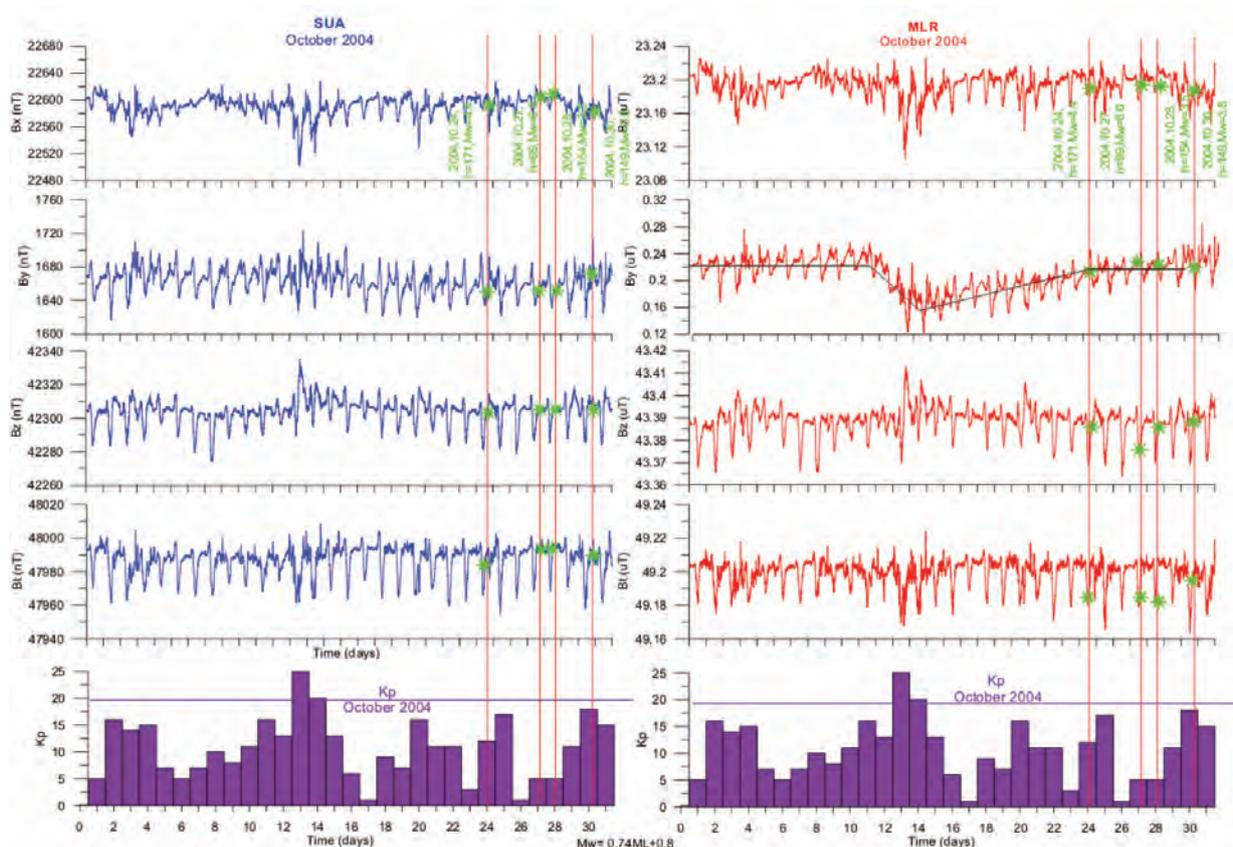
Figure 8. The V-shaped anomaly recorded on the horizontal component  $B_y$  of the MLR Observatory data prior to the  $M_w = 6.3$  (October 27, 2004) intermediate depth Vrancea earthquake.
