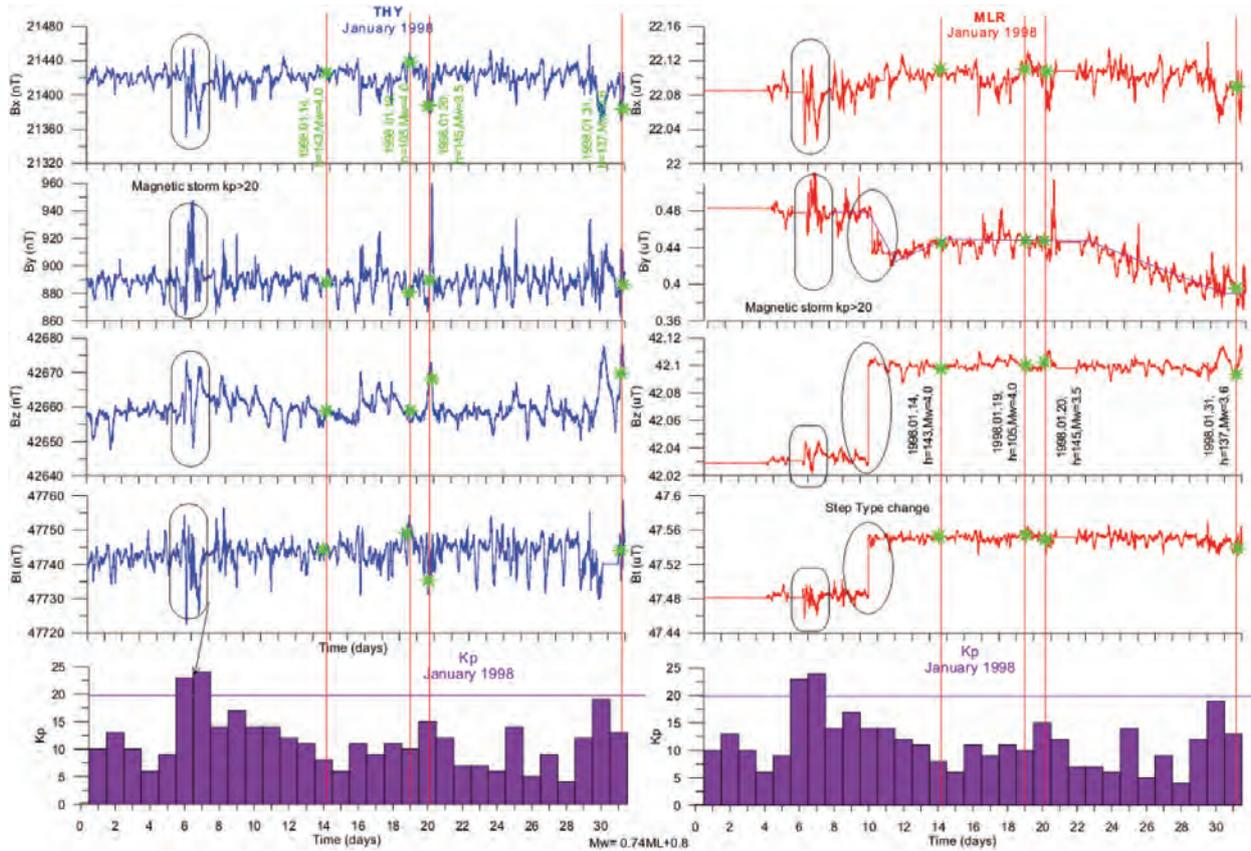
**Figure 3.** *Kp* indices of January 6, 7, 1998, reveal a magnetic storm. Two days later, on January 10, 1998, a step-change of *Bz* and *By* occurred. The *By* component developed a V-shaped anomaly with a duration of 4 days. An earthquake with magnitude *Mw* 4.0 (*h* = 143 km) occurred at the end of this anomaly.
