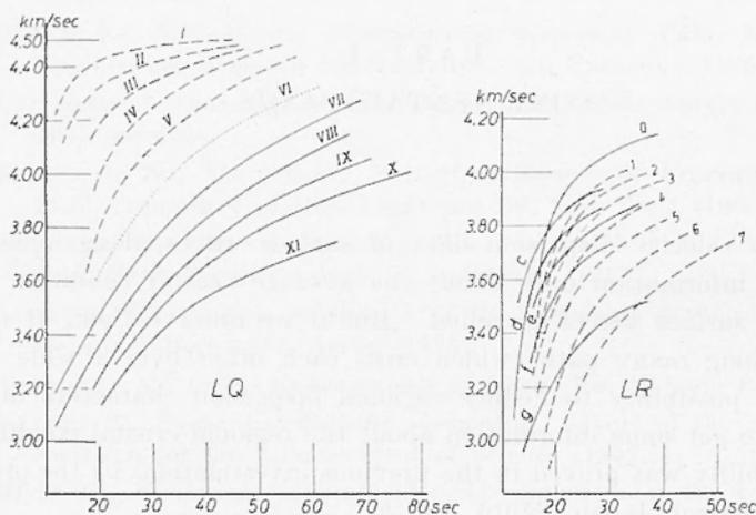
Fig. 1 - Classified dispersion curves of Love (left) and Rayleigh (right) waves.
