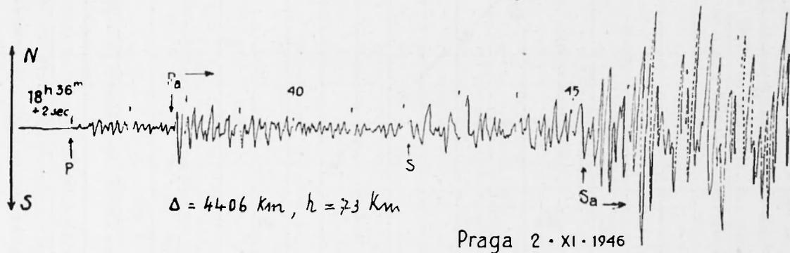
Wiechert 1000 kg.  $T_0 = 9,5^s$   $V_0 = 193$   $\epsilon = 4,7:1$   $\frac{r}{T_0^2} = 0,003_3 \frac{mm}{sec^2}$
