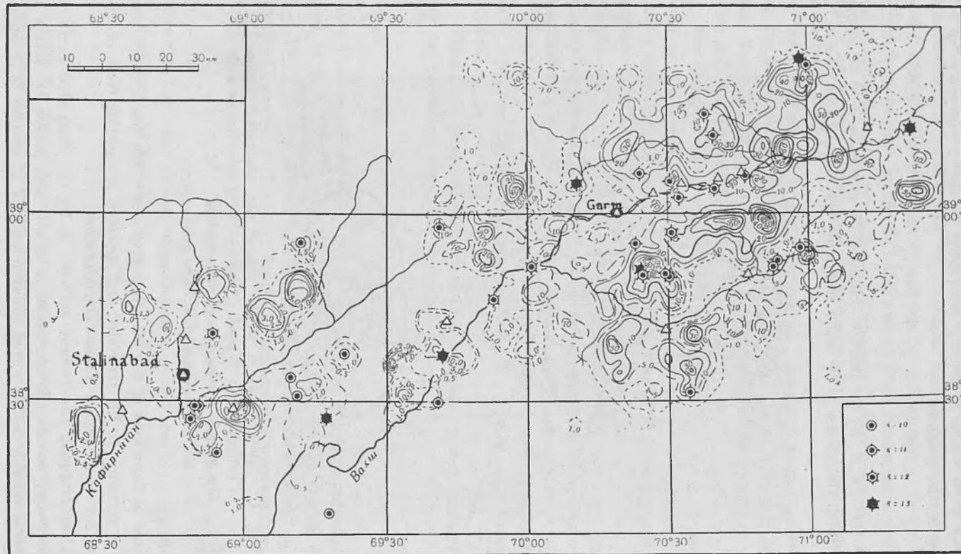
Fig. 5 - Schematic map of the seismic activity of the Garm-Stalinabad region, 1955-1957.
