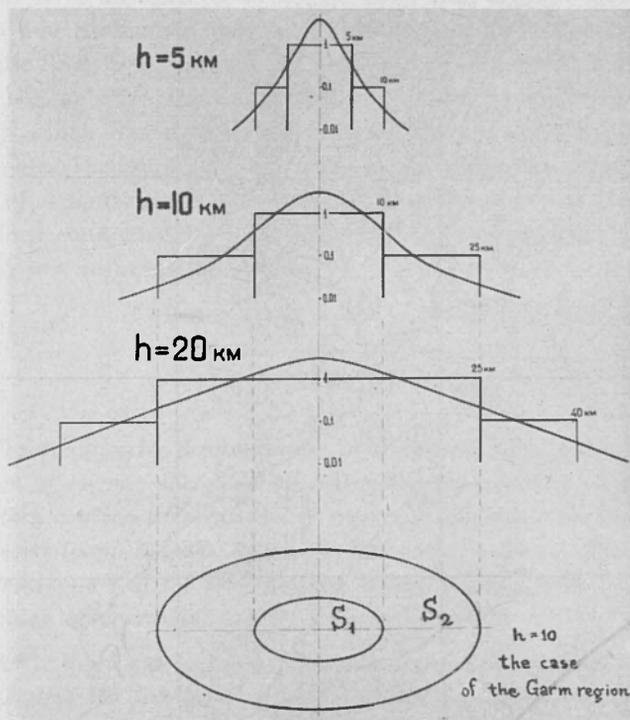
Fig. 4. - Determination of the size of the averaging region to calculate the Seismic Activity  $A$  in accordance with the seismic waves energy attenuation.
