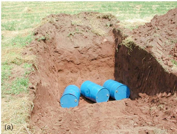
urban area that is today subjected to high electromagnetic interference. Three metal drums were buried at a depth of 2 m. Two more drums, one in a vertical position and the second in a horizontal position, were placed at a safe distance from the other three drums. In addition, a 1-m-length of railway track that weighed about 80 kg was also buried 1 m deep.
