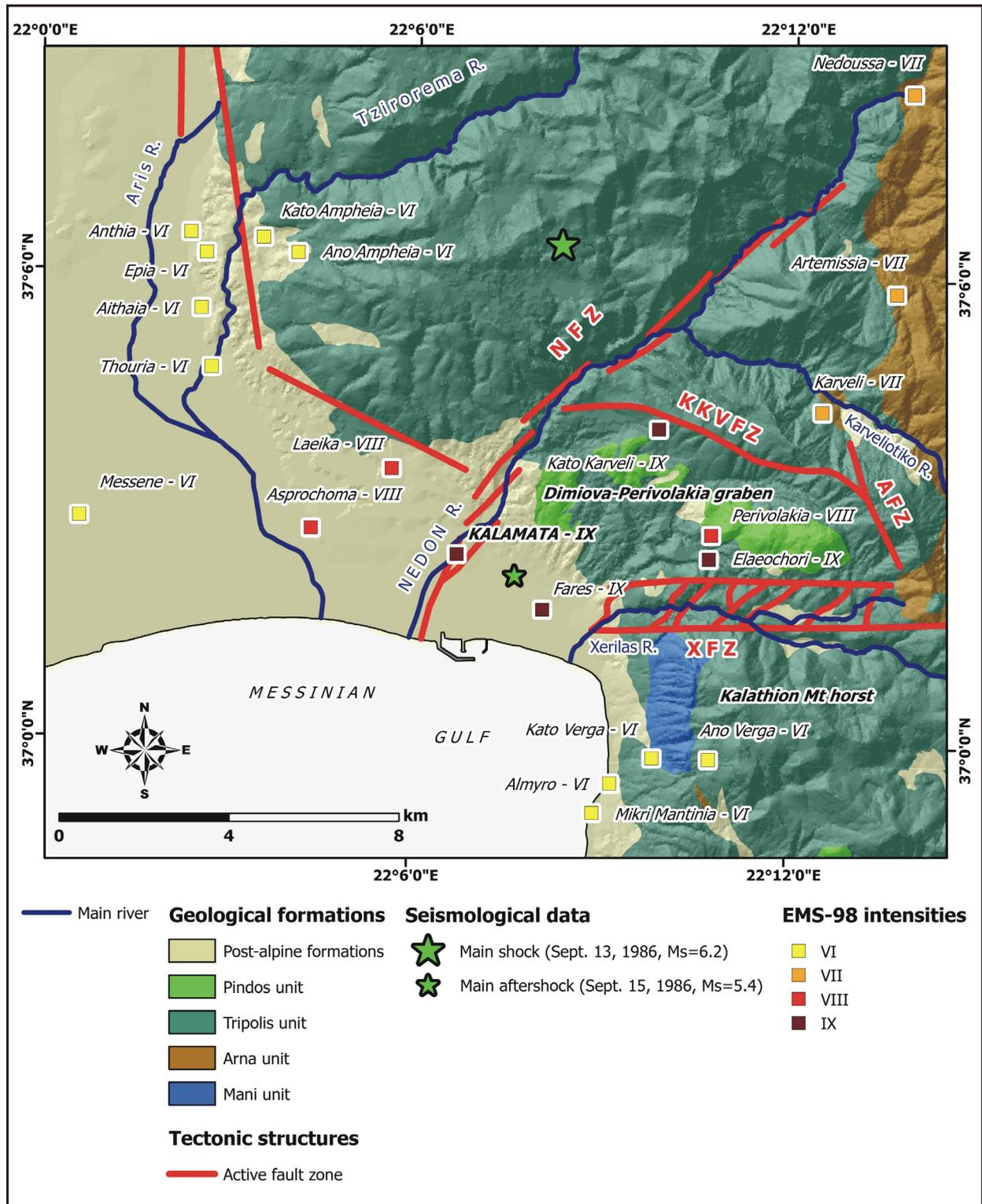
**Figure 6.** Geological map depicting the seismic intensities derived from the application of the EMS-98 scale to the September 13, 1986, Kalamata earthquake and their correlation with the neotectonic structures and the active fault zones of the study area (NFZ: Nedon fault zone, KKVfZ: Kato Karveli-Venitsa fault zone, AFZ: Arachova fault zone, XFZ: Xerilas fault zone).
