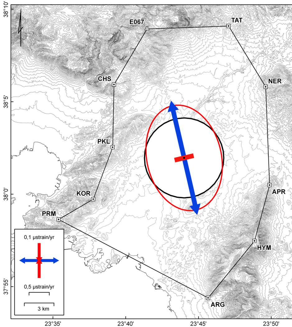
**Figure 4.** Principle axes of the strain rate tensor for the area of interest, calculated from velocities of selected GPS sites, in background topographic contour lines of 20m interval. An extension rate of  $0.27 \pm 0.06 \cdot 10^{-6} \text{ yr}^{-1}$  along a NNW-SSE direction ( $N 347^\circ$ ) is calculated.
