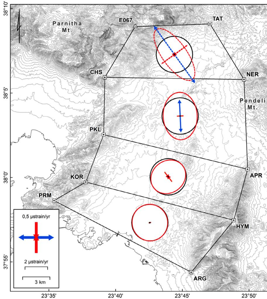
**Figure 5.** Principle axes of the strain rate tensors within Athens Basin. Dashed lines indicate local estimates around which GPS data are poorly distributed from a geometrical point of view. This figure shows negligible compressional rates at the southern part of the basin compared to the dominant extensional regime of gradually higher strain rates northwards up to  $0.91 \pm 0.09 \cdot 10^{-6} \text{ yr}^{-1}$  towards the northern part of the network between the Pendeli and Parnitha ranges.
