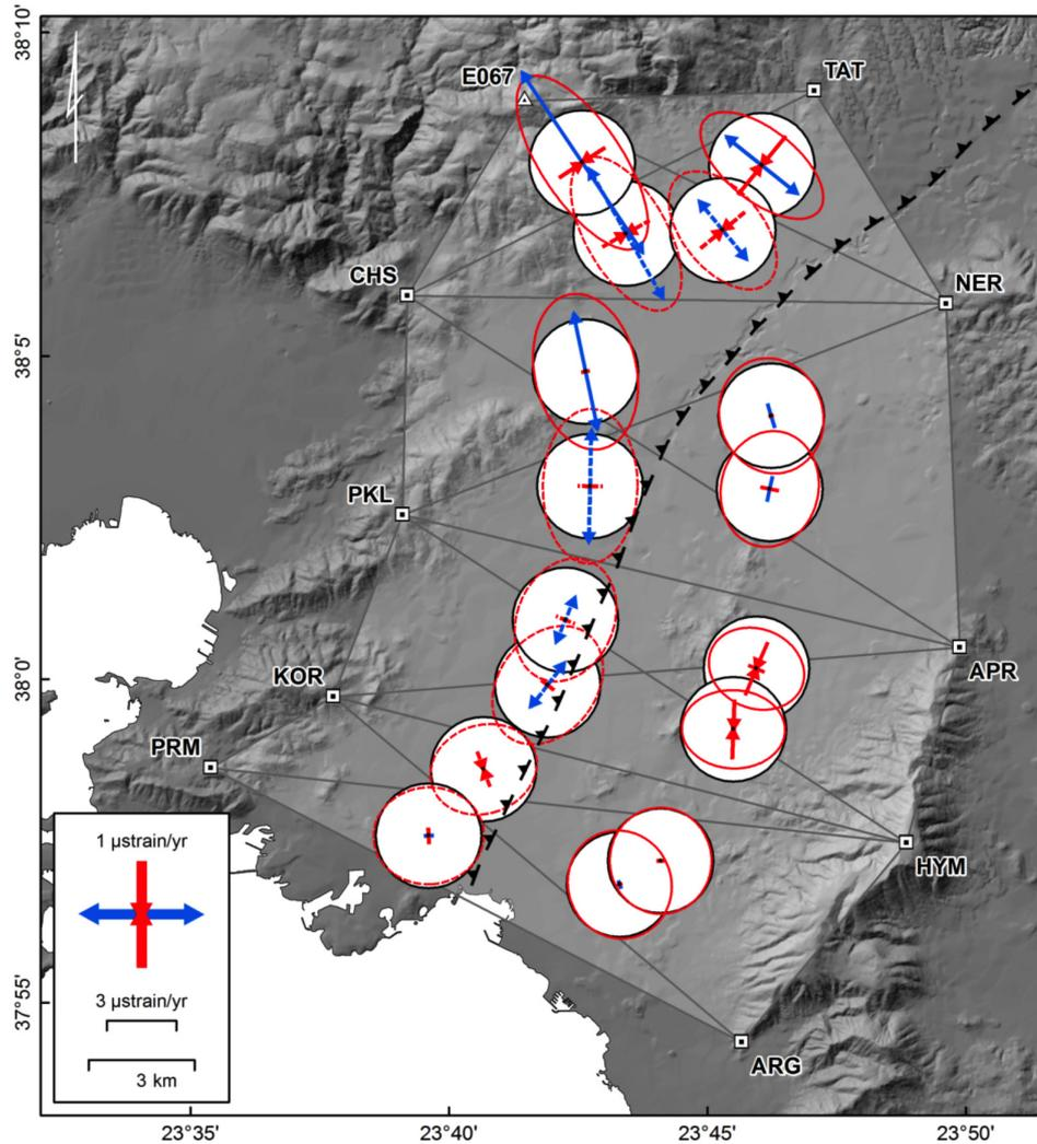
**Figure 6.** Detailed strain analysis by different triangulations of selected GPS sites. Principle axes of the strain rate tensors are calculated at the center of mass of each triangle. The approximate location of the tectonic boundary separating metamorphic and non-metamorphic alpine rocks in Attica is shown (dashed line). There is a significant strain-rate difference on either side of the boundary.
