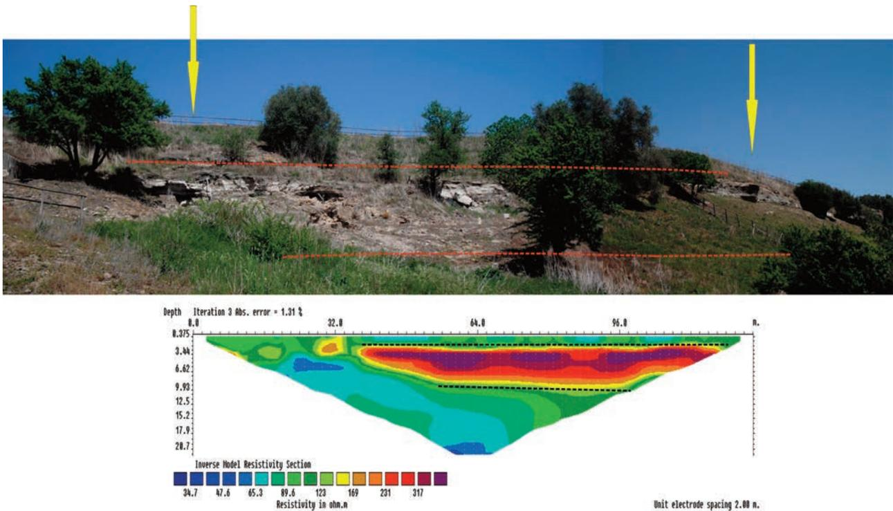
Figure 10. Electric Resistivity Tomography performed on a outcrop.
