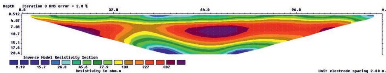
Figure 11. Electric Resistivity Tomography performed on *Ostera Necropolis*.
