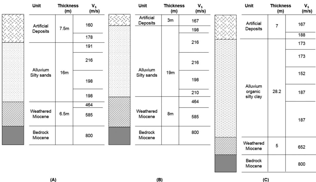
**Figure 10.** Soil profiles used to calibrate the  $V_s$  values: (A) S5; (B) S9; (C) S32
