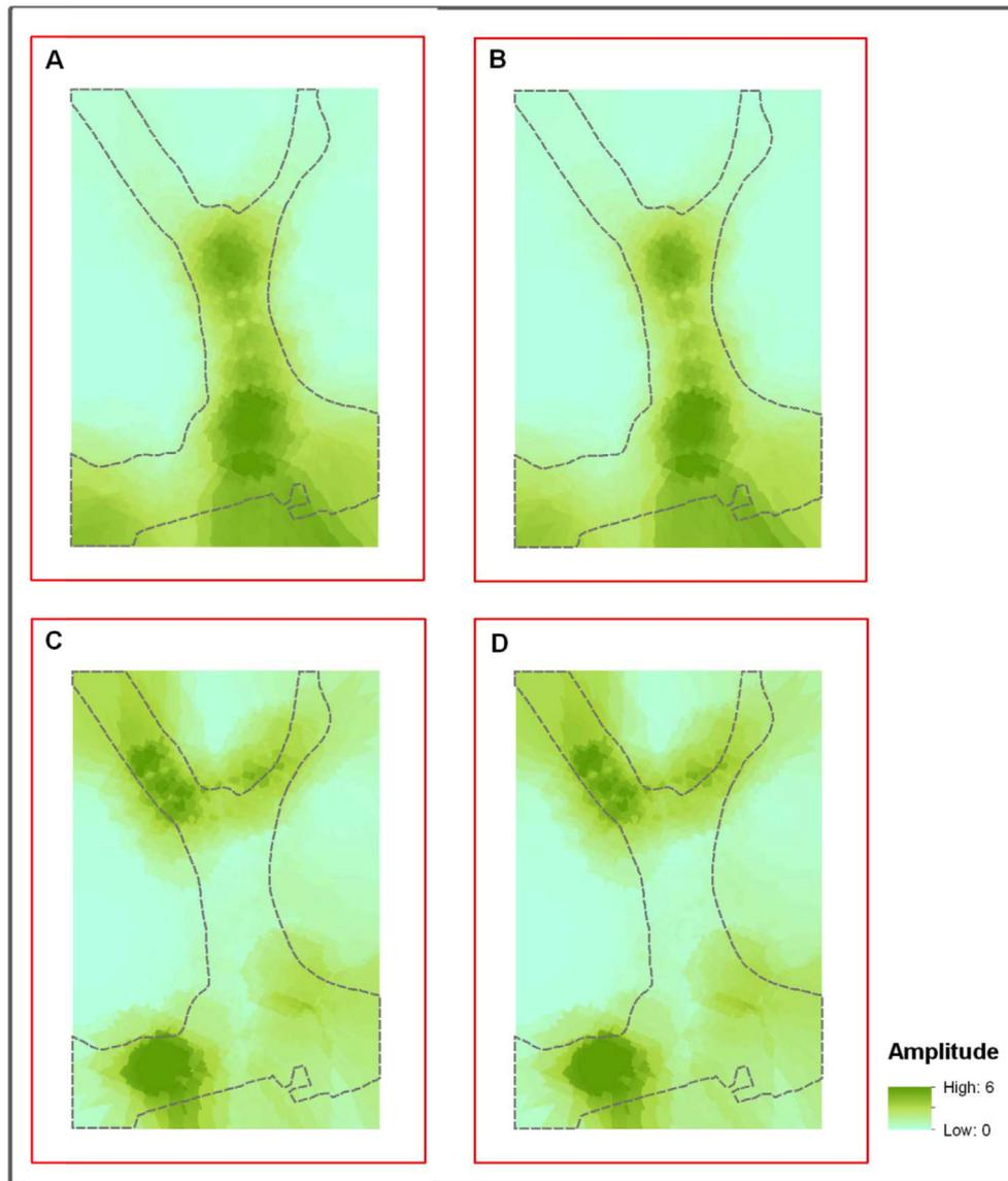
**Figure 15.** Spectral amplitude at 1 Hz (top) and 2.5 Hz (bottom) for a near-field seismic motion (left) and a far-field seismic motion (right).
