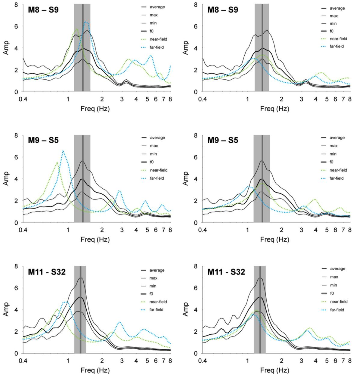
**Figure 12.** Comparison between the computed transfer functions and the H/V curves obtained from ambient vibration analysis. Left: transfer functions computed with the first estimated  $V_S$  values. Right: transfer functions computed with the final estimated  $V_S$  values.
