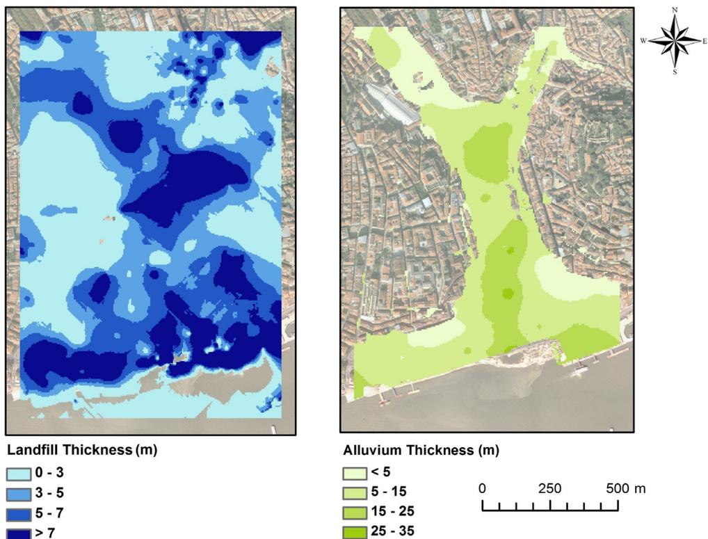
Figure 3. Thickness of anthropogenic deposits (left) and alluvial deposits (right) in Baixa.
