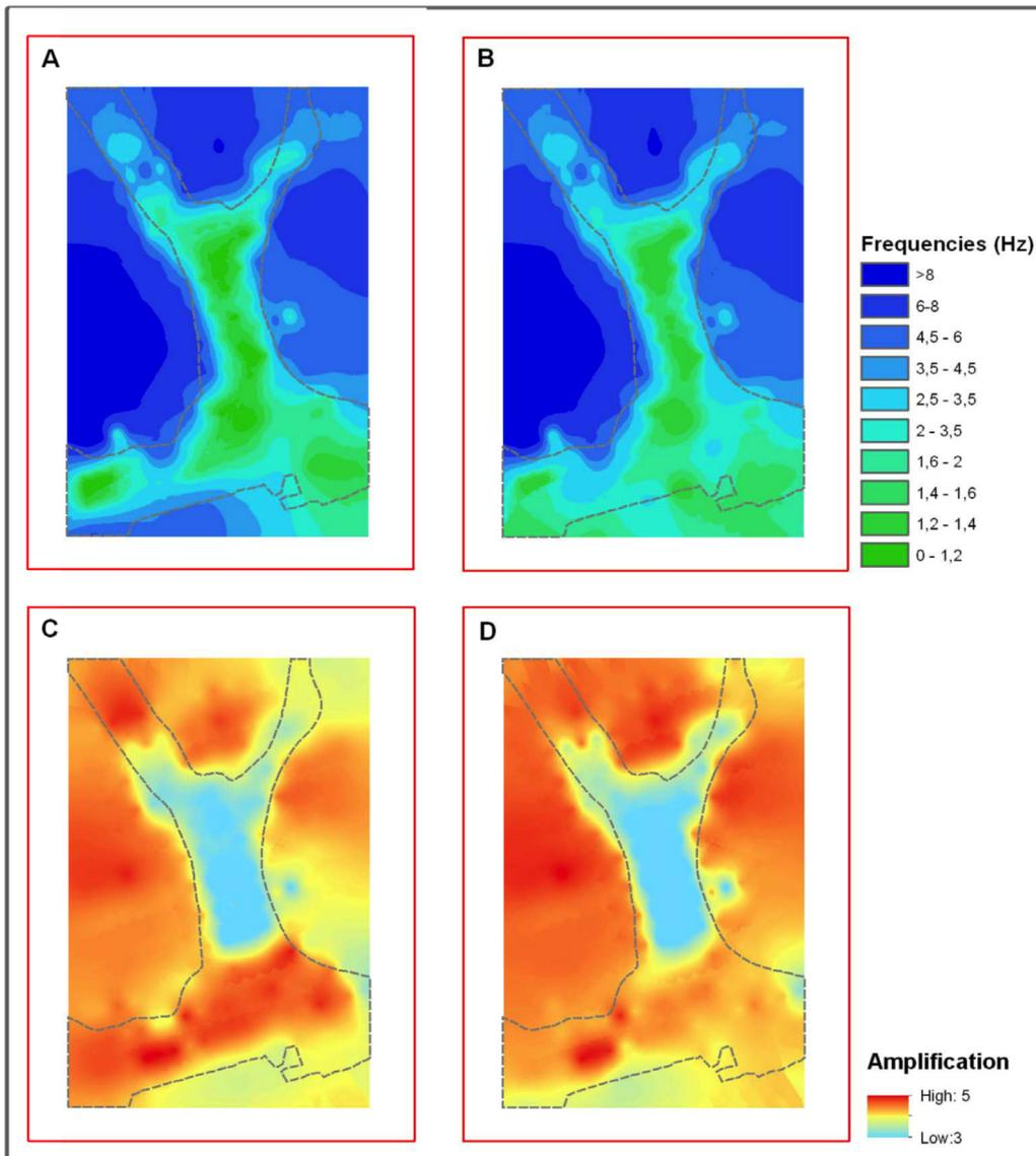
**Figure 14.** Fundamental frequencies (top) and the corresponding amplifications (bottom) for a near-field seismic motion (left) and a far-field seismic motion (right).
