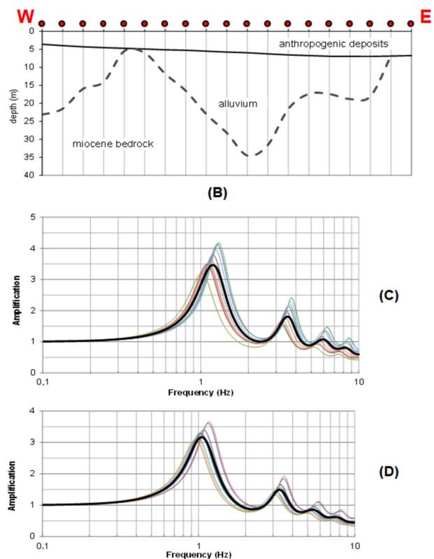
**Figure 13.** Location of the 256 soil profiles for which the transfer functions were computed (A). Example of one cross section performed to define the soil profiles (B). Transfer functions computed for 10 near-field (C) and 10 far-field (D) seismic motions for an arbitrary profile. The black bold curves are the mean transfer functions for each type of motion.
