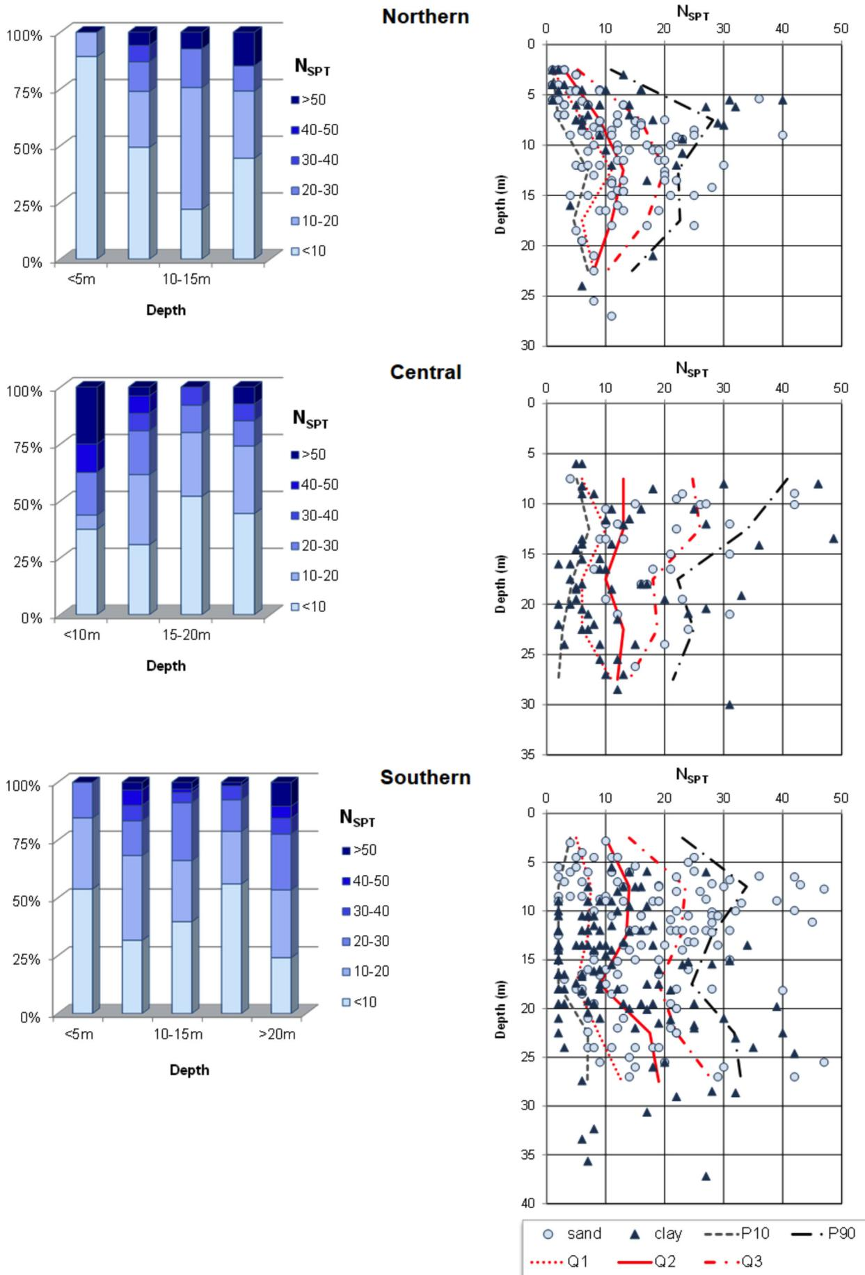
**Figure 5.** Distribution of  $N_{SPT}$  values in the alluvial deposits for the three zones. Left: histograms of  $N_{SPT}$  for different depths. Right: distribution of  $N_{SPT}$  (< 50) with depth for clayey and sandy materials. Percentiles lines (in black) and quartiles lines (in red) are also presented.
