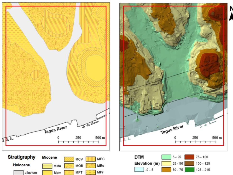
**Figure 2.** Left: Surface geology of the Baixa area (adapted from Pais et al. [2006]). The central part is filled by alluvial sediments covering Miocene formations (see lithological composition in the text). Right: Digital terrain model (DTM) obtained from a 1:1000 survey scale. Dashed black lines separate the three defined zones (north, central and south).
