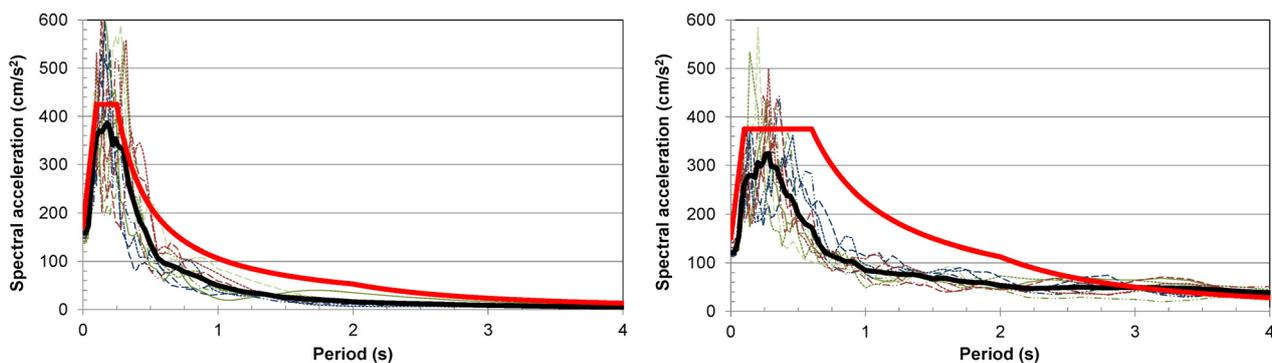
**Figure 11.** Response spectra for the 10 seismic motions computed for each source: (left) near-field seismic motion; (right) far-field seismic motion. The mean of the 10 spectra are presented in bold (black curve). Bold red curve: Portuguese seismic code response spectra for 475 year return period.
