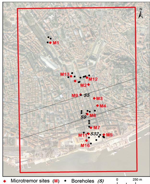
Figure 8. Location of the ambient vibration measurements (M) and the closest geotechnical boreholes (S). Boreholes used to calibrate the  $V_s$  values are identified. The dashed black lines separate the three defined zones (northern, central and southern).
