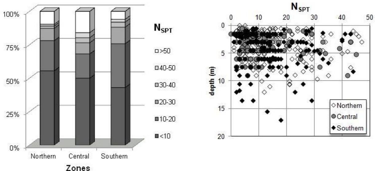
**Figure 4.** Distribution of  $N_{SPT}$  values in the anthropogenic deposits for the three zones. Left: histograms of  $N_{SPT}$  for depths less and greater than 5 m. Right: distribution of  $N_{SPT}$  ( $< 50$ ) with depth.
