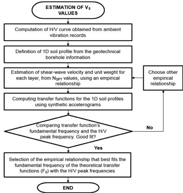
Figure 7. Synthesis of the procedure for estimating the  $V_s$  values for each layer. The empirical relationships used are presented in Table 4.
