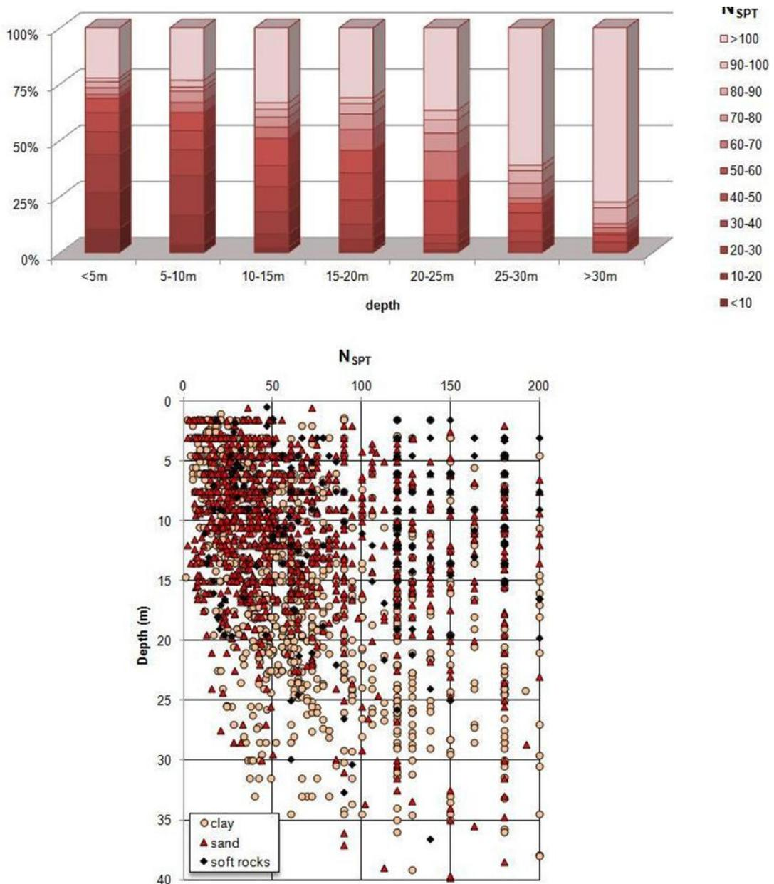
Figure 6. Distribution of  $N_{SPT}$  values in the Miocene bedrock (excluding 10% of the tests with  $N_{SPT}$  values greater than 200). Top: histograms of  $N_{SPT}$  values for different depths. Bottom: distribution of  $N_{SPT}$  values with depth.
