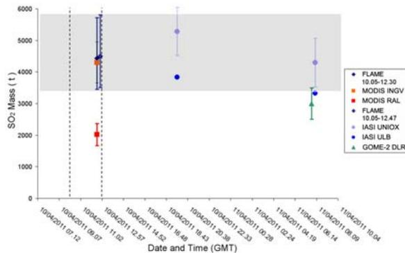
**Figure 4:** SO<sub>2</sub> Mass comparison ground vs satellite measurements across Mt. Etna for the 10 April 2011 paroxysmal event.
