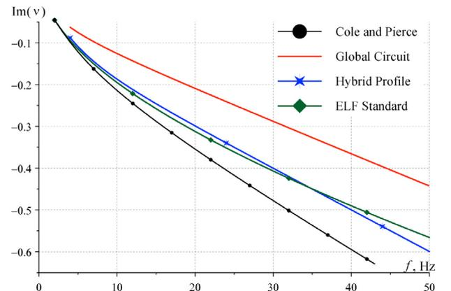
**Figure 3.** Imaginary part of the ELF propagation constant obtained with the full wave solution for the Cole and Pierce [1965] profile (black line with dots); profile based on the global circuit data (red smooth line); the hybrid profile (blue curve with stars). The ELF Standard reference model (Equations 10 to 13) is shown by the green curve with diamonds.
