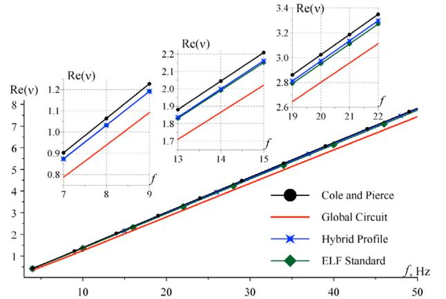
**Figure 2.** Real parts of the ELF propagation constant obtained with the full wave solution for the Cole and Pierce [1965] profile (black line with dots); profile based on the global circuit data (red smooth line); the hybrid profile (blue curve with stars). These are compared with the reference model (green curve with diamonds).
