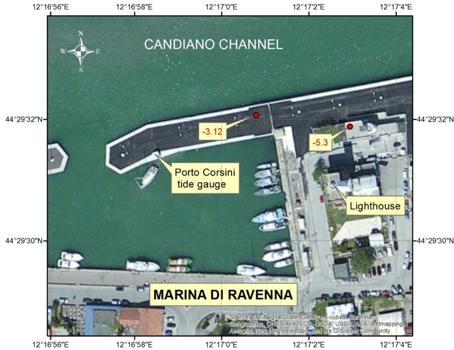
**Figure 3.** Aerial view of Marina di Ravenna showing the Porto Corsini tide gauge station and the surroundings. The ARPAE benchmark is sited in the same place of the tide gauge. The altimetric reference is the benchmark of the lighthouse. Red dots mark the scatter points from the interferometric satellite considered in this work, for the period 2006-2011 (units are  $\text{mm yr}^{-1}$ ).
