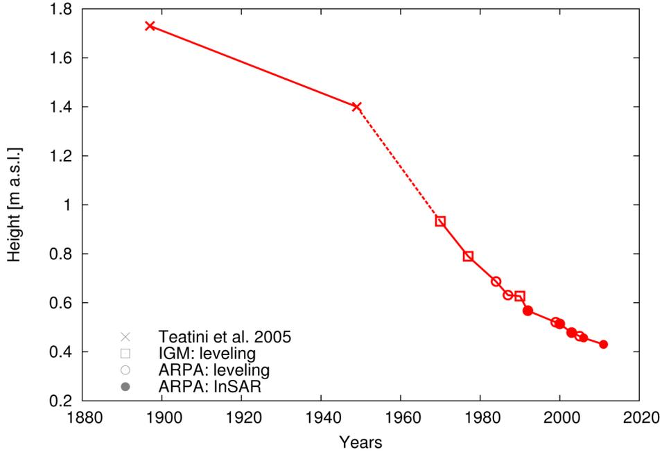
**Figure 4.** Altitude measurements in Marina di Ravenna at various epochs. Given the various elaborations applied to data before 1970 (see Section 2.2), the association with the 1970 IGM leveling is approximate (dashed line). Data after 1970 refer to different sources and survey methods, marked by various symbols (see legend). Further details are given in Tables 1 and 2.
