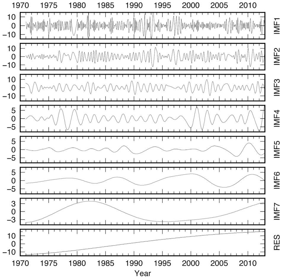
**Figure 5.** Results of the EMD analysis of the Marina di Ravenna relative sea-level time series since 1970, with the IMFs in the top frames and the residual (RES) in the bottom, respectively. Units are cm throughout.
