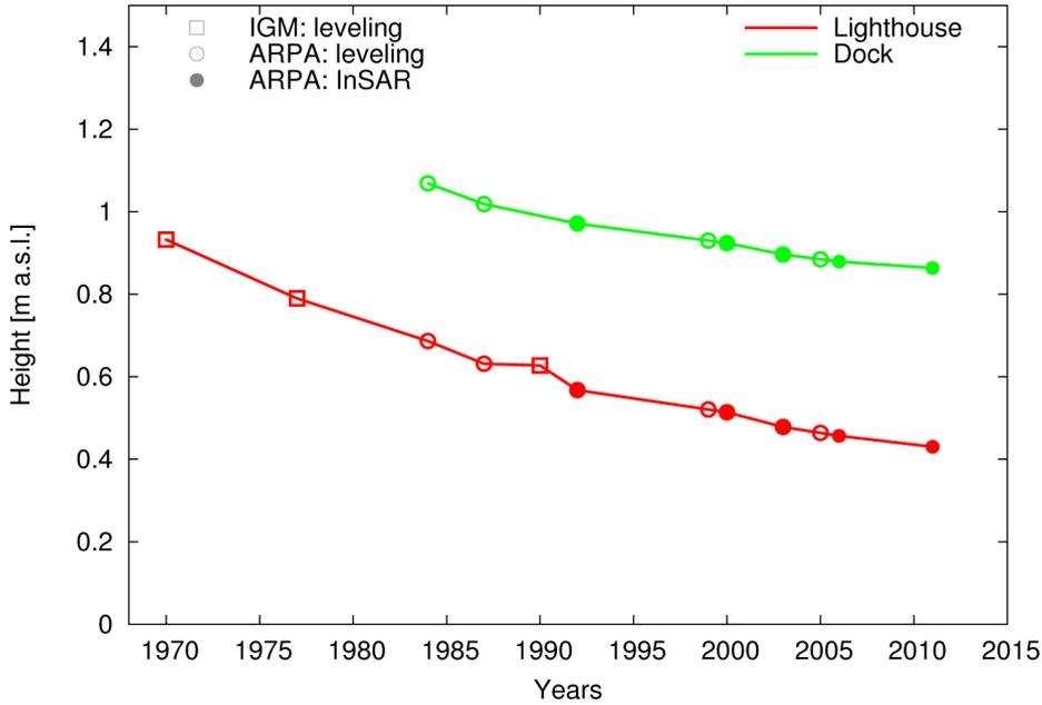
**Figure 6.** Elevation measurements at the Porto Corsini lighthouse (red) and dock (green) benchmarks at various epochs. The various data sources and sampling methods are denoted by different symbols, as indicated in the legend (see Tables 1 and 2 for details).
