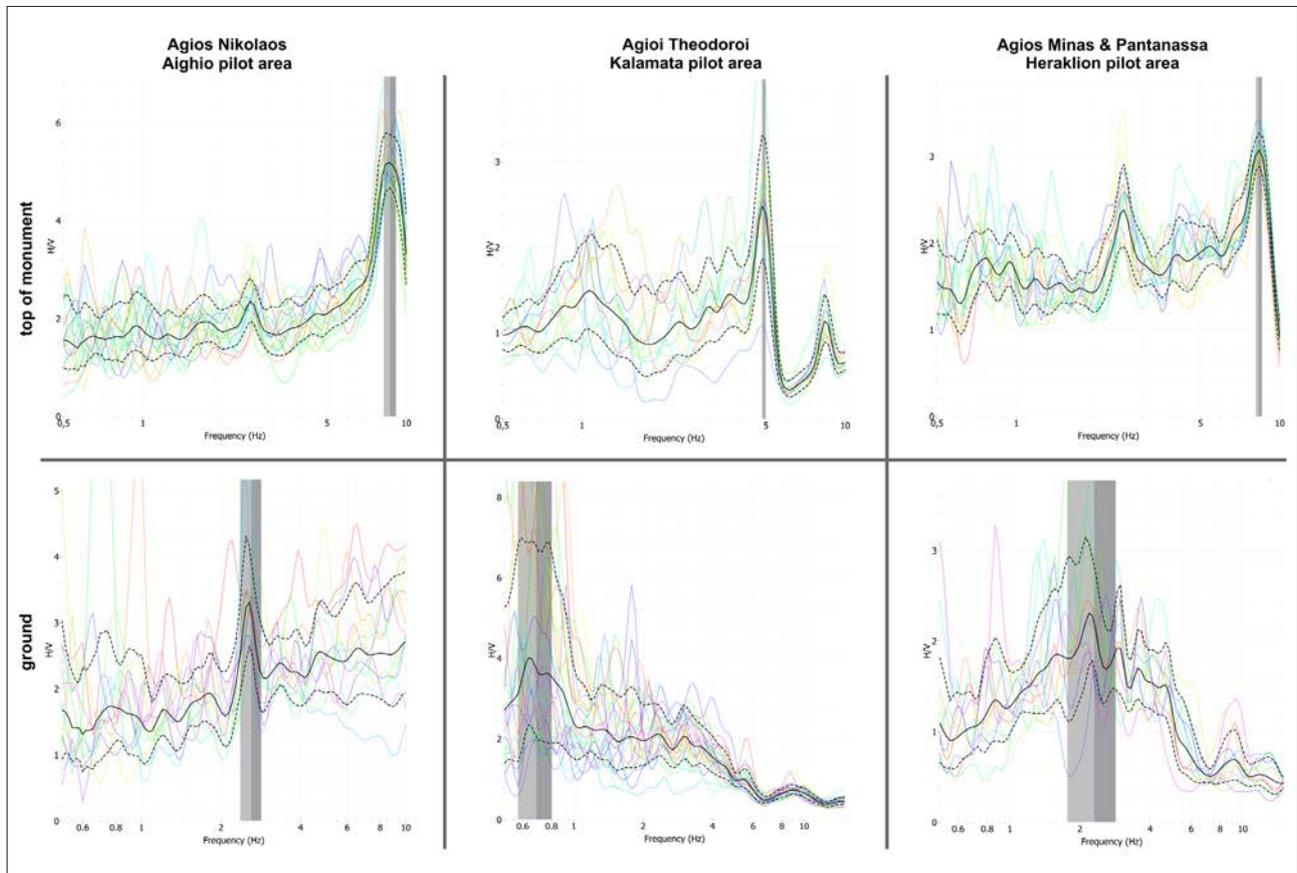
**Figure 6.** H/V spectral ratios resulting from microtremor measurements for the Agios Nikolaos (Aighio pilot area), Agioi Theodoroi (Kalamata pilot area) and Agios Minas and Pantanassa (Heraklion pilot area) monuments (left, central and right column, respectively), on the top of the monuments (top row) and on the ground (bottom row).
