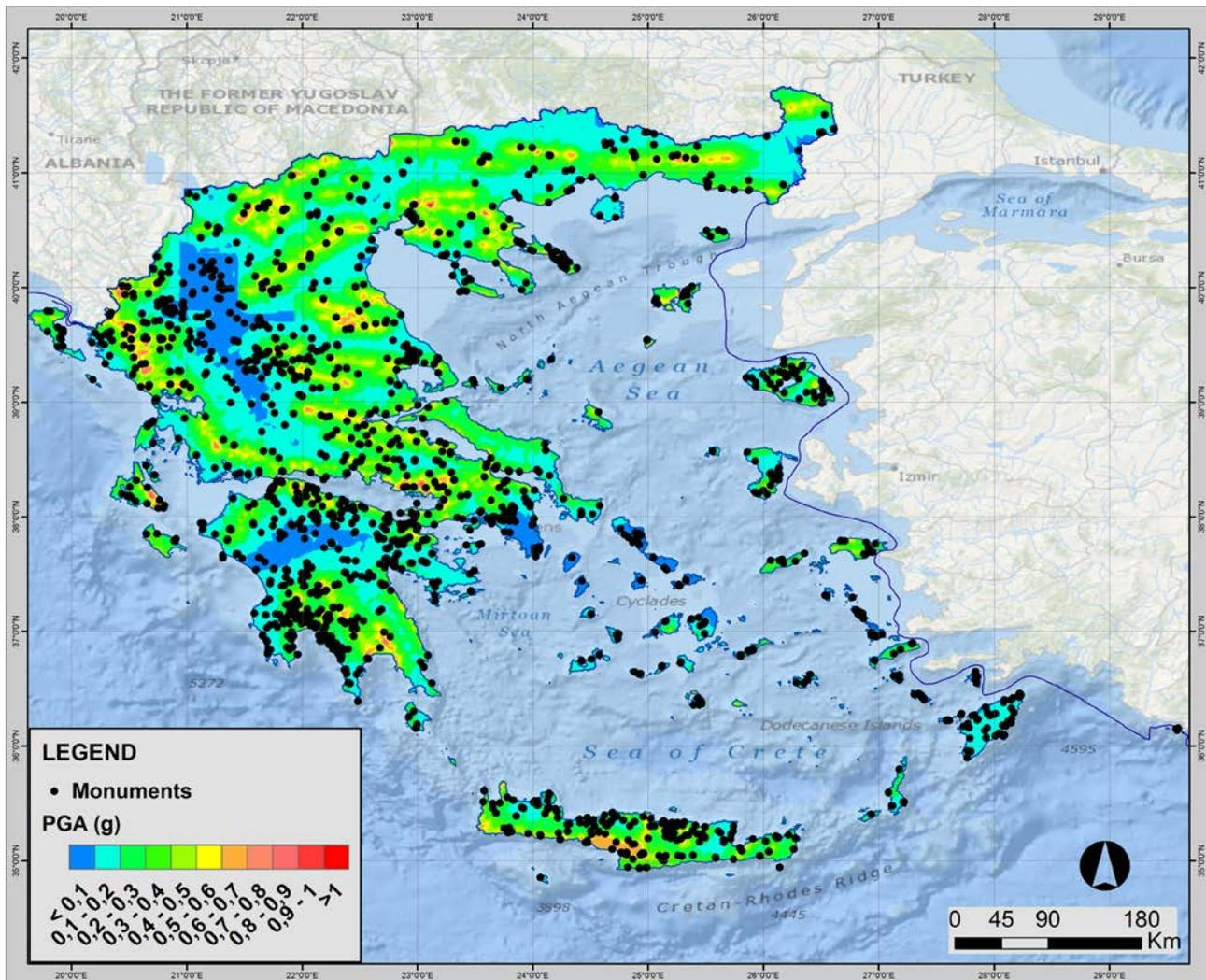
**Figure 2.** Map showing the maximum PGA distribution that was calculated in the scopes of this project. The monuments are also shown as black dots.
