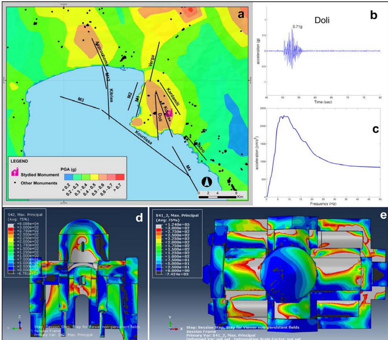
**Figure 9.** Maximum PGA distribution for the Kalamata pilot area that was calculated in the scopes of this project. (b) The calculated synthetic accelerogram at the site of the Agioi Theodoroi monument produced by the Doli seismic source. (c) The calculated spectrum for the same site. (d) and (e) The monument's structure response to ground motion after the hypothetical rupture of Doli seismic source.
