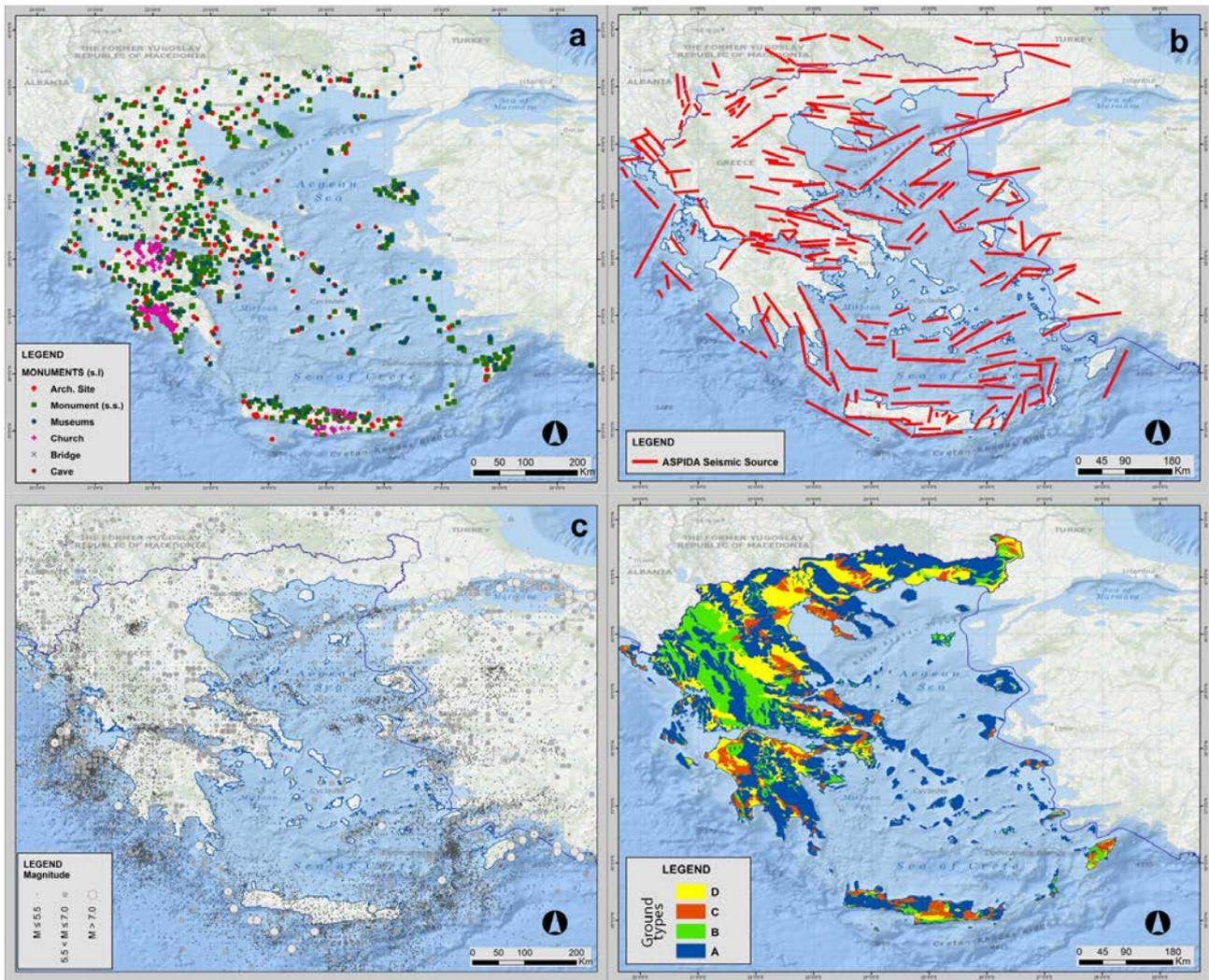
**Figure 1.** The basic datasets of the “ASPIDA” geodatabase: (a) Monuments categorised, (b) seismic sources, (c) combined seismicity from the catalogues of Papazachos et al. [2000], for the period between 550 BC and AD 1963 (included), and NOA, since AD 1964, (d) ground geotechnical characterization.
