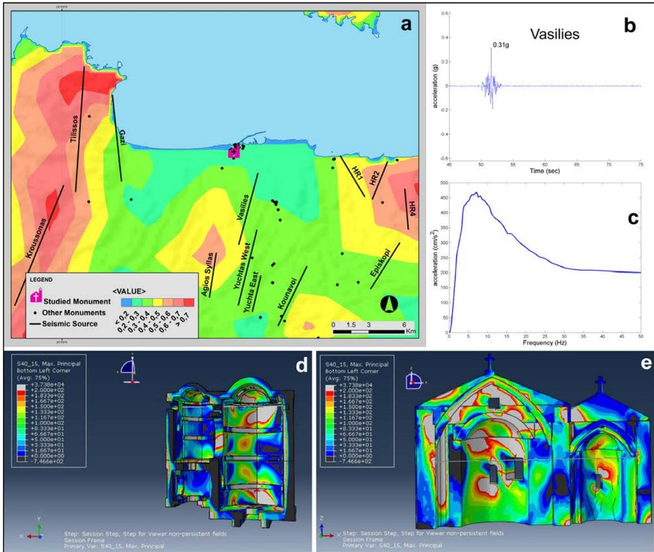
**Figure 10.** Maximum PGA distribution for the Heraklion pilot area that was calculated in the scopes of this project. (b) The calculated synthetic accelerogram at the site of the Agios Minas and Pantanassa monument produced by the Vasilies seismic source. (c) The calculated spectrum for the same site. (d) and (e) The monument's structure response to ground motion after the hypothetical rupture of Vasilies seismic source.
