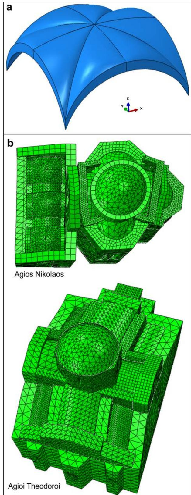
**Figure 7.** (a) Geometry of a modelled Byzantine cross vault. (b) The first predominant eigen mode of the entire models of Agios Nikolaos and Agioi Theodoroi monuments.
