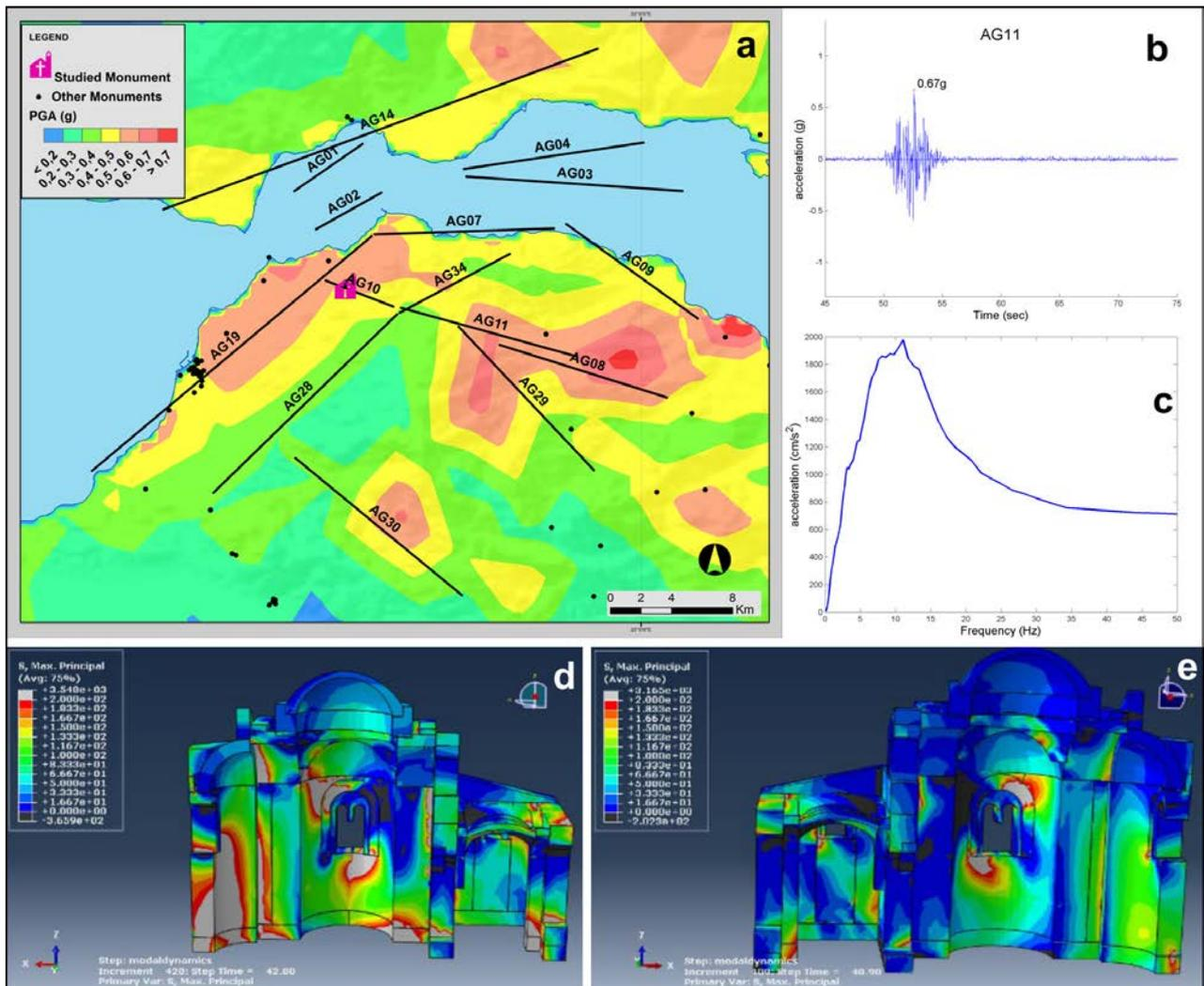
**Figure 8.** (a) Maximum PGA distribution for the Aighio pilot area that was calculated in the scopes of this project. (b) The calculated synthetic accelerogram at the site of the Agios Nikolaos monument produced by the AG11 seismic source. (c) The calculated spectrum for the same site. (d) and (e) The monument's structure response to ground motion after the hypothetical rupture of AG11 seismic source.
