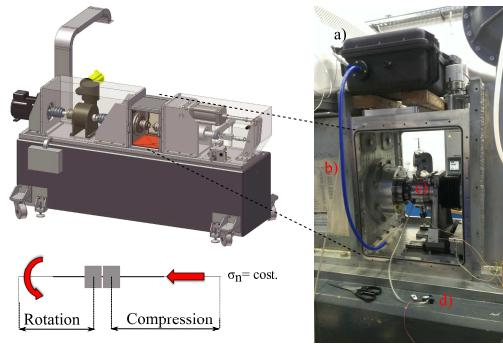
**Figure 2:** The experimental apparatus (SHIVA, on the left modified from [Di Toro et al.(2010)]) essentially made of a rotary axes, a stationary axis and a sample chamber. The experimental assembly consists of the radon detect. (labelled with a), the connection (b) allowing for close loop circulation of fluids from the vessel (c) to the radon detect.; the air pump for air flux (d).
