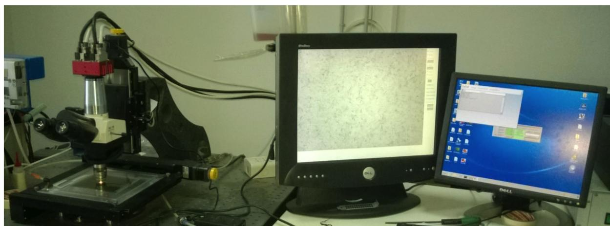
**Figure 4.** The QSS setup. A Cartesian robot with readout head (automatic microscope) is seen on the left. In the centre and right part of the picture, screenshots of the data acquisition program, showing a live image of the emulsion.
