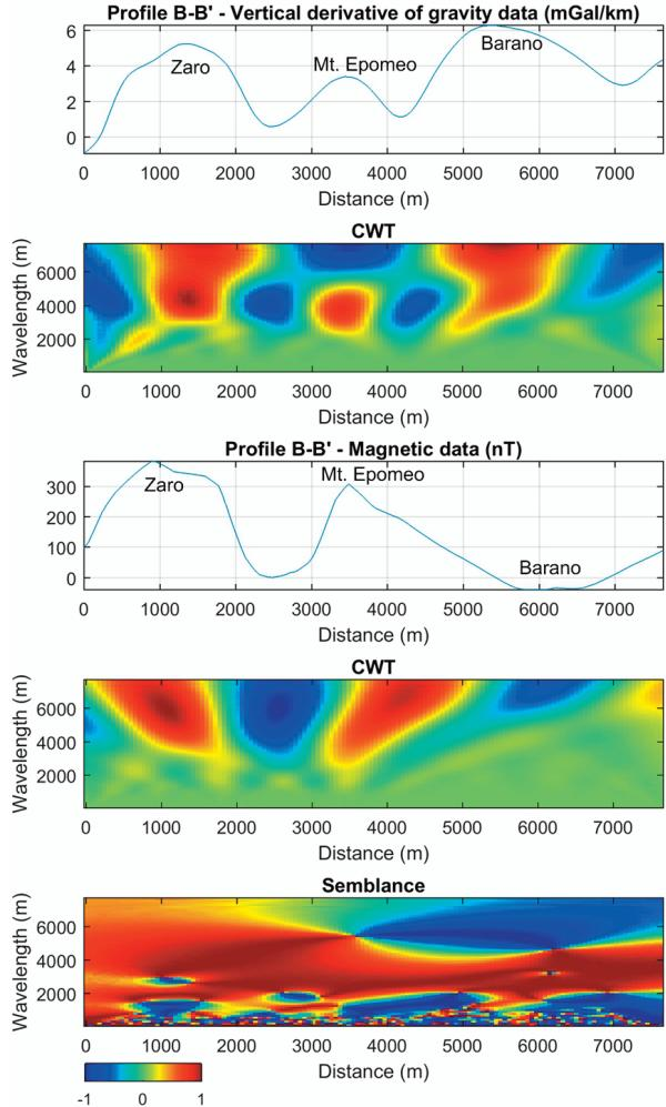
**Figure 6.** The semblance analysis along profile B-B'. a) Gravity data; b) CWT of the gravity data; c) magnetic data; d) CWT of magnetic data; e) semblance function obtained by the processing of the two CWT according to Equation 2.
