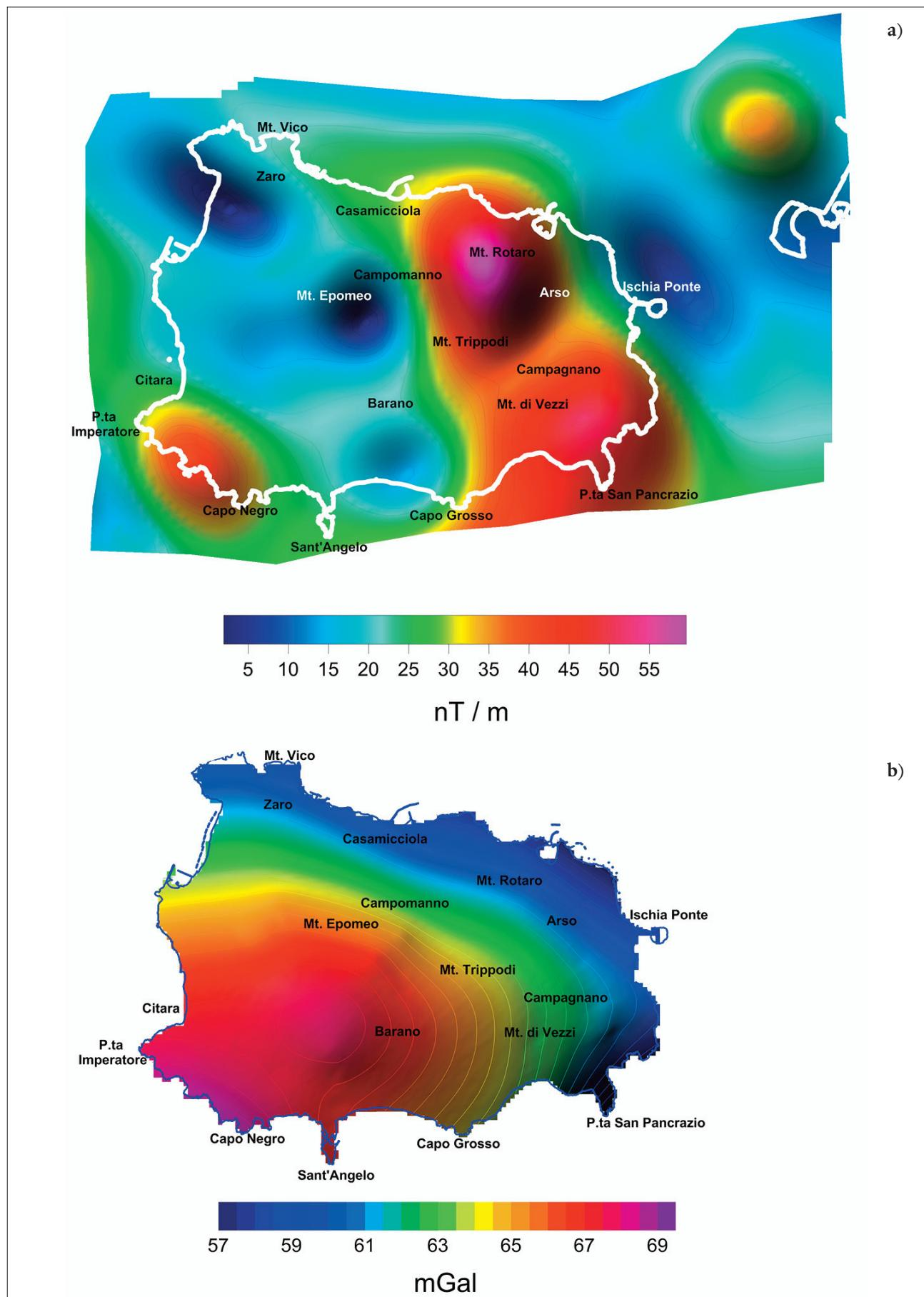
**Figure 10.** Maps of the two datasets after upward continuation at 1500 m a.s.l., highlighting the horizontal position of large scale sources:
