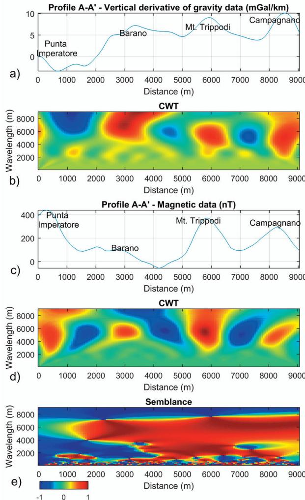
**Figure 5.** Semblance analysis along profile A-A' (see text for details). a) Gravity data; b) CWT of the gravity data; c) magnetic data; d) CWT of magnetic data; e) semblance function obtained by the processing of the two CWT according to Equation 2.
