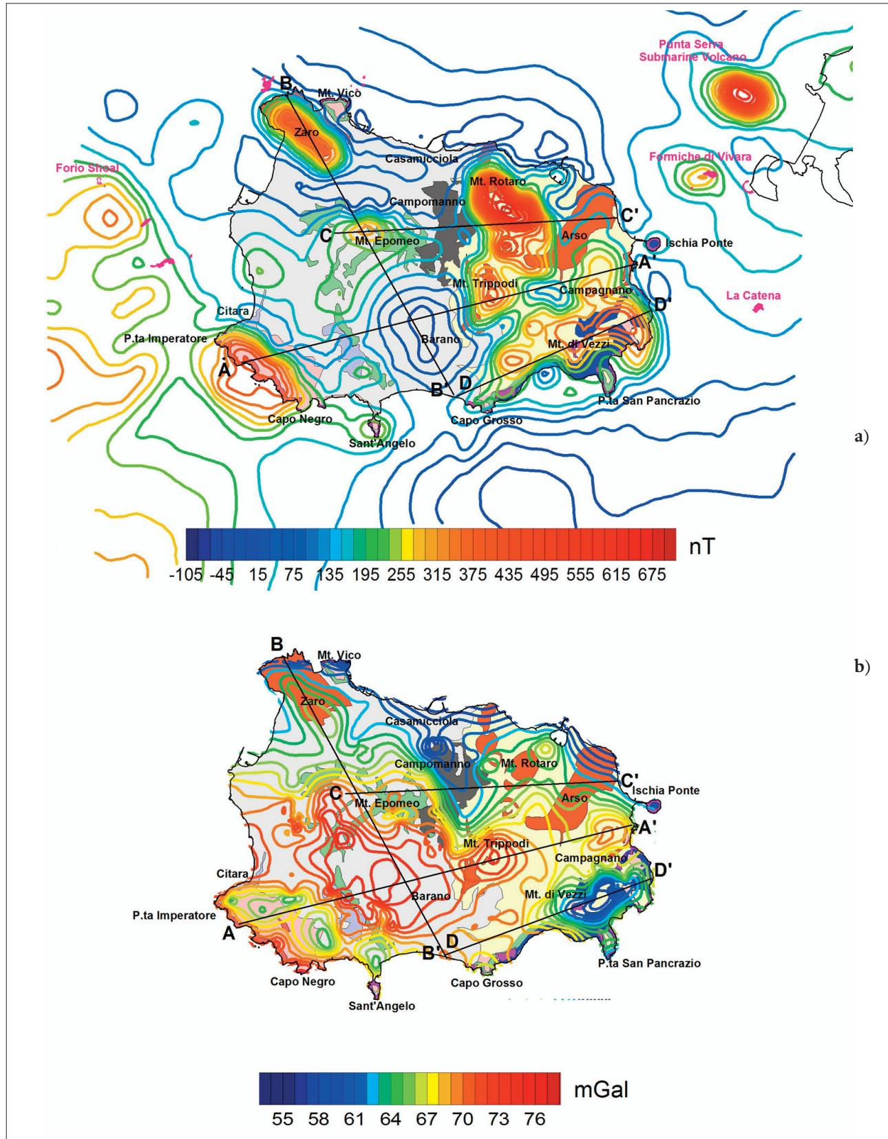
**Figure 4.** Pole-reduced magnetic data (a) and gravimetric data (b) overlaid on a volcanological sketch map of the island (refer to Figure 2a for details). The lines show the location of profiles analyzed in Figs. 5-8.
