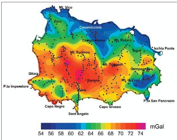
**Figure 3.** Bouguer gravity anomalies of Ischia, including the newly collected in-land gravity stations [Fedi et al. 2011]. Black dots mark the position of the gravity stations.
