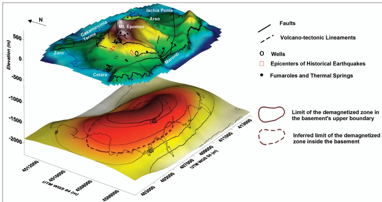
**Figure 11.** Pattern of the Ischia's basement inferred from gravimetric modeling [Nunziata and Rapolla 1987]. Demagnetized areas were identified based on magnetic modeling [Paoletti et al. 2009]. The main faults and volcano-tectonic lineaments area redrawn from Acocella and Funiciello [1999]. Fumaroles, thermal springs and historical earthquakes epicenters are from Manzo et al. [2006], Wells are from Ippolito and Rapolla [1982].
