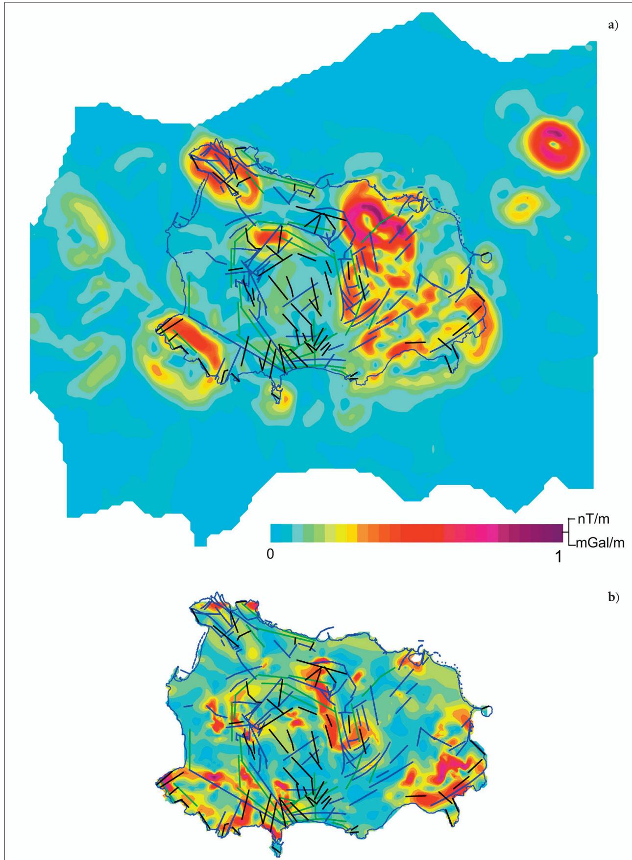
**Figure 9.** Maps of the horizontal gradient of the magnetic and gravity data at Ischia, highlighting the location of magnetic/density lineaments: a) Total horizontal gradient of the pole-reduced aeromagnetic data (M-THG); b) Total horizontal gradient of gravity data (G-THG). The values of the two THG datasets are normalized. Structural lineaments are from: Nappi et al. [2010] (black lines), De Vita et al. [2006] (blue lines), Acocella and Funiciello [1999] (green lines).
