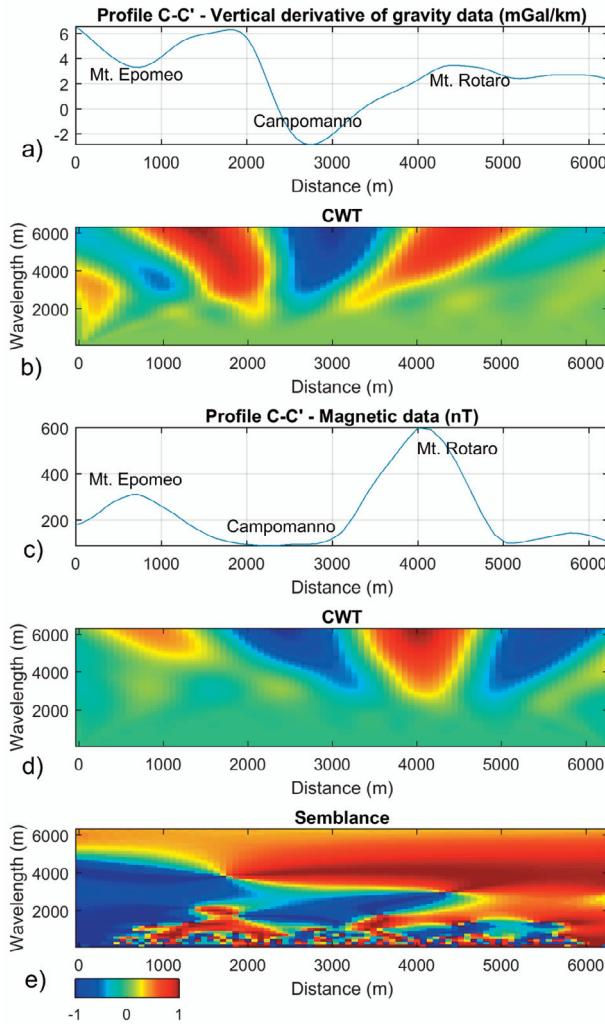
**Figure 7.** The semblance analysis along profile C-C'. a) Gravity data; b) CWT of the gravity data; c) magnetic data; d) CWT of magnetic data; e) semblance function obtained by the processing of the two CWT according to Equation 2.
