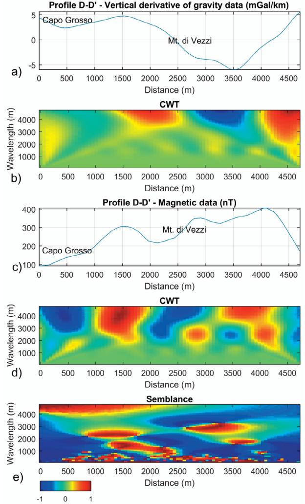
**Figure 8.** The semblance analysis along profile D-D'. a) Gravity data; b) CWT of the gravity data; c) magnetic data; d) CWT of magnetic data; e) semblance function obtained by the processing of the two CWT according to Equation 2.
