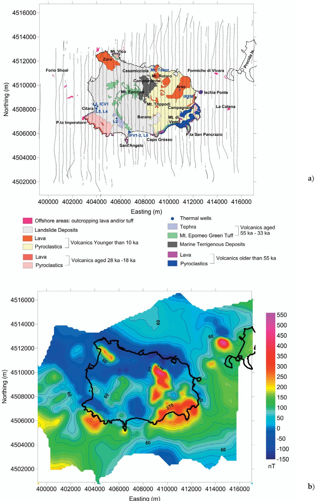
**Figure 2.** a) Helicopter-borne acquisition lines from the October 2005 high-resolution survey overlain to the geologic sketch map of Ischia. The geo-volcanological features of the island are from Vezzoli [1988], de Vita et al. [2006] and Paoletti et al. [2013]. The lava and/or tuff deposits of the offshore areas are from Budillon et al. [2003]. Blue dots show the thermal wells [Ippolito and Rapolla 1982 and references therein]. b) Aeromagnetic data of Ischia and its offshore surroundings.
