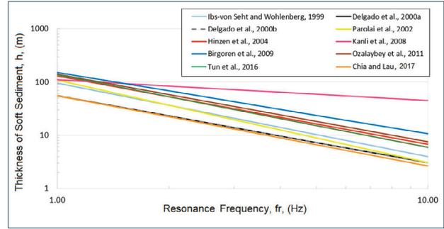
FIGURE 7. Empirical relationships for thickness of soil layer and resonance frequency.
