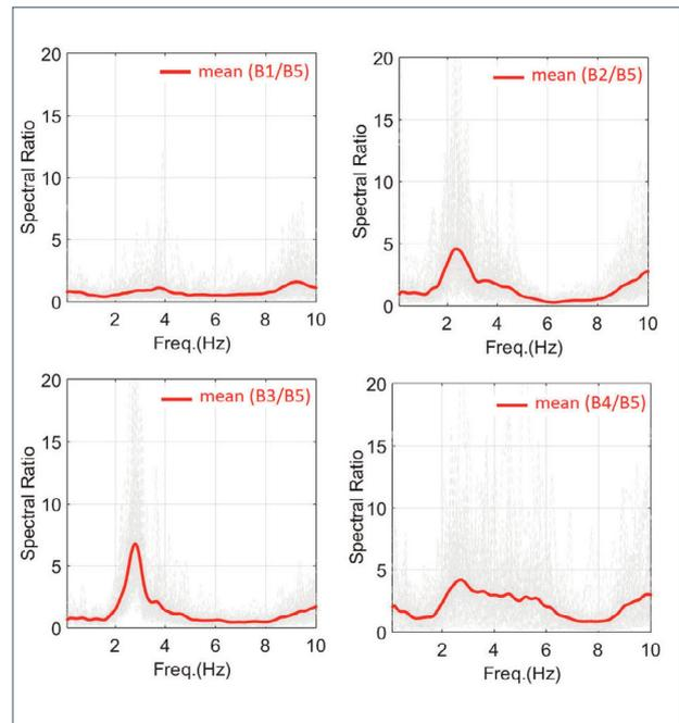
FIGURE 6. Plots of standard spectral ratios vs frequencies (Hz). Red lines represent mean values.
