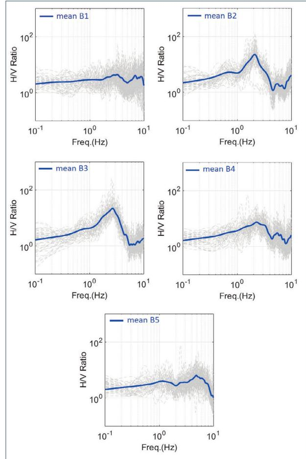
FIGURE 5. Plots of H/V ratios vs frequencies (Hz). Blue lines represent mean values.
