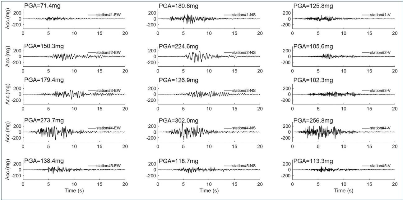
**FIGURE 3.** Time histories of the Mw6.6 Bodrum-Kos earthquake recorded by all B-Net stations. Maximum peak ground acceleration (PGA) value calculated at station#4 (B4=Yali-Ciftlik) is 0.302g.
