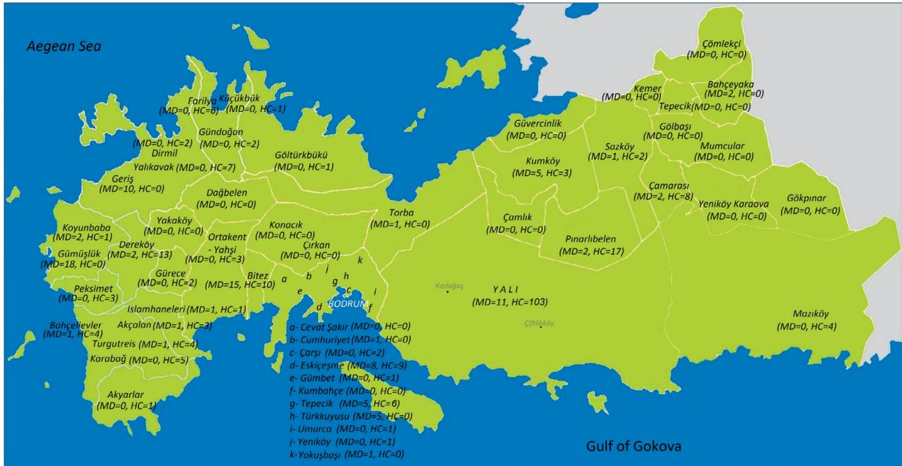
FIGURE 8. Damage distribution in the Bodrum neighborhoods. MD and HC represent *Medium Damage and Heavy Damage and Collapsed* buildings, respectively.
