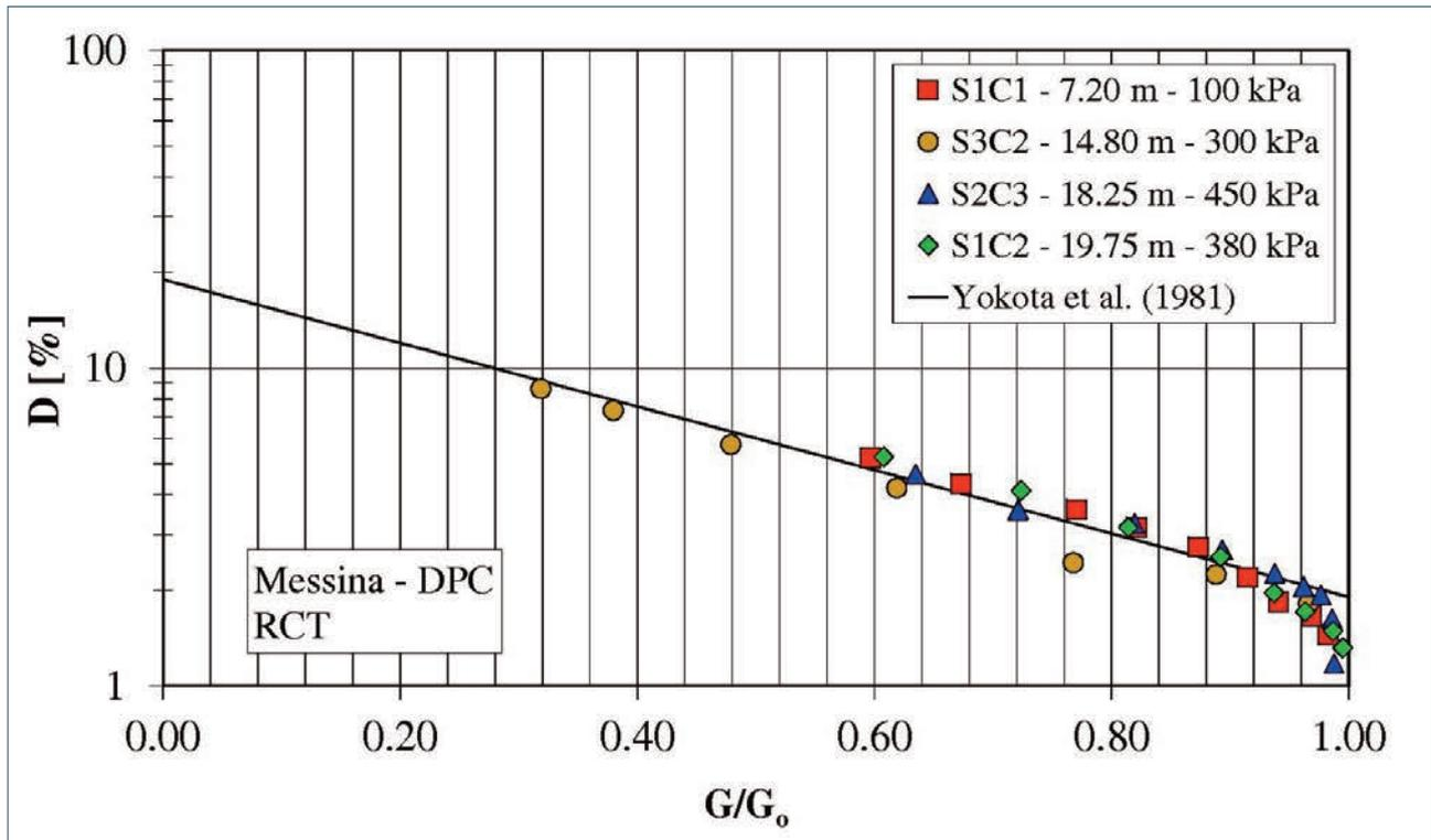
FIGURE 19. D- $G/G_0$  curves from RCT tests.
