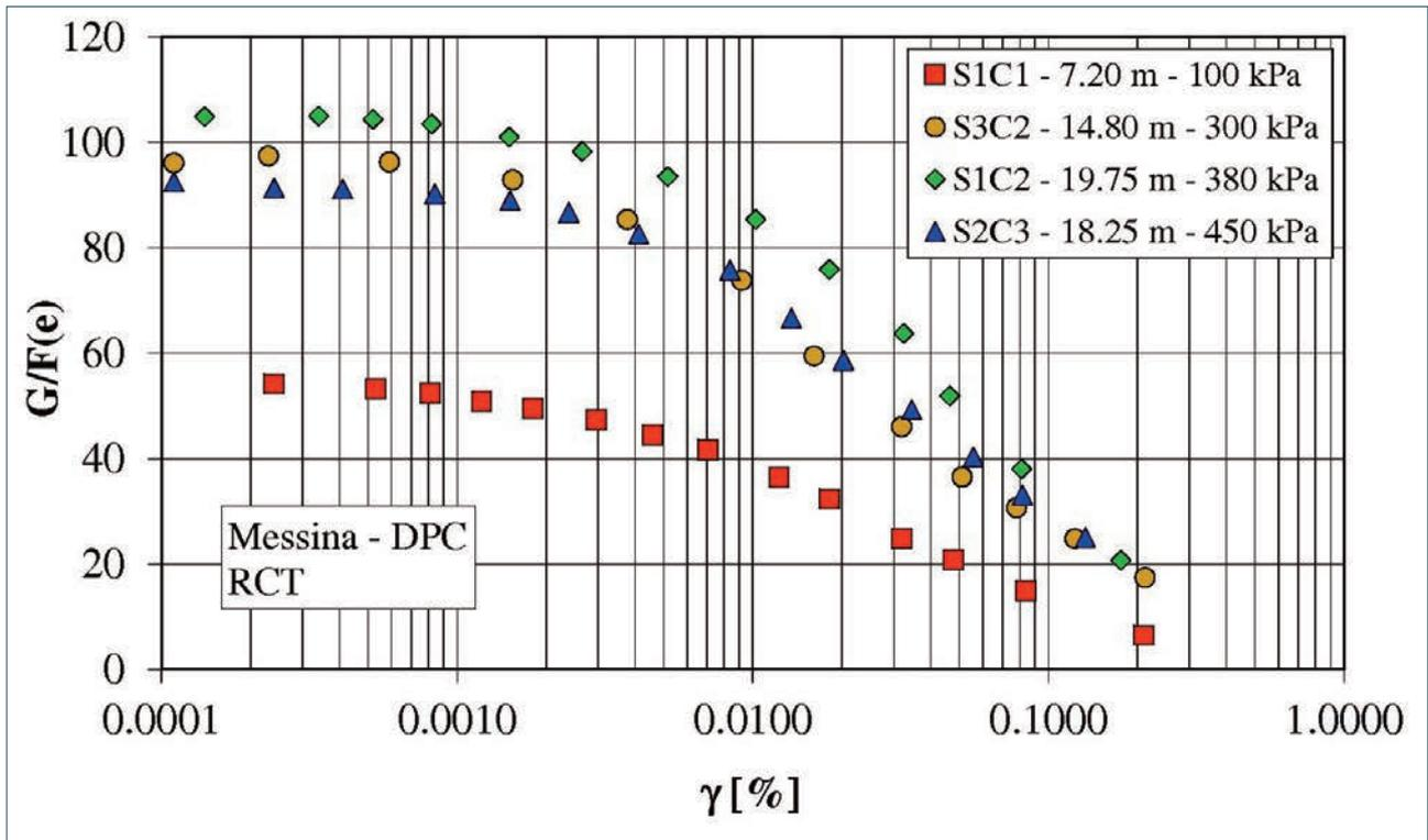
FIGURE 17.  $G/F(e) - \gamma$  curves from RCT tests.
