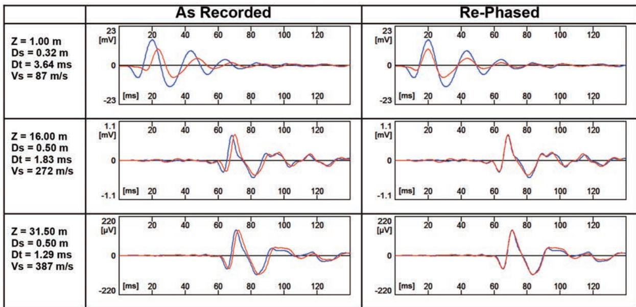
FIGURE 11. Example of seismograms obtained by SDMT at the site of DPC.
