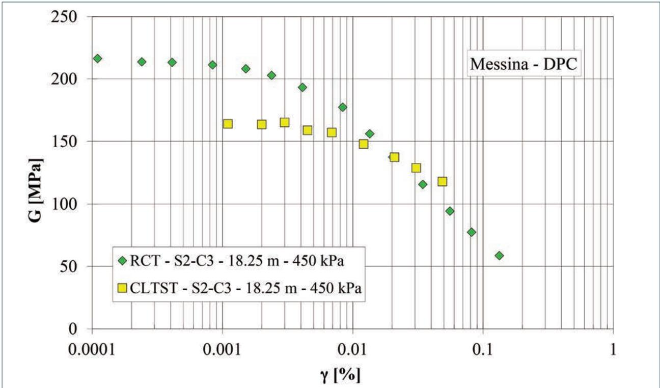
FIGURE 15. G vs γ curves from RCT and CLTST tests.
