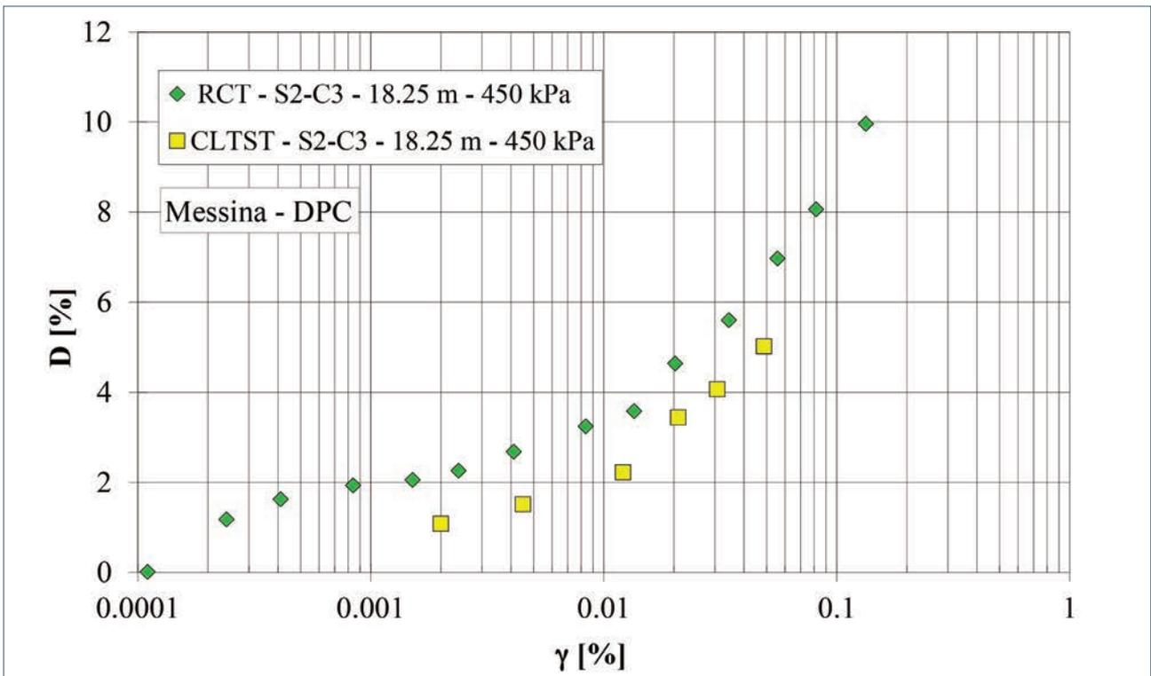
FIGURE 16. D vs γ curves from RCT and CLTST tests.
