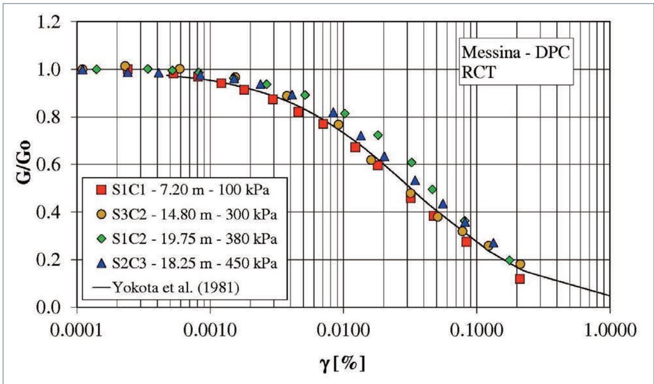
FIGURE 18.  $G/Go - \gamma$  curves from RCT tests.
