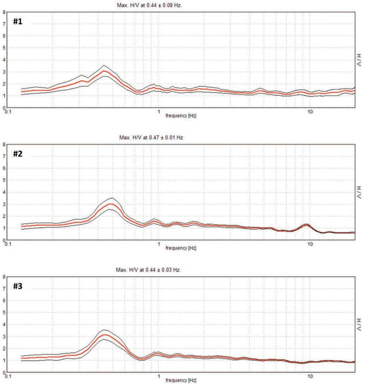
FIGURE S2. HVSR curves for the Faro Superiore area (#11). Red curve = mean spectral ratio, black curves = standard deviation.
