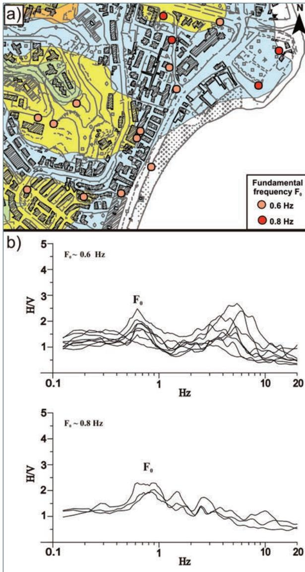
**FIGURE 4.** a) Geological base map of Salvatore dei Greci (SG) showing the location of HVSr measurement points (red and orange dots). For geologic details see Figure 2. b) Examples of different H/V curves obtained in the investigated area. We observed curves characterized by a bimodal behavior with a low  $F_0$  at about 0.6 Hz and peaks at frequencies higher than 3.0 Hz (top plot), and curves with  $F_0$  peaks at about 0.8 Hz (bottom panel).
