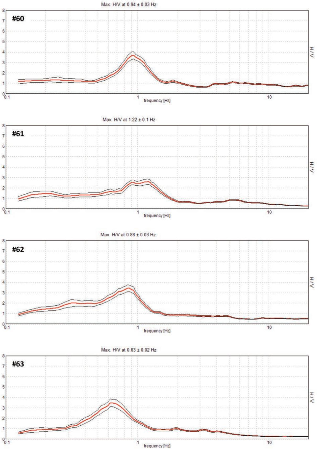
FIGURE S6. HVSR curves for the Historical Center area (#80). Red curve = mean spectral ratio, black curves = standard deviation.
