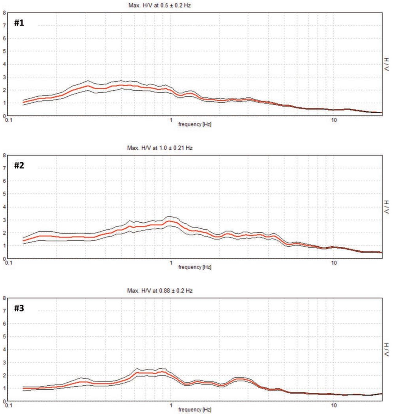
FIGURE S4. HVSR curves for the Salvatore dei Greci area (#16). Red curve = mean spectral ratio, black curves = standard deviation.
