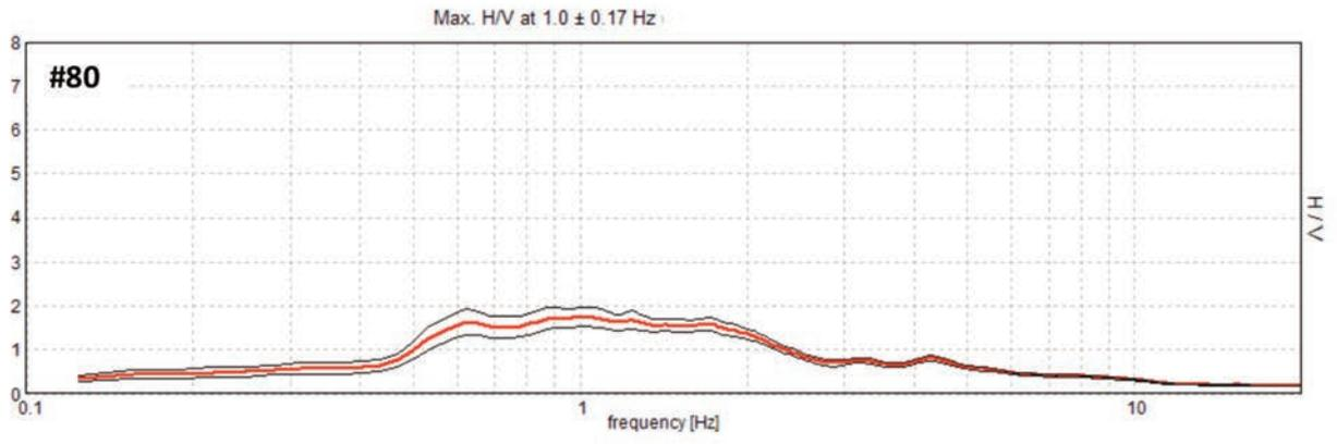
FIGURE S6. HVSR curves for the Historical Center area (#80). Red curve = mean spectral ratio, black curves = standard deviation.
