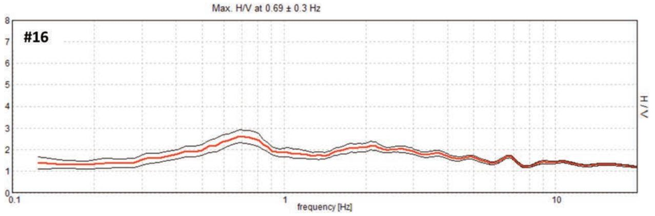
FIGURE S4. HVSR curves for the Salvatore dei Greci area (#16). Red curve = mean spectral ratio, black curves = standard deviation.
