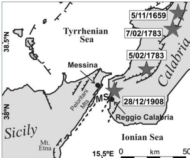
**FIGURE 1.** The figure shows the Messina Straits (MS) area and the principal fault systems: hatched, normal faulting [Ghisetti, 1992; Bonini et al., 2011; Doglioni et al., 2012]. Stars indicate the historical earthquakes for the study area with  $M_w \geq 6.5$  (<http://doi.org/10.6092/INGV.IT-CPT111>).
