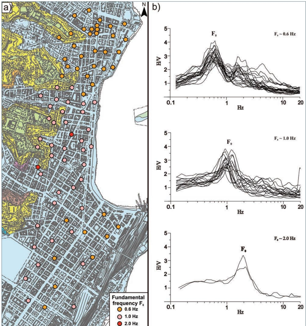
FIGURE 5. a) Geological base map of the Historic Center (HC) showing the location of HVSR measurement points (colored dots). For geologic details see Figure 2. From North to South the sample points exhibit  $F_0$  frequencies in the range 0.6 - 2 Hz. b) Examples of different H/V curves obtained in the investigated area. Plots from top to bottom show curves with peaks at about 0.6 Hz, 1.0 Hz and 2.0 Hz respectively.
