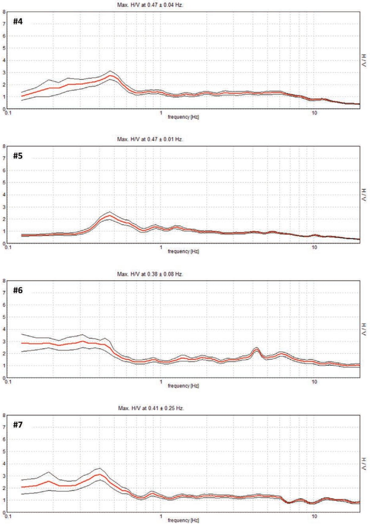
FIGURE S2. HVSR curves for the Faro Superiore area (# 11). Red curve = mean spectral ratio, black curves = standard deviation.
