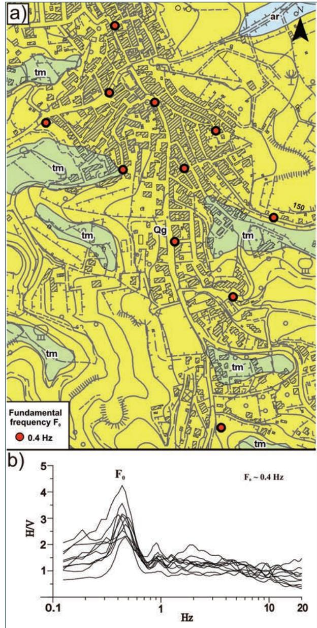
**FIGURE 3.** a) Geological base map of Faro Superiore (FS) showing the location of the seismic noise acquisition points (red dots). For geologic details see Figure 2. b) The panel reports the H/V curves obtained in the FS area. A fundamental frequency peak at about 0.4 Hz is present at all investigated sites.
