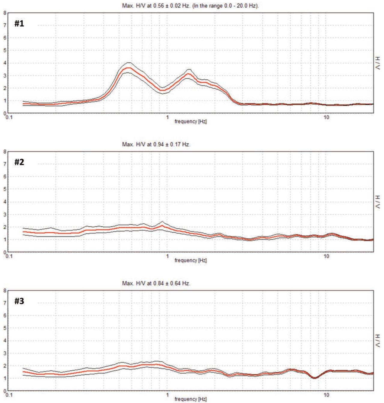
FIGURE S8. HVSR curves for the Monumental Cemetery area (#60). Red curve = mean spectral ratio, black curves = standard deviation.
