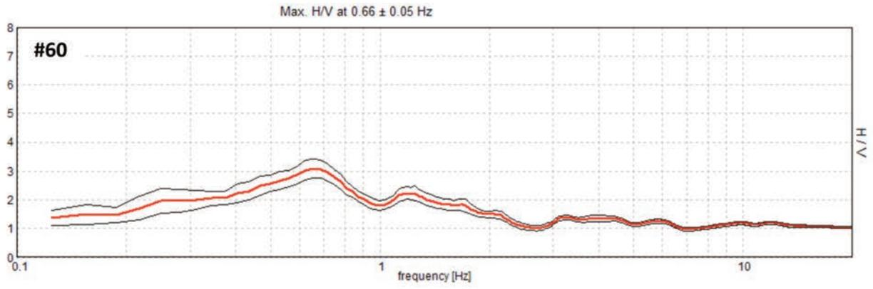
FIGURE S8. HVSR curves for the Monumental Cemetery area (#60). Red curve = mean spectral ratio, black curves = standard deviation.
