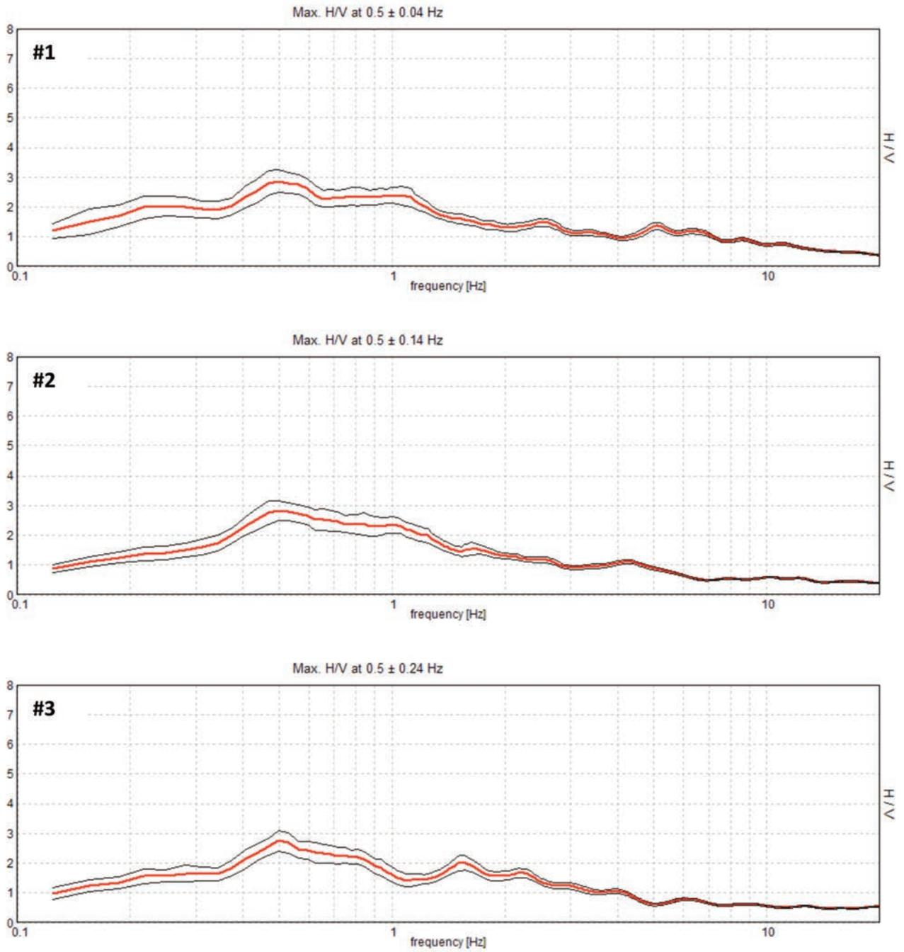
FIGURE S6. HVSR curves for the Historical Center area (#80). Red curve = mean spectral ratio, black curves = standard deviation.
