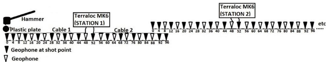
Figure 5. Roll-along technique during seismic refraction survey.
