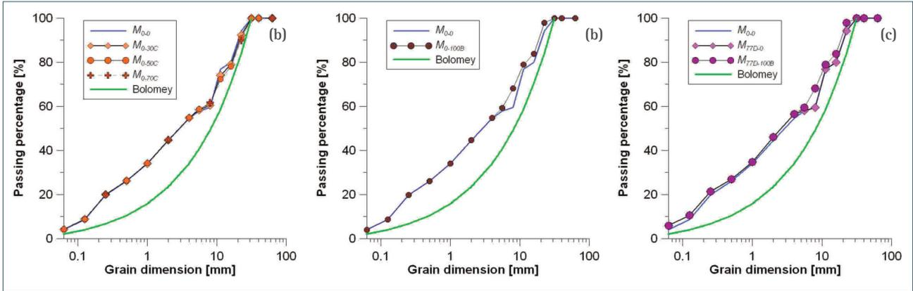
FIGURE 3. Comparison between the Bolomey optimal grain size distribution curve and the real grain size distribution in the mix design. (a) Mixtures  $M_{0-0}$ ,  $M_{0-30C}$ ,  $M_{0-50C}$ ,  $M_{0-70C}$ ; (b) Mixtures  $M_{0-0}$ ,  $M_{0-100B}$ ; (c) Mixtures  $M_{0-0}$ ,  $M_{77D-0}$ ,  $M_{77D-100B}$ .
