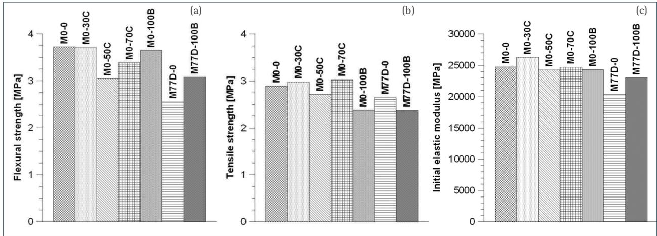
FIGURE 8. (a) Concrete flexural strength  $\sigma_f$ . (b) Concrete uniaxial tensile strength  $\sigma_t$ . (c) Concrete initial elasticity modulus.
