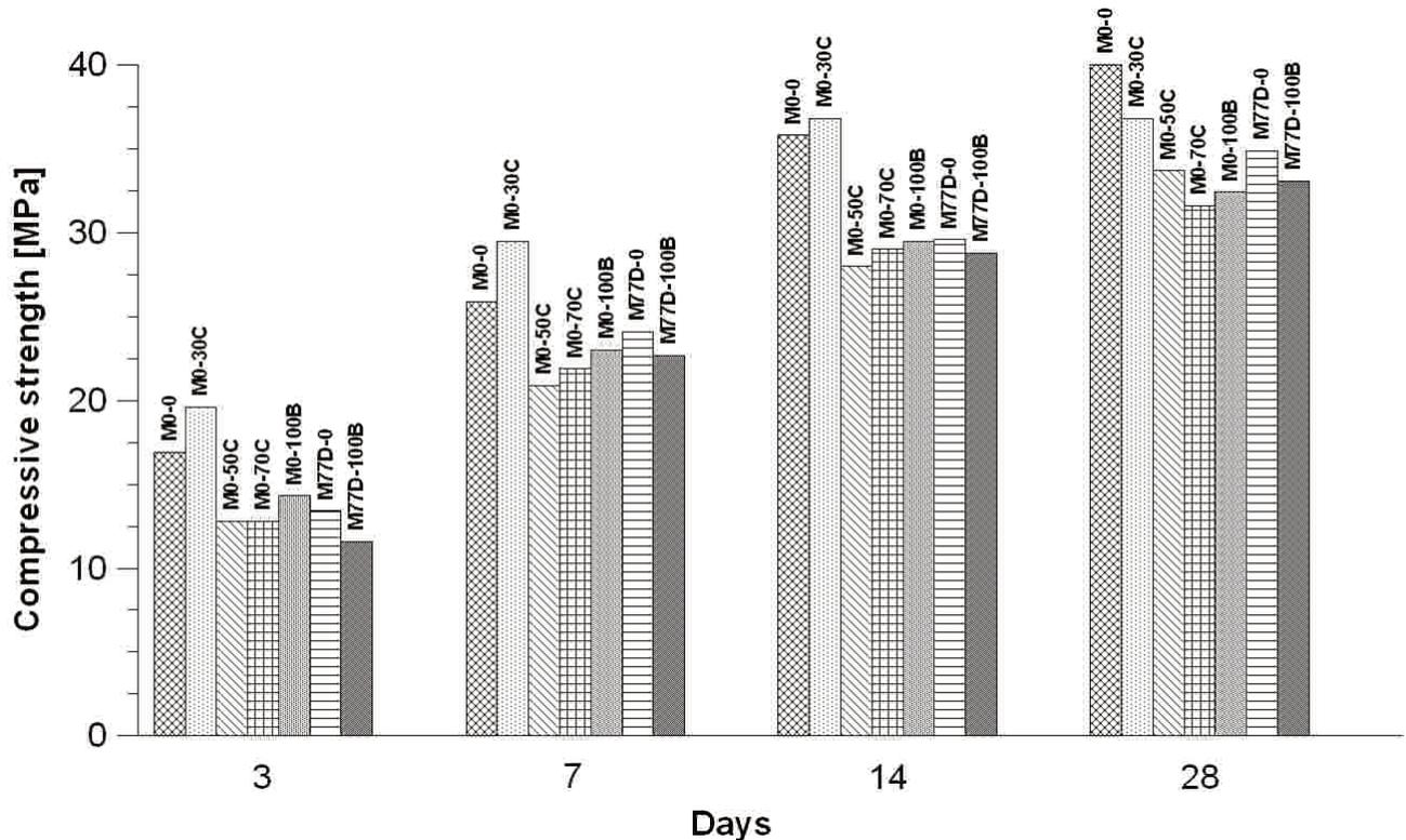
FIGURE 6. Concrete uniaxial compression strength.
