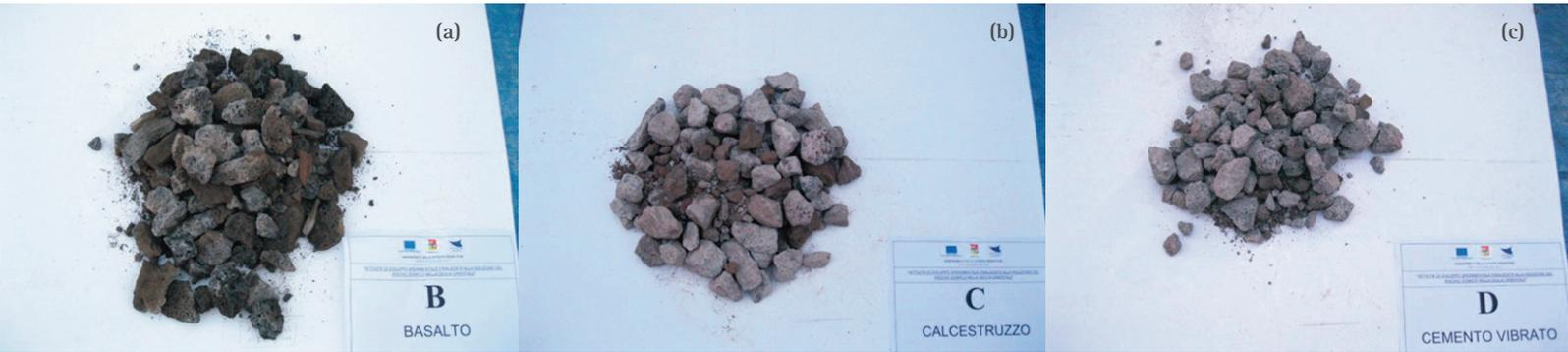
FIGURE 1. (a) Recycled basalt aggregate (B). (b) Recycled structural concrete aggregate (C). (c) Recycled vibrated concrete blocks aggregate (D).
