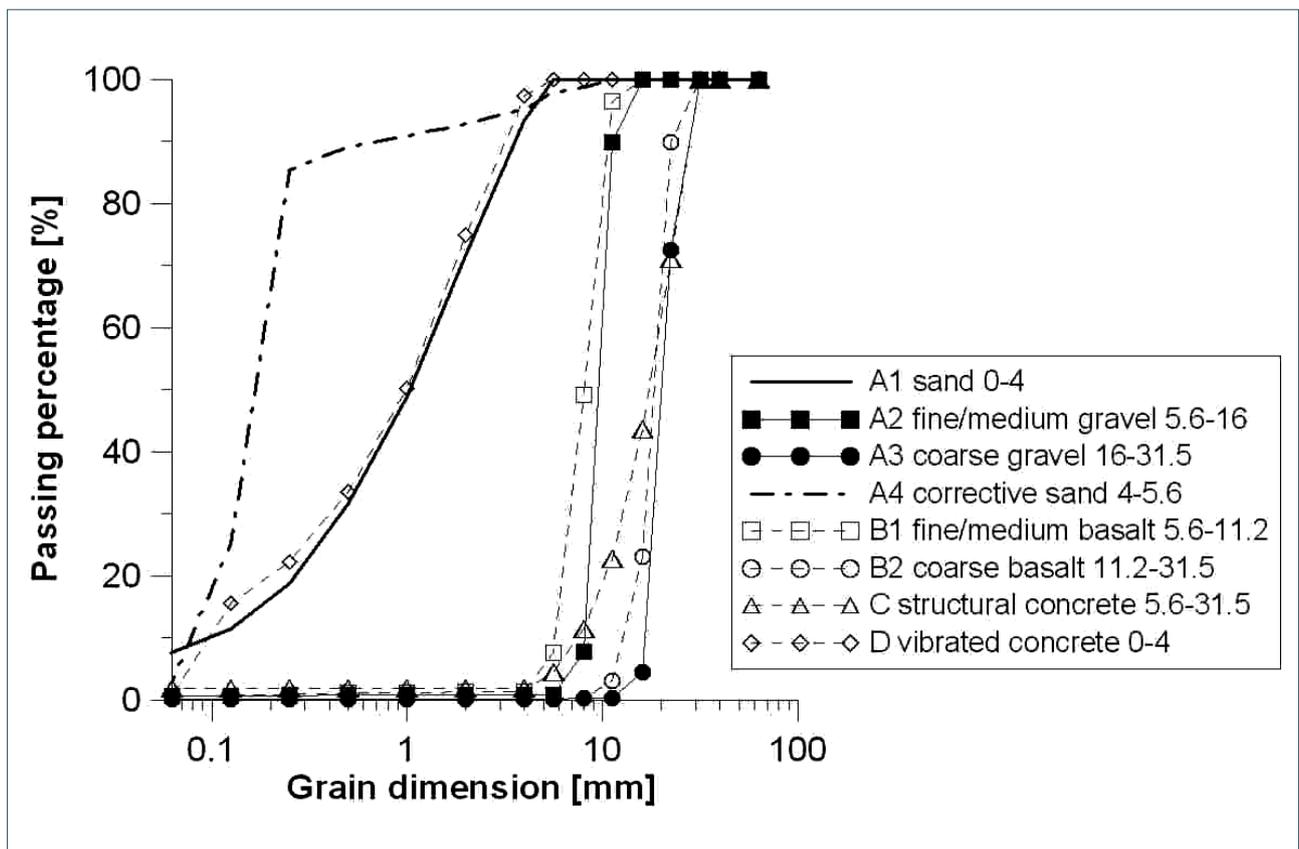
FIGURE 2. Particle size distribution curve.
