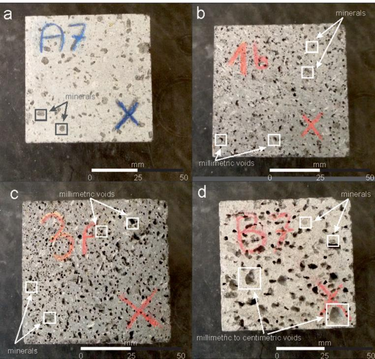
**FIGURE 7** Etna basalt. (a) Class I: massive specimens with no visible vesicles. (b), (c) class II: vesicular specimens with millimetric voids; (d) Class III: vesicular specimens with millimetric to centimetric voids. From Pappalardo and Mineo [Pappalardo and Mineo, 2016].
