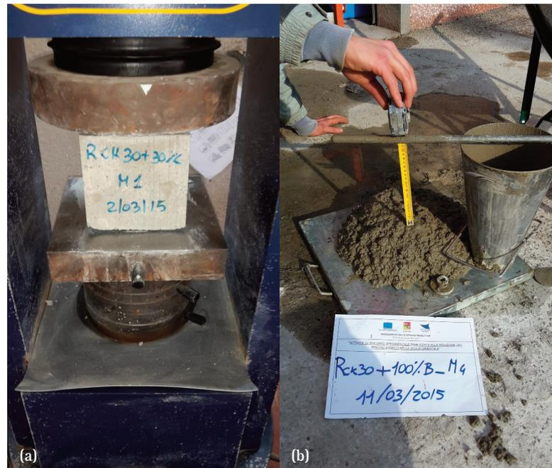
FIGURE 4. (a) Concrete mix  $M_{0-100B}$ : Monotonic uniaxial test for the measure of the compressive strength  $\sigma_c$ . (b)  $M_{0-100B}$  mixture -Slump test.
