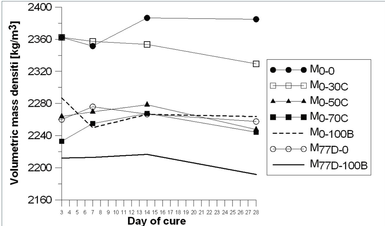
FIGURE 5. Density of fresh and hardened concrete.
