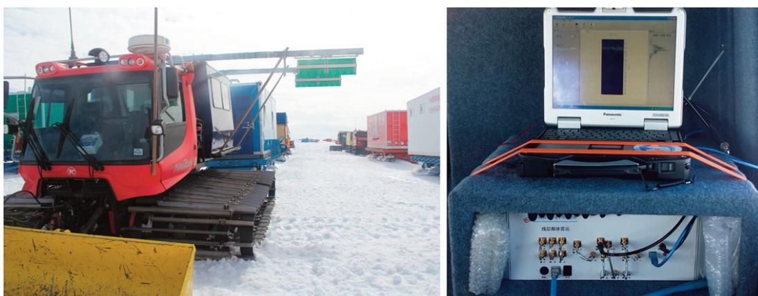
**Figure 2.** Sounding radar system and antenna arrangements on the snowmobile.
