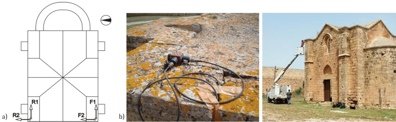
FIGURE 9. Dynamic identification. (a) One of the test setups showing the position of the reference ( $R$ ) and free ( $F$ ) accelerometers; and (b) views of the dynamic measurements.
