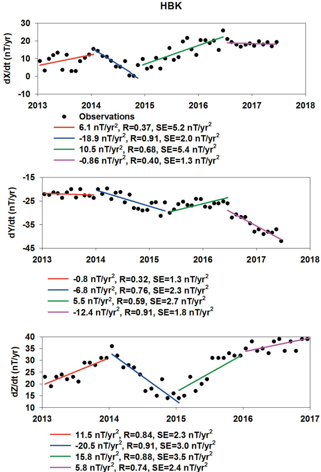
**Figure 2.** Secular variation of the X, Y and Z components at HBK between 2013.0 and 2017.5 as derived from monthly-mean values. The black dots show monthly mean secular variation estimates derived from 12-month differences, while piecewise linear fits to the data provide estimates of secular acceleration as given in the respective legends. The quality of each fit can be estimated by the respective regression coefficients R, while Standard Errors (SE) are also included.
