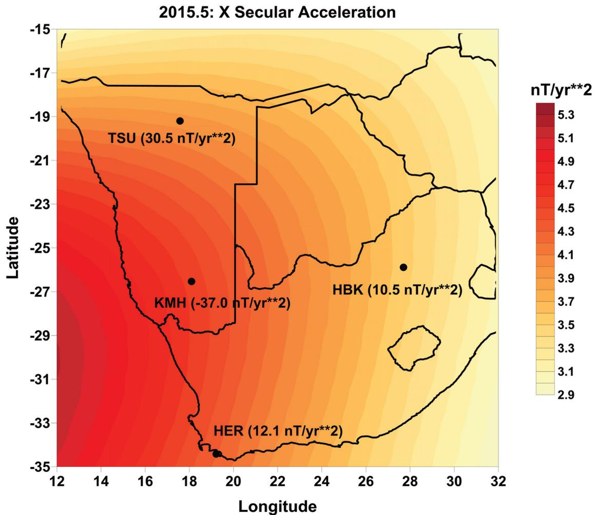
**Figure 5.** A map showing X-component secular acceleration at the Earth’s surface at 2015.5 in the southern African region as determined using the CHAOS6-x7 model. The positions of the different observatories used in the investigation are indicated by their respective IAGA codes and black dots. Values for SA determined from experimental observations at 2015.5 are included for each observatory to serve as reference.
