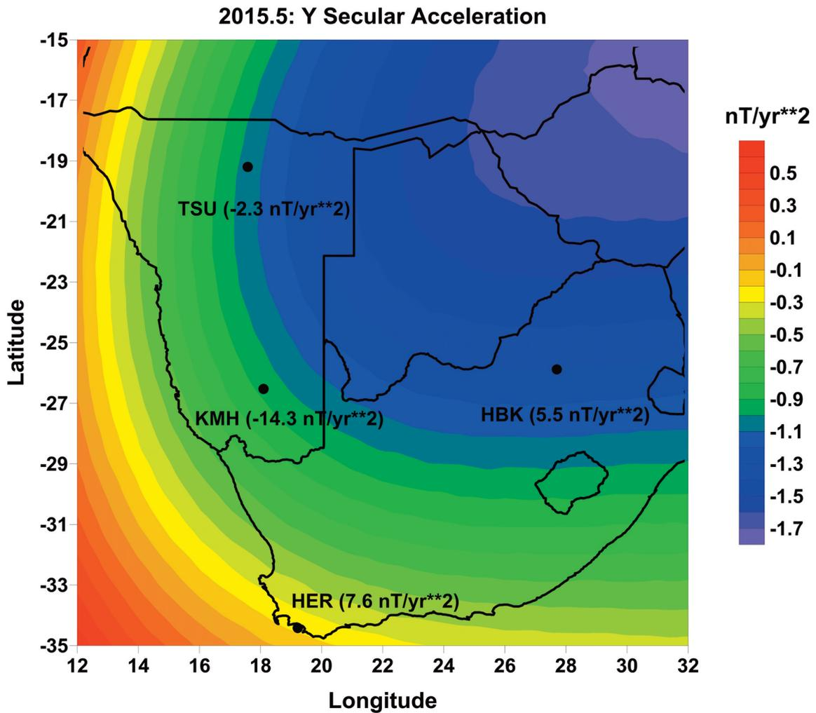
**Figure 6.** A map showing Y-component secular acceleration at the Earth’s surface at 2015.0 in Southern Africa using the CHAOS6-x7 model. The positions of the different observatories used in the investigation are indicated by their respective IAGA codes and black dots. Values for SA determined from experimental observations at 2015.5 are included for each observatory to serve as reference.
