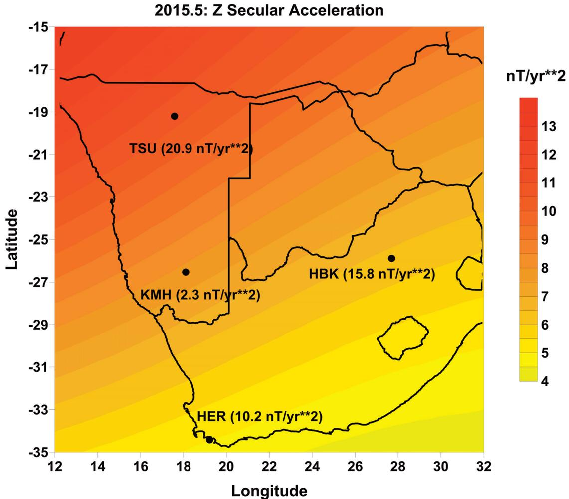
**Figure 7.** CHAOS6-x7 geomagnetic field model estimates of Z component secular acceleration across Southern Africa for 2015.0. The respective magnetic observatories used in this study are indicated by black dots and their IAGA codes. Values for SA determined from experimental observations at 2015.5 are included for each observatory to serve as reference.
