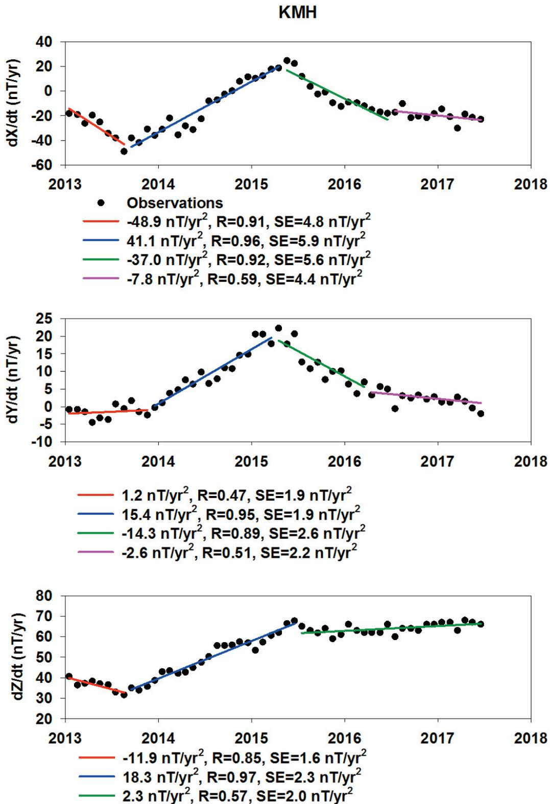
**Figure 3.** Secular variation of the X, Y and Z components at KMH between 2013.0 and 2017.5. The black dots show monthly mean secular variation estimates from 12-month differences, while automatically fitted piecewise linear fits to the data provide estimates of secular acceleration as given in the respective legends. Regression coefficients R provide an estimate of the quality for every fit, together with Standard Errors (SE).
