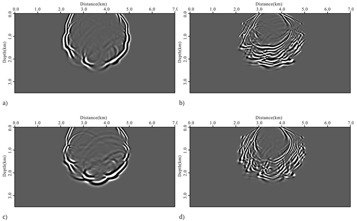
**Figure 11.** Snapshots corresponding to the horizontal component of the P-wave (a), the vertical component of the P-wave (b), the horizontal component of the S-wave (c) and the vertical component of the S-wave (d) at 0.8 s with the 6th-order ESGLFD method. The model used for elastic wave simulation is the subset, denoted by the dashed rectangle, of the resampled elastic Marmousi2, shown in Figure 9.
