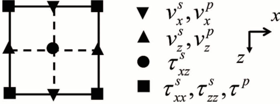
Figure 1. A schematic of a 2D staggered grid scheme.
