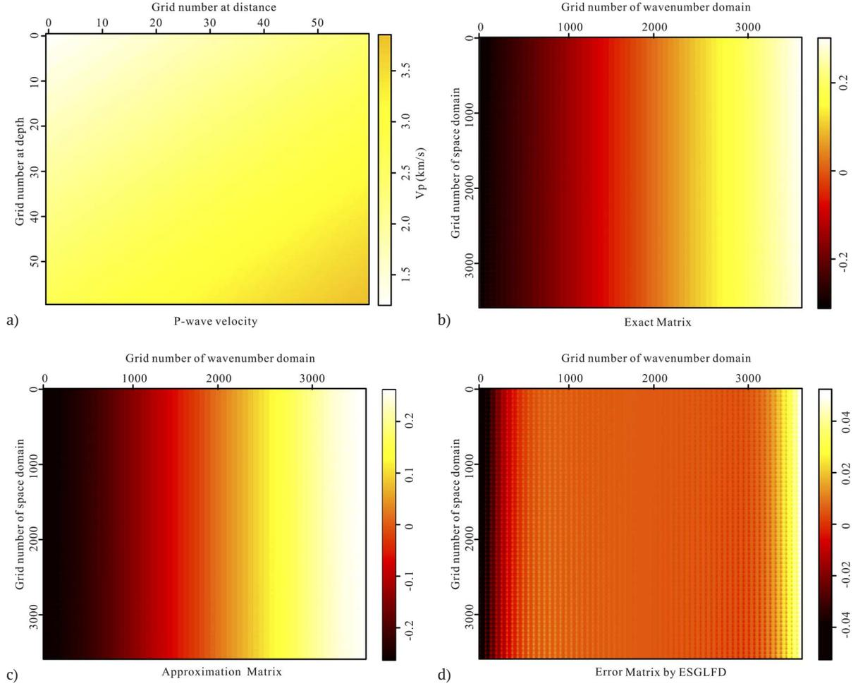
**Figure 2.** (a) A linearly increasing P-wave velocity model, (b) An exact matrix for  $\partial_p / \partial_{x_j^*}$  with the k-space method, (c) An approximation matrix for  $\partial_p / \partial_{x_j^*}$  with the ESGLFD method, (d) The absolute error between the exact matrix and the approximate matrix.
