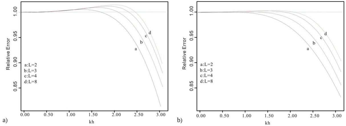
**Figure 3.** 2D dispersion curves of the FD methods (a) and the ESGLFD methods (b) for different orders, fourth-order ( $L = 2$ , blue), six-order ( $L = 3$ , red), eight-order ( $L = 4$ , purple), sixteen-order ( $L = 8$ , green),  $v = 3000\text{m/s}$ ,  $Dt = 1\text{ms}$  and  $\theta = \pi/8$ .
