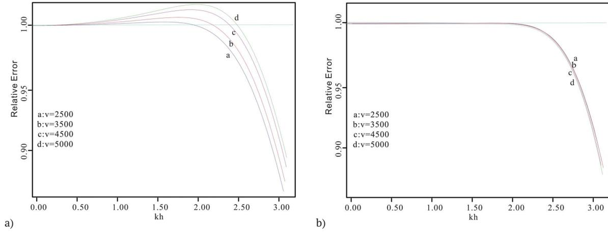
**Figure 4.** 2D dispersion curves of the FD methods (a) and the ESLFD methods (b) for different velocities,  $v = 2500$  m/s (blue),  $v = 3500$  m/s (red),  $v = 4500$  m/s (purple),  $v = 5000$  m/s (green),  $L = 6$ ,  $Dt = 1$  ms and  $\theta = \pi/8$ .
