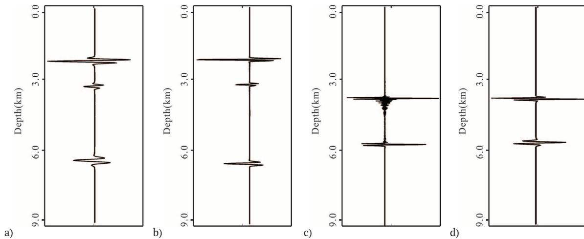
**Figure 9.** Vertical slices extracted from the  $x$ -component snapshots (a) related to P-wave by the SGFD method, (b) related to P-wave by the ESGLFD method, (c) related to S-wave by the SGFD method, and (d) related to S-wave by the ESGLFD method at the distance of 3.0 km.
