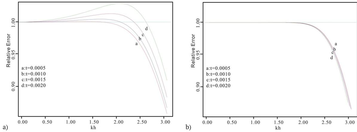
**Figure 5.** 2D dispersion curves of the FD methods (a) and the ESLFD methods (b) for different time intervals,  $Dt = 0.5$  ms (red),  $Dt = 1.0$  ms (blue),  $Dt = 1.5$  ms (purple),  $Dt = 2.0$  ms (green),  $v = 3000$  m/s,  $L = 6$  and  $\theta = \pi/8$ .
