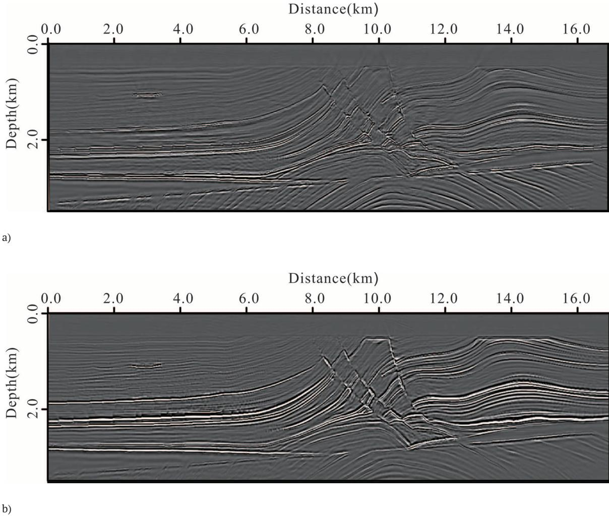
**Figure 13.** The stacked PP image component (a), the stacked PS image component (b).
