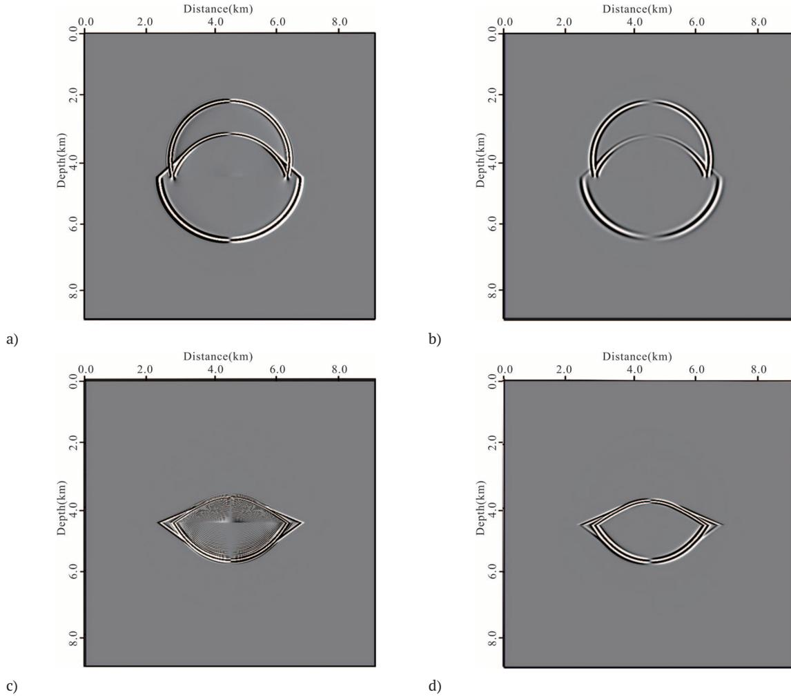
**Figure 8.** Elastic wavefield snapshots at  $t=0.8$ s of a two-layer model by using the 4th-order SGFD method and the 4th-order ESGLFD method: (a) the  $x$ -component snapshot of the P-wave by the SGFD method; (b) the  $x$ -component snapshot of the P-wave by the ESGLFD method; (c) the  $x$ -component snapshot of the S-wave by the SGFD method; (d) the  $x$ -component snapshot of the S-wave by the ESGLFD method. Head waves are highlighted by the red arrows.
