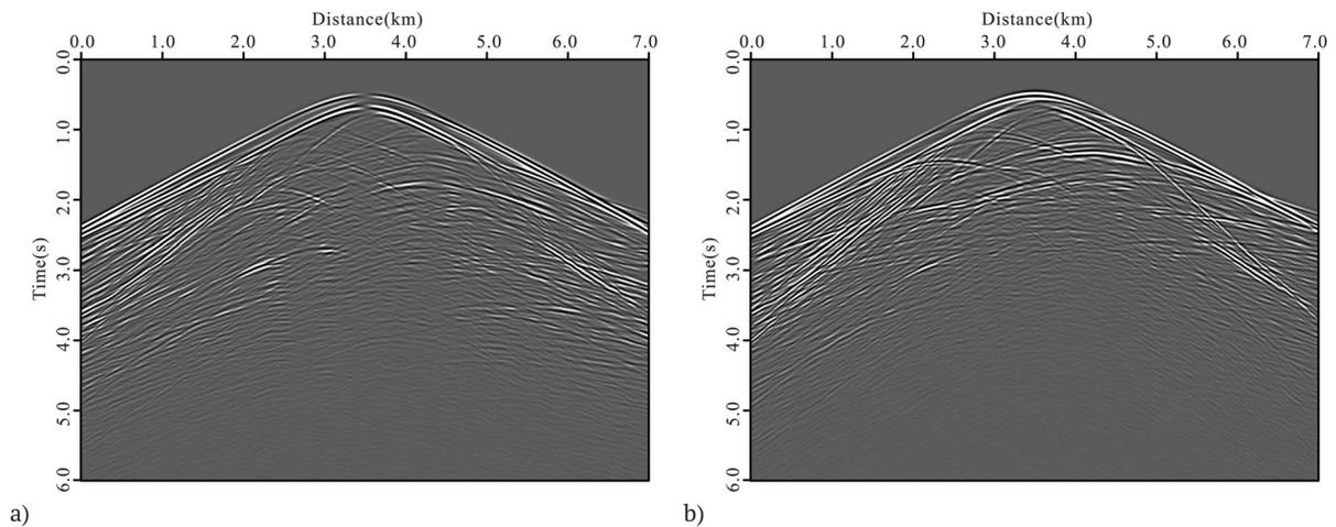
**Figure 12.** Elastic common-source gathers corresponding to the horizontal component (a) and the vertical component (b).
