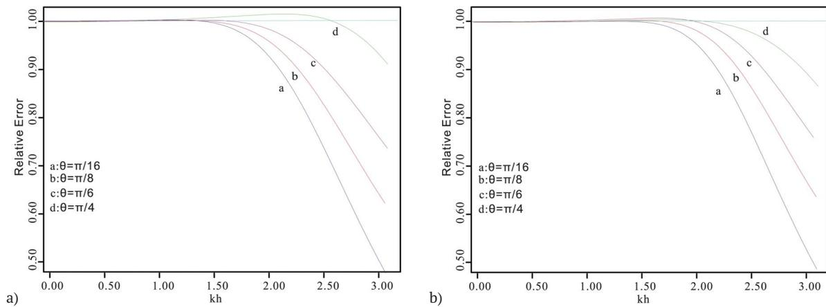
**Figure 6.** 2D dispersion curves of the FD methods (a) and the ESLFD methods (b) for different propagation angles,  $\theta = \pi/16$  (blue),  $\theta = \pi/8$  (red),  $\theta = \pi/6$  (purple),  $\theta = \pi/4$  (green),  $Dt = 1$  ms,  $v = 3000$  m/s and  $L = 6$ .
