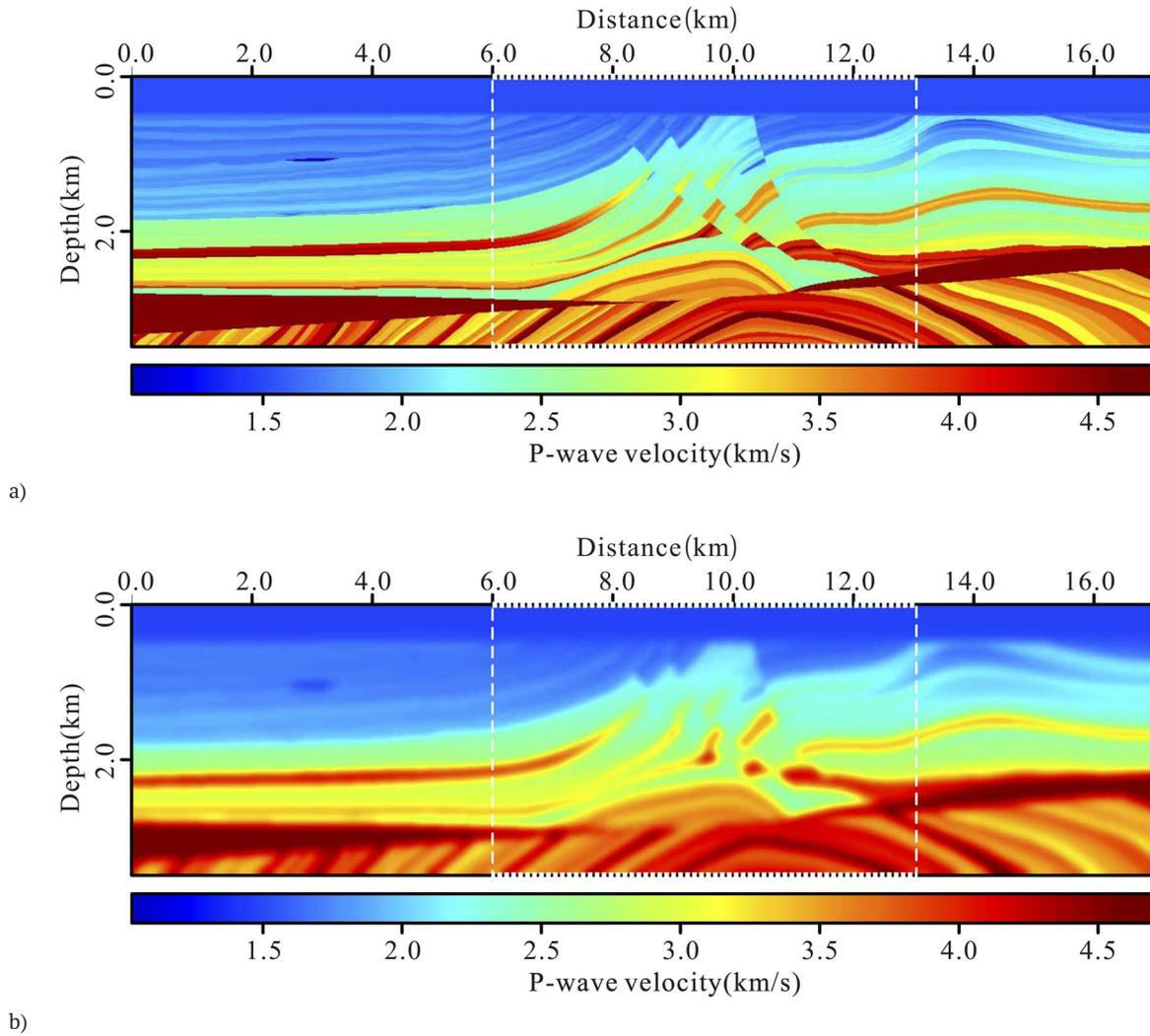
**Figure 10.** The resampled (a) and smoothed (b) Marmousi2 model corresponding to P-wave velocity for elastic wave simulation and reverse time migration, respectively. The subset denoted by the dashed rectangle is used for elastic wave simulation.
