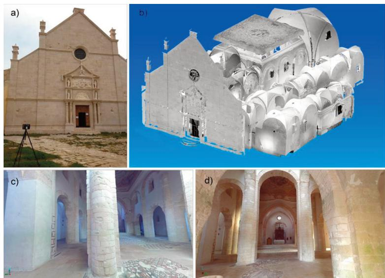
FIGURE 10. Laser scanner Focus 3D MS120 (FARO) (a), mesh visualization of the model (b), RGB visualization of the cloud points (c, d).
