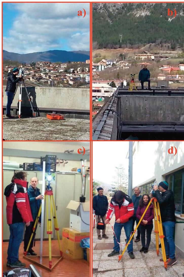
**Figure 5.** Images of the topographic survey: on the roof of the building, the total station (a) and the prism b) targeted from a); indoor the laboratory, the prism on tripod (c) targeted by the total station (d) located outside the laboratory.
